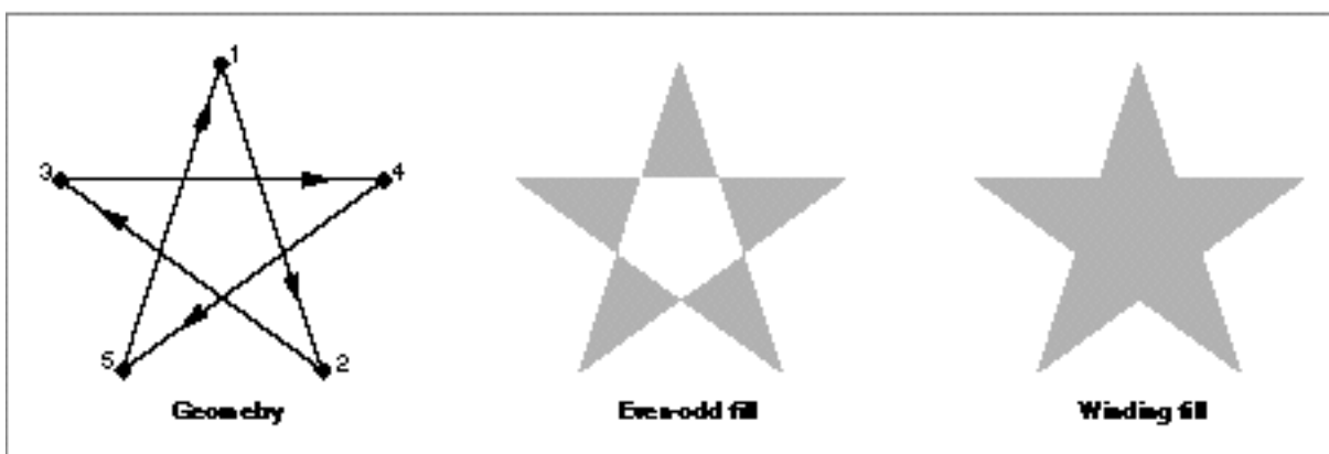
Figure 2-4 Even-odd and winding fills
