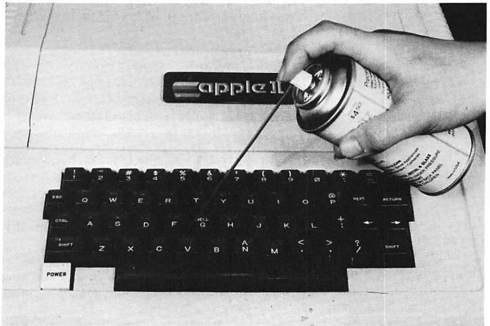
Fig. 1-4. Dusting with compressed air.
