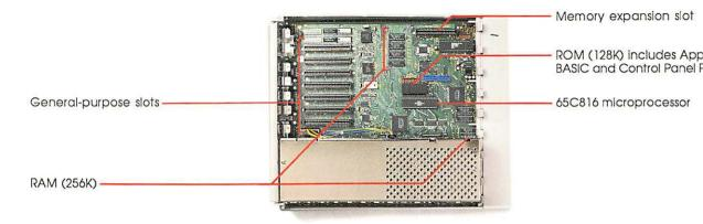
Figure D-1 Main circuit board
