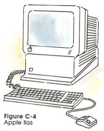
**Display** Columns: 80 or 40, selectable with Control Panel Program. Resolution: low (16 colors, 40 by 48); high (6 colors, 280 by 192); double-high (16 colors, 140 by 192); super-high (4 colors, 640 by 200; 16 colors, 320 by 200).
