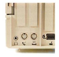
Figure 6-2 Serial ports
