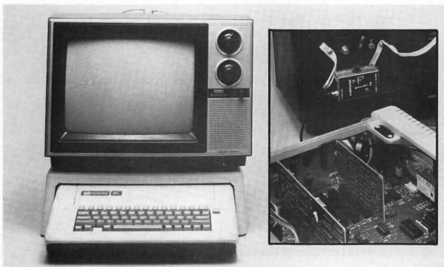
Figure 1-8. Attaching a television set
