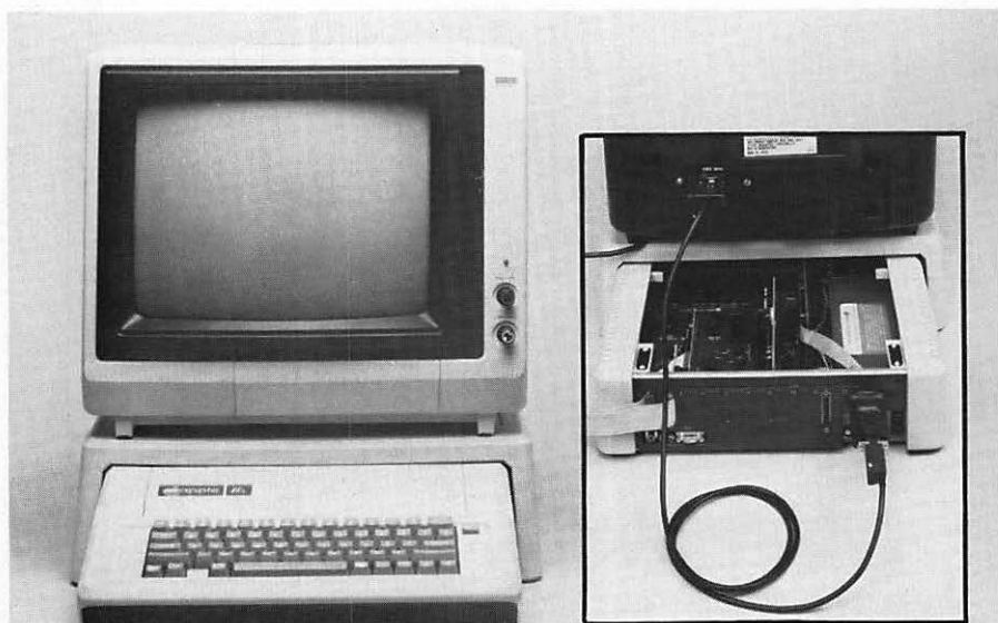
Figure 1-9. Attaching an RGB monitor
