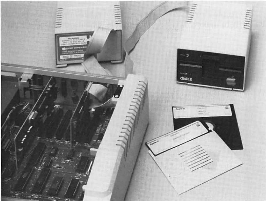
Figure 1-10. Disk II drives, controller cards, and disks
