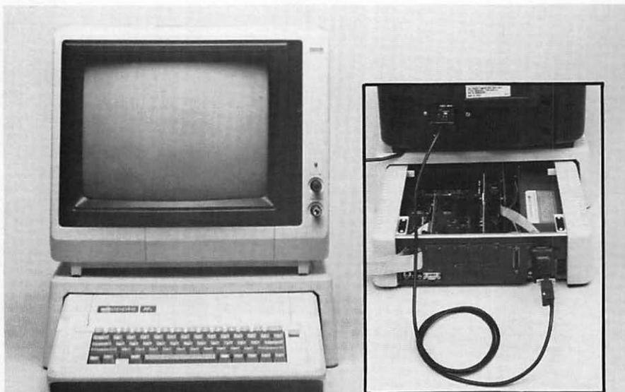
Figure 1-9. Attaching an RGB monitor
