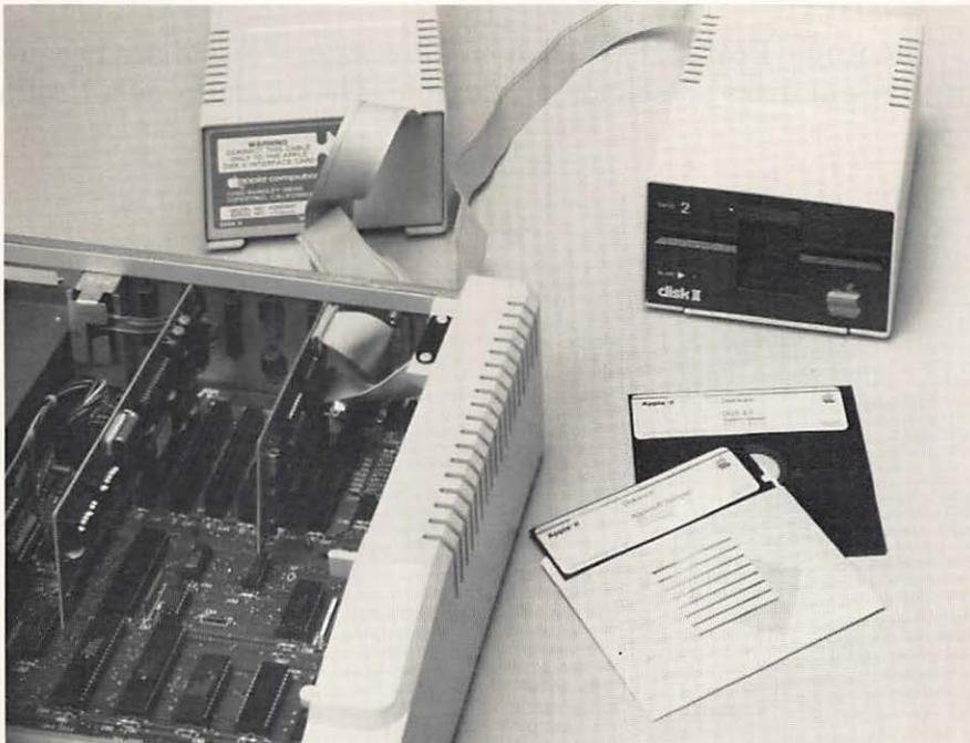
Figure 1-10. Disk II drives, controller cards, and disks
