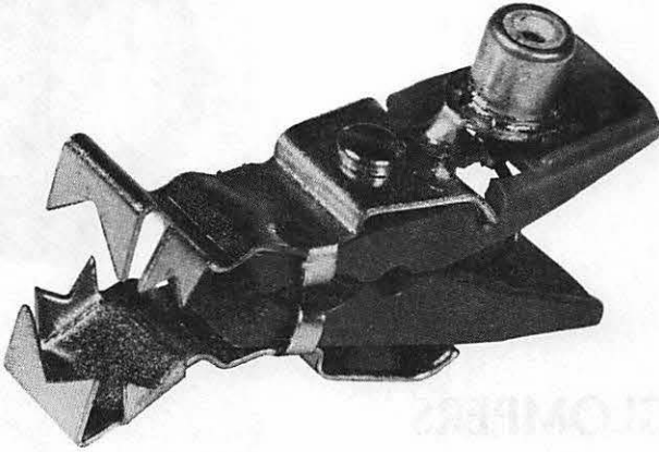
Glomper of the first kind is made from a phono jack and a clothespin connector. Use it if you often change or test different tv's.
