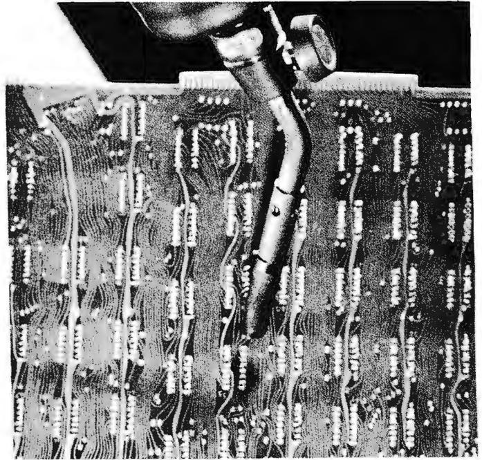
out separately results in bent, often broken leads. Devices are available which will heat all 14 or 16 pins of a small IC, but again a long time is needed to melt the solder since the total amount of energy available is limited to a small soldering pencil heating element. Most available boards are two sided and four layer boards aren't uncommon. Multi-layered boards make the required amount of energy even higher.
