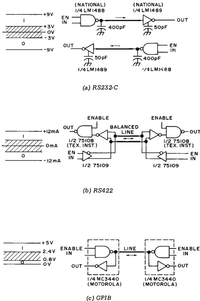
commercial modems, printers, test equipment, computers, and anywhere else you need a reasonable distance, noise free interface. Three of the most common include the RS232, the RS422, and the General Purpose Interface Buss or GPIB. Fig. 7 shows us what's involved in the way of signal levels and interface techniques.
