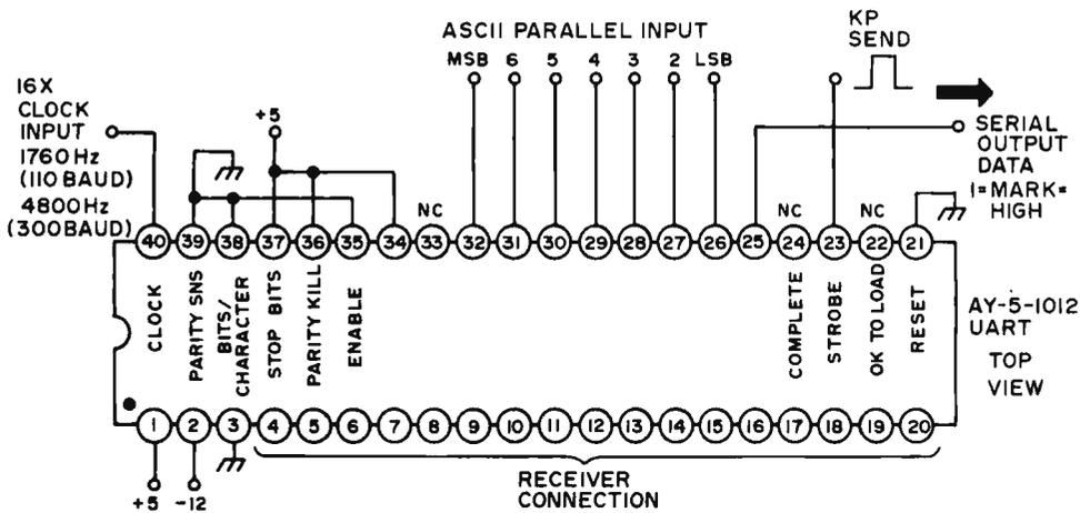
Baud circuit needs a clock of 1760 Hertz, while a 300 Baud one uses a 4800 Hertz clock and so on.
