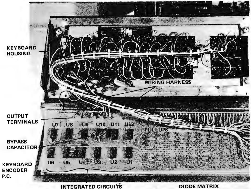
keyboard of the 1966-1970 vintage. This keyboard is a surplus Sanders Associates Model 722-1 subsystem, which comes enclosed in a metal housing with a fairly typical Teletype style key layout. On the right hand side of the keyboard is a set of special function keys, which obviously had some meaning in the original system using the device.
