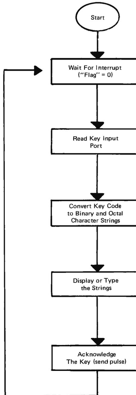
Fig. 6. Keyboard Test Program Flow Chart.
