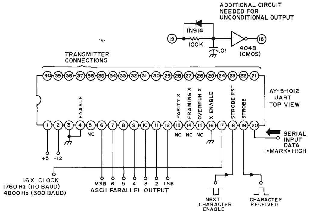
the receiver portion of the UART. Although the receiver and transmitter can be used in totally different circuits and at different baud rates, they have to operate with a common format, set by these pins.
