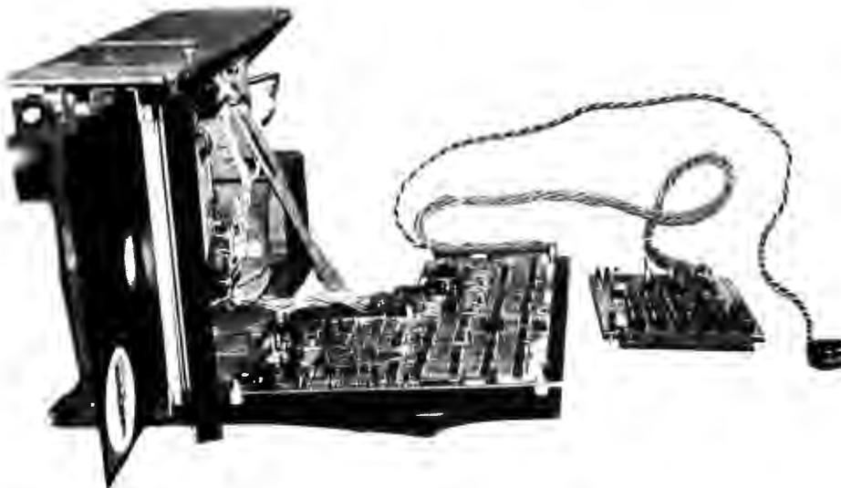
*Photo 1: The author's disk drive and interface board shown removed from the system. The Innovex drive is at left, with a diskette partially inserted in the front door and the electronics board for the drive shown in an "open" position. The interface board is at the end of a multiconductor twisted pair cable, and a separate cable is used for drive power.*
