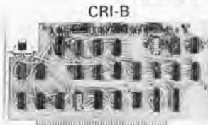
600 to 12,000 baud status controls, 1K monitor with cassette routines provided on tape.
