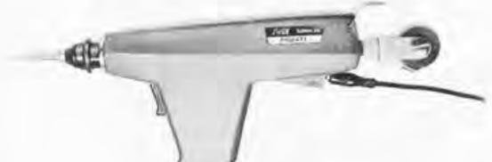
110 VAC powered wrapping tool. This \$80 tool will accept the P180 Slit-N-Wrap tool bit, or a standard wire wrapping attachment in the form of the P160-2A wrapping bit. While Slit-N-Wrap can be done by hand, it becomes much more convenient when it is powered as with this tool. (Because the Slit-N-Wrap technique requires no stripping of wire, it tends to be somewhat faster than standard wire wrap as a matter of course,
