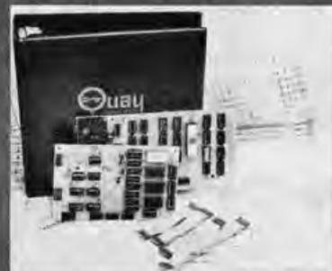
This dynamite new microcomputer system in a kit moves data like nothing else on the market. Run it alone or plug it into an S100 bus Altair/MSAI. For solo performance, all you need is an unregulated power supply and an I/O device. Plugged in, Quay 80AI is a CPU, ROM, SIO, and RAM board—run any S100 compatible device. BUT MORE THAN THAT. Quay 80AI's Z-80 CPU opens challenging new areas of personal computing.
