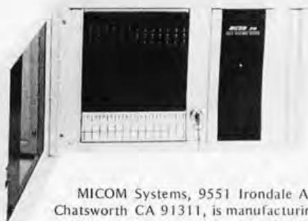
MICOM Systems, 9551 Irondale Av, Chatsworth CA 91311, is manufacturing a Voice Response System intended for minicomputers, which uses a micro-processor as a control element. The press release describes a system which can accept Touch-Tone encoded inputs and give digitally generated synthetic voice outputs. This system, which is definitely oriented toward commercial systems markets, has prices beginning at \$500. ■
