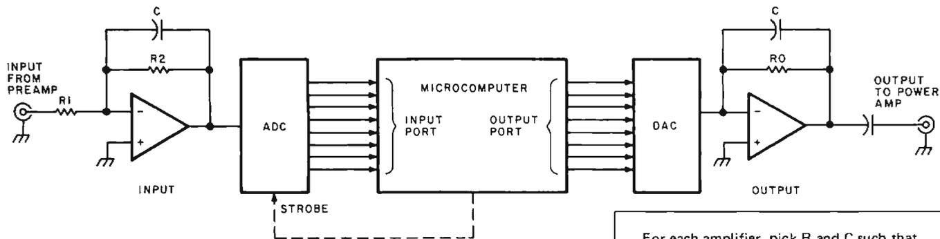
amplifier, needn't have as sharp a cutoff, but it should have the same cutoff frequency as the input filter. For the simple filters in figure 1, the cutoff frequency is equal to  $1/2\pi RC$ , where R and C are the values of the feedback resistor and capacitor, respectively.
