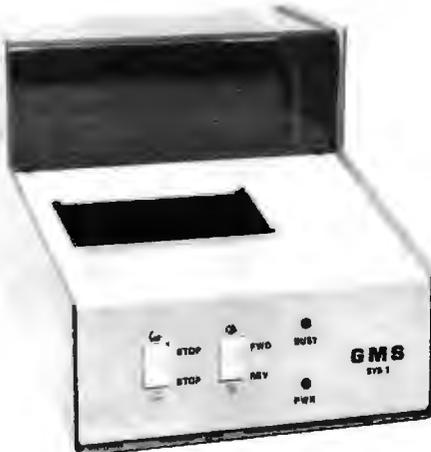
General Micro-Systems' new tape drive subsystem is a fast, inexpensive, high capacity mass storage device for microcomputers. The SYS 1 records biphasic Manchester code at 1600 bits per inch on ANSI specified data cassettes with a transfer rate of 2000 characters per second at ten inches per second.
