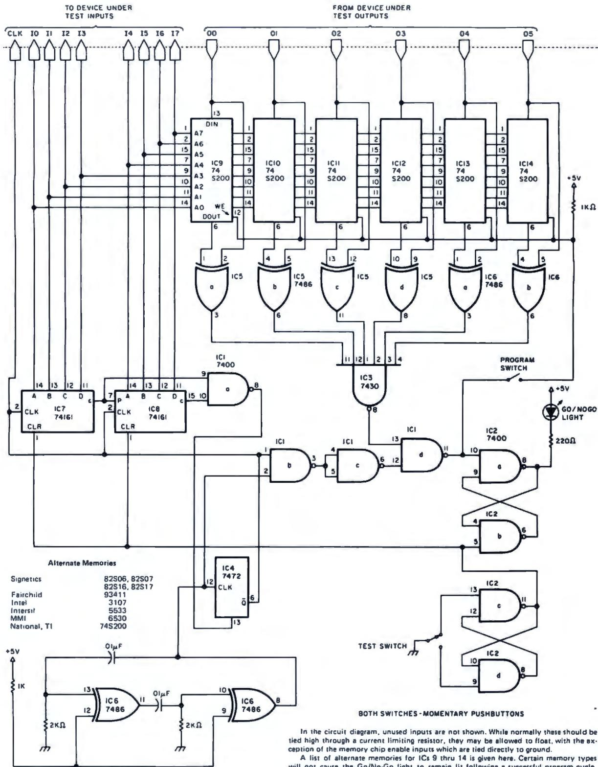
In the circuit diagram, unused inputs are not shown. While normally these should be tied high through a current limiting resistor, they may be allowed to float, with the exception of the memory chip enable inputs which are tied directly to ground.
