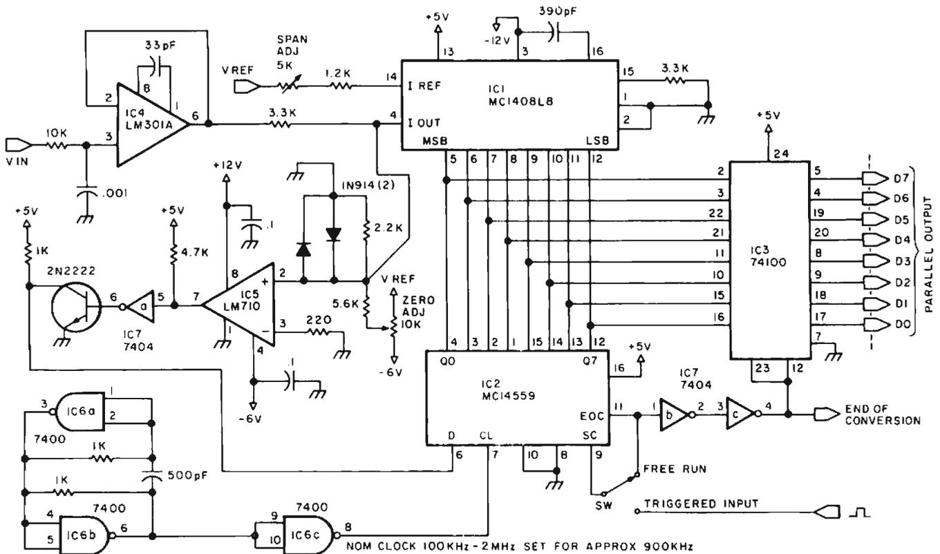
Figure 3a: An 8 bit successive approximation analog to digital converter.
