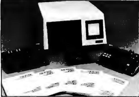
The AID-80F is a complete disk based computer from MOSTEK that provides for hardware and software development and debug. The heart of the AID-80F is the SDB-80 which combines the Z-80 processor with 16 K bytes of on board programmable memory. The
