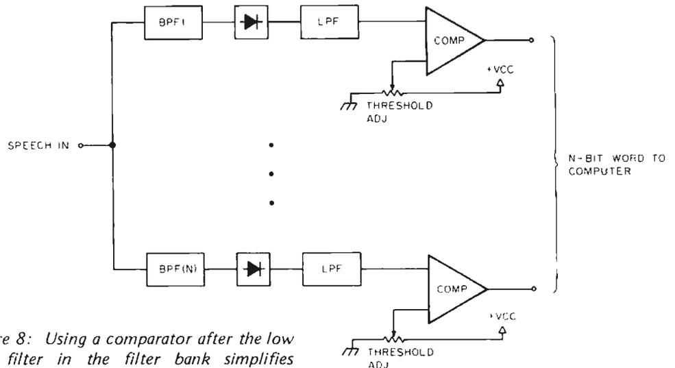
Figure 8: Using a comparator after the low pass filter in the filter bank simplifies hardware and reduces data rate at the cost of discarding useful information. The thresholds should be adjusted for the voice of each individual speaker. In addition, a good automatic gain control circuit should precede the filter bank to normalize the time domain signal.
