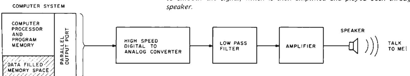
A digitized speech system creates its output waveform by digital to analog conversion rather than by completely analog generation as in the case of a voice synthesizer. The major consideration that limits the usefulness of digital speech is the vast quantity of data which must be stored to reproduce a single spoken word.
