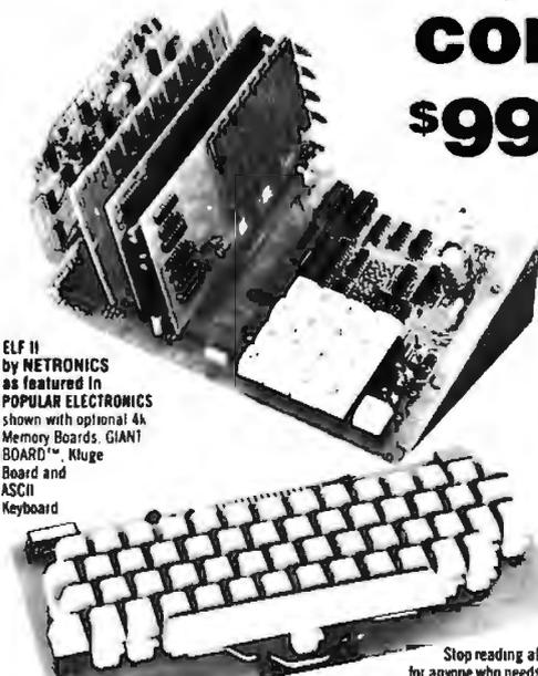
ELF II by NETRONICS as featured in POPULAR ELECTRONICS shown with optional 4k Memory Boards, GIANT BOARD™, Kluge Board and ASCII Keyboard
