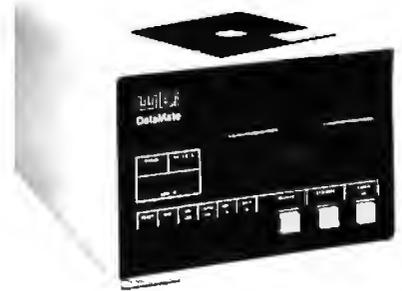
The DataMate minifloppy disk system is a data storage and editing unit for connection between any RS-232 asynchronous ASCII coded printer or display terminal and its modem. Features include 560 addressable records of up to 128 characters each, selective data transfer rates of up to 9600 bps, editing capabilities, search modes, and manual and remote controls. The price is \$1750 from Western Telematic Inc, 2435 S Anne St, Santa Ana CA 92704. ■
