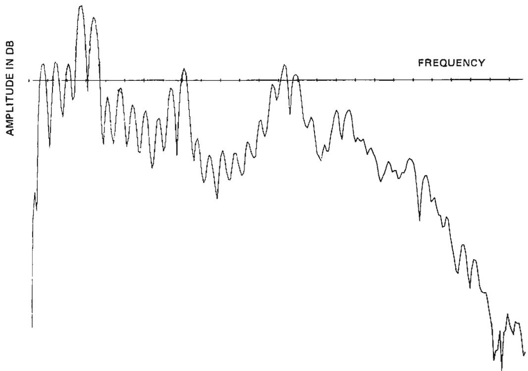
*Figure 5: The frequency (logarithmic magnitude) spectrum of a 25 ms segment of speech. It covers the frequencies from 0 to 3.2 kHz. The major peaks correspond to the formant frequencies while the smaller, regularly spaced peaks are harmonics of the glottal frequency. In this case it is obvious that the sound is voiced both from the harmonics of glottal frequency which are highly visible and from the fact that the lower frequencies have more energy than the higher ones.*
