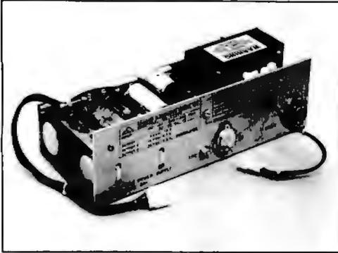
A power supply for floppy disk subsystems has been developed by Advanced Electronics Design Inc, POB 61779, Sunnyvale CA 94088. The AED 101 Triple Output supplies +5 VDC at 12 A, -12 VDC at 0.7 A, and +24 VDC at 3.5 A. It contains features such as switching regulation of +5 V, foldback limiting, current limiting and short circuit protection. The AED 101 is compact and is said to be available immediately. The cost is \$137.50 in large production quantities (\$.90 per watt). ■
