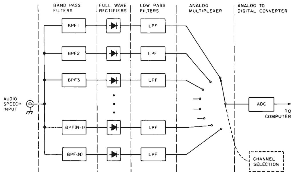
Figure 7: A filter bank feature extractor consists of a number of bandpass filters (BPF1 to BPF(N)) covering the range from about 100 to 10 kHz. The output of the filters is rectified and low pass filtered (LPF). Then it is multiplexed and digitized by the analog to digital converter for input into the computer.
