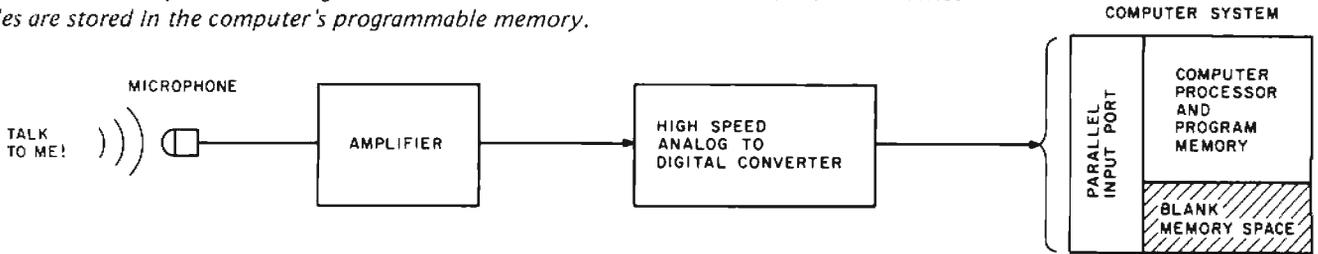
I needed it to troubleshoot this board. This is all you need for digitized speech." I tossed the board to Ken. "It contains a 100,000 sample per second 8 bit analog to digital converter and an equivalent speed digital to analog converter. And now the beauty part: It cost less than \$35 to build."
