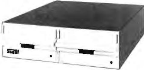
The Southwest Technical Products Corp DMAF1 is a dual drive, single density, double sided 8 inch floppy disk system. The hardware consists of an SS-50 bus (SwTPC 6800) compatible direct memory access (DMA) controller capable of handling up to four drives,
