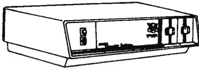
This sleek new mainframe is neatly trimmed to hold six S-100 boards, two mini-floppy drives, and is available in five colors. Power requirements: 115/220 VAC, 50 60 HZ, Weight: 27 lbs. (with drives). Dimensions: 21.375" Wide X 8.4" High X 15.875" Deep. Power Supply: 8 volts at 18 Amps unregulated. 16 volts at 3 amps unregulated. 16 volts at 3 amps unregulated. 5 volts at 3 amps regulated. 12 volts at 3 amps regulated.
