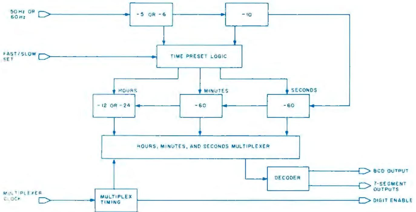
Figure 2: The block diagram for a typical clock chip.
