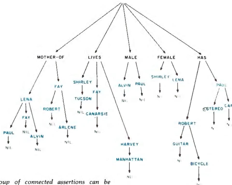
Figure 1: A group of connected assertions can be represented by a tree structure where the nodes of the tree represent locations within an assertion.
