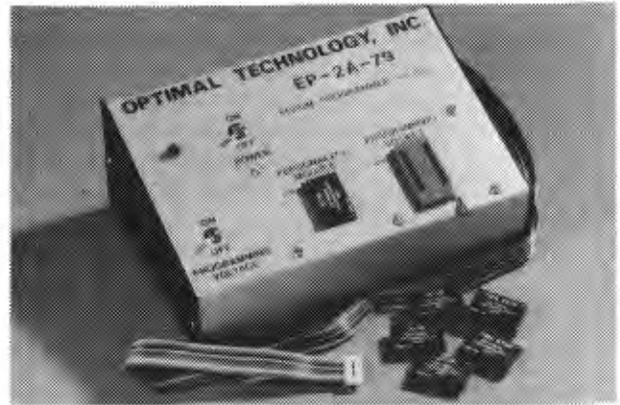
SOFTWARE AVAILABLE FOR F-8, 8080, 6800, 8085, Z-80, 6502, KIM-1, 1802, 2650. EPROM type is selected by a personality module which plugs into the front of the programmer. Power requirements are 115 VAC, 50/60 HZ at 15 watts. It is supplied with a 36 inch ribbon cable for connecting to microcomputer. Requires 1½ I/O ports. Priced at \$155 with one set of software. Personality modules are shown below.
