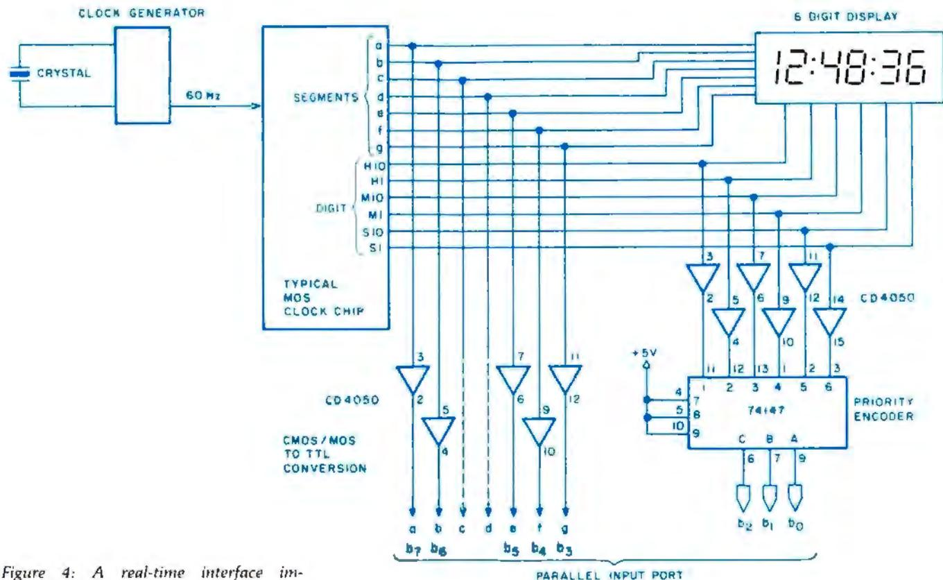
Figure 4: A real-time interface implemented using a typical clock chip.
