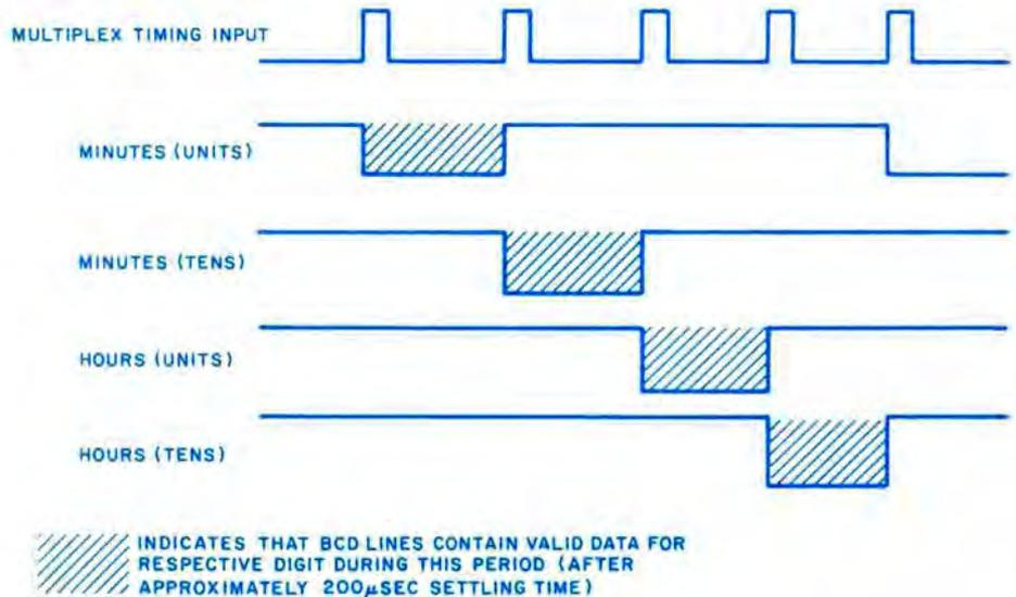
Figure 6: Display multiplex timing sequence for the circuit in figure 5.
