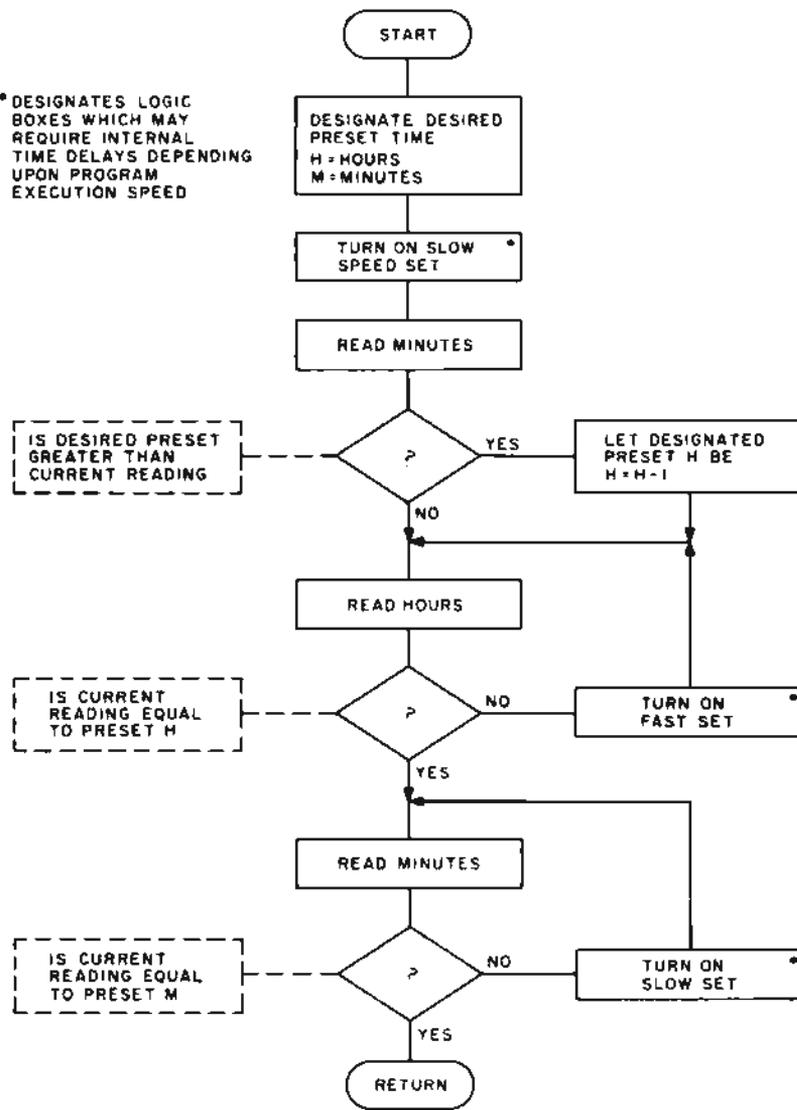
Figure 8: Flowchart for the automatic reset routine.
