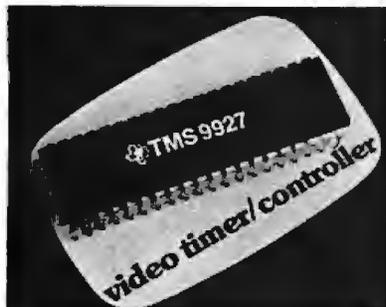
This single device video timer and controller has been announced by Texas Instruments Inc, POB 1443 M/S 6404, Houston TX 77001. A silicon gate, N-channel metal-oxide semiconductor (MOS) device, the TMS9927, offered in a 40 pin dual-in-line package, generates video display timing signals for standard and nonstandard video monitors that incorporate both interlaced and non-interlaced formats.
