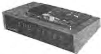
The EduCALC 189 GD is a 16-bit printed circuit board designed specifically for instruction. The instructor has an onboard 45-key alphanumeric keyboard and gets input, output and status information from the light-emitting diode display. Large characters on the other side of the unit repeat this display to the audience.
