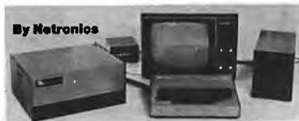
By Netronics registers...single step with register display at each break point...go to execution address. Level "A" in the Hex Version makes a perfect controller for industrial applications and can be programmed using the Netronics Hex Keypad/Display.
