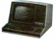
Two Z80 microprocessors, built-in mini-floppy drive, 25x80 display, upper and lower case, direct cursor addressing, 16K, expandable to 48K! DOS supports MICROSOFT BASIC and Assembly languages. Call for price!
