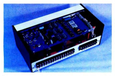
**Photo 5:** An internal view of the I/O controller containing relays, optoisolators, and analog interface components.
