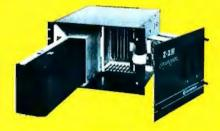
Hard disk drive at lower left can be interchanged just by stiding out and disconnecting plug. Seven free card stots are available. Z-2H includes printer interface card.
