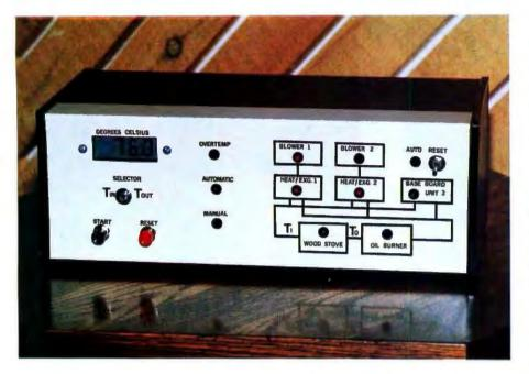
**Photo 4:** The computer I/O interface for the heating control system is attractively housed. It includes a display of either the input or output temperature of the Hydrostove and a real-time status display of the circulators and blowers.
