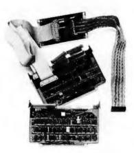
Motorola has announced six update packages to adapt a user's previous EXORciser I, IA, or II systems to MC6809 system design. These products enable designers to develop and debug any system centered around this power-
