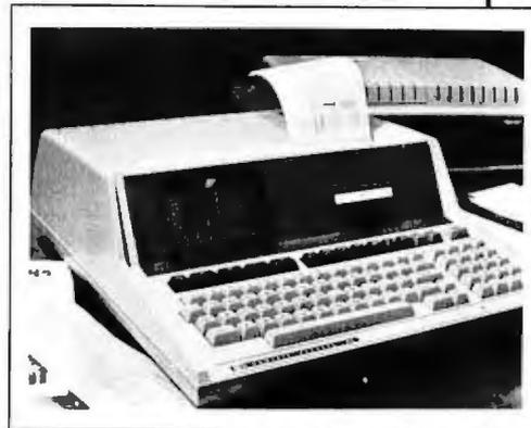
and graphics modes, prints two 32-character lines per second. The HP-85 tape drive uses HP Data Cartridges, which have a capacity of 200 K bytes, and feature a tape directory that enables the system to automatically find exact tape locations of recorded programs and data.
