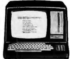
Z-89 Computer System: includes: Z19 Display, a built in 5 1/2" Floppy Disk, 2 serial ports, and 16K of memory. 2295.00 48K Memory version 2595.00
