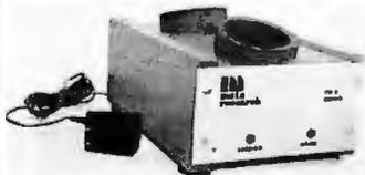
This acoustic modem uses a new type of crystal-lock circuitry. Even in kit form, no calibration or adjustments are required.
