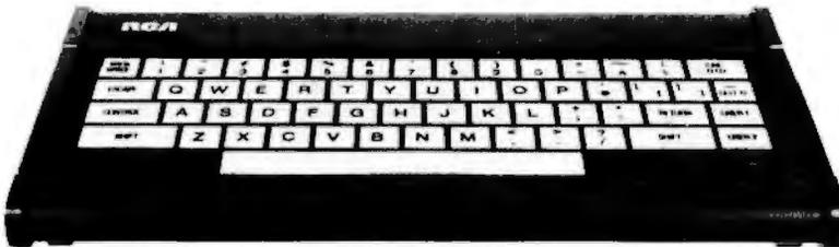
The RCA VP-601 keyboard has a 58 key typewriter format for alphanumeric entry. The VP-611 (\$15 additional\*) offers the same typewriter format plus an additional 16 key calculator type keypad.
