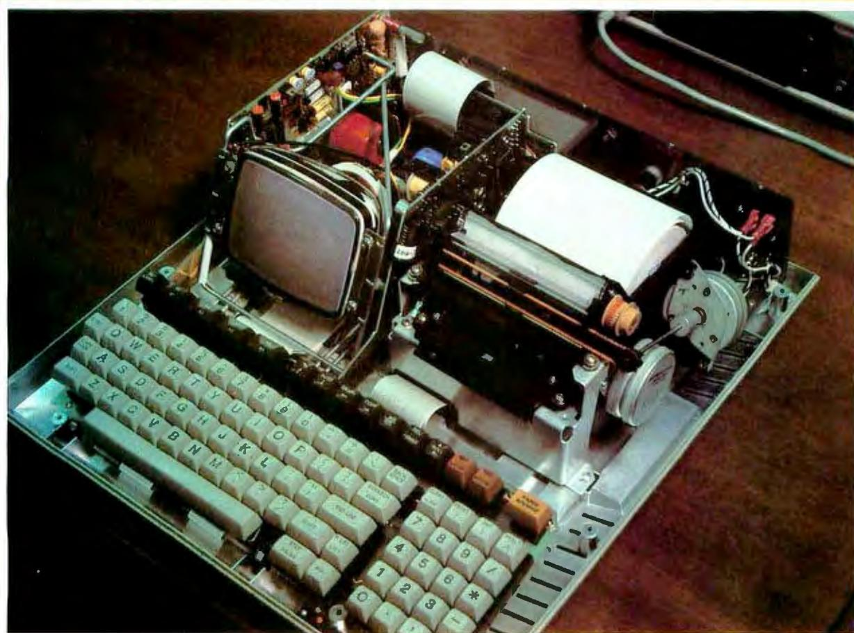
**Photo 2:** Inside the HP-85, showing the 5-inch video display cathode-ray tube, thermal printer, and data cartridge drive. The processor board is located under the keyboard (see photo 4). Note the set of user-definable keys at upper left of the keyboard. Labels for these keys are displayed at the bottom of the video screen.
