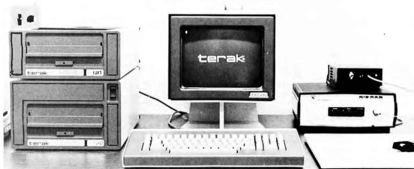
Photo 1: The Terak microcomputer with dual floppy-disk drive, video display, and keyboard. The Summagraphics Bit Pad consists of the digitizing tablet and the microcomputer control unit.
