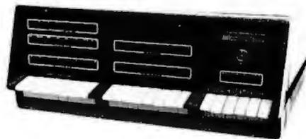
The new series II CPO Board features a 4 MHz Z-80A CPU and a full feature front panel. 20-slot actively terminated motherboard, with 25-amp power supply (50/60 HZ operation, incl. 68 cfm fan).
