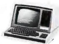
Two Z80 processors, mini-floppy drives, 25X80 display, 16K expandable to 48K!
