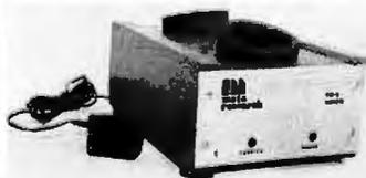
This acoustic modem uses a new type of crystal-lock circuitry. Even in kit form, no calibration or adjustments are required.
