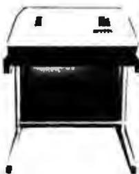
**300 Series Ballistic Printers.** This application-oriented matrix printer is built to last. Features include: Ballistic Printing • Positive 180 cps • Bi-directional Printing • A character buffer that is optionally expandable to 2,048 characters • 512 character buffer standard.
