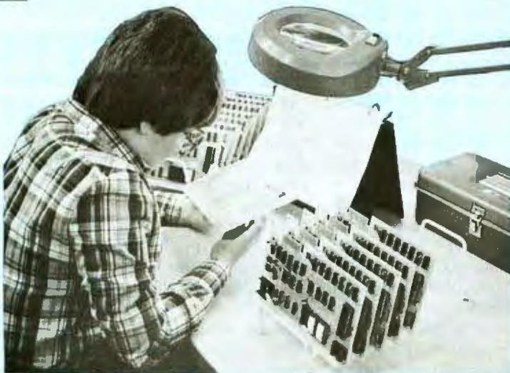
"Slipping a circuit board through the eye of a needle would be easier than slipping a cold solder joint past Beverly. These are four-drive LFD-400/800 disk system controllers she's inspecting."
