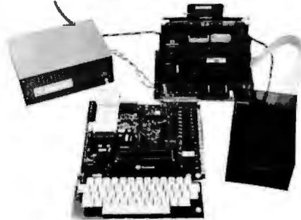
A complete disk system for the Rockwell Aim 65. Uses the Rockwell Expansion Motherboard. Base price of \$850 (U.S.) includes controller with software in Eprom, disk power supply and one packaged Shugart SA400 Drive.
