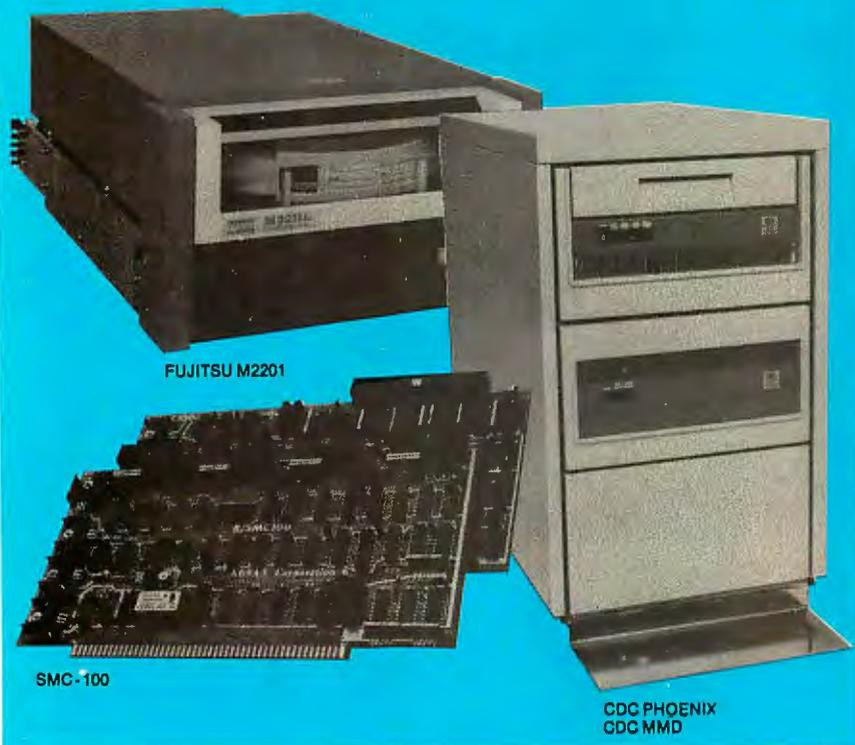
**Konan's SMC-100 is versatile, fast, cost efficient. It's the disk controller that brings S-100 bus micro computers together with large capacity hard disk drives.**
