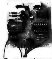
• Converts a low cost tape recorder to a digital recorder • Works up to 1200 baud • Digital in and out are TTL serial • Output of board connects to mic. in of recorder • Earphone of recorder connects to input on board • No coils • Requires +5 volts, low power drain • Board only \$7.60 Part No. 111, with parts \$29.95 Part No. 111A
