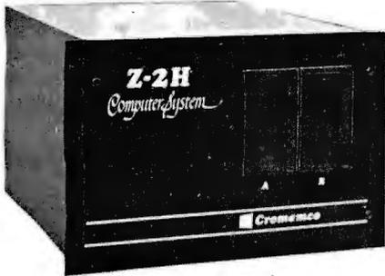
• Full 11-megabyte hard disk system • fast Z80A 4 MHz processor • two floppy disk drives • 64K RAM memory • RS232 special interface • printer interface • extensive software available
