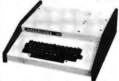
**The Challenger 4P.** A 4-slot computer with one open slot. Highly sophisticated 16 color video interface. 32 rows x 64 columns, upper and lower case. BK BASIC-in-ROM, BK RAM. 200-20KHz programmable tone generator. AC remote interface. Expandable to 32K RAM and two mini-floppy drives. **\$750.**
