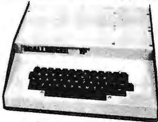
**The Challenger 1P.** The best bargain in personal computer anywhere! BK BASIC-in-ROM. 4K RAM. Cassette based with 53-key keyboard. B&W video interface, 30 rows x 30 columns. Upper and lower case. **\$399.**
