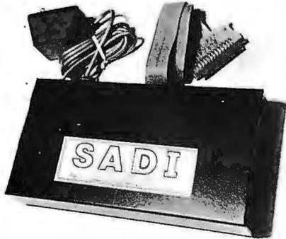
SADI - The microprocessor based serial and parallel interface for the Commodore PET. SADI allows you to connect your PET to parallel and serial printers, CRT's, modems, acoustic couplers, hard copy terminals and other computers. The serial and parallel ports are independent allowing the PET to communicate with both peripheral devices simultaneously or one at a time. In addition, the RS-232 device can communicate with the parallel device.
