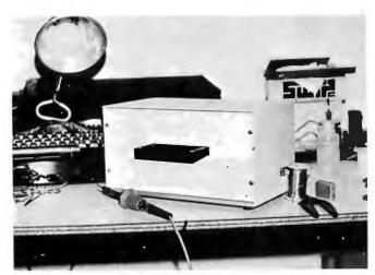
Photo 6: Taurus card reader. Cards are inserted through the slit above the black shelf on the front. Output is through the DB-25 connector on the side (partially obscured by roll of solder).
