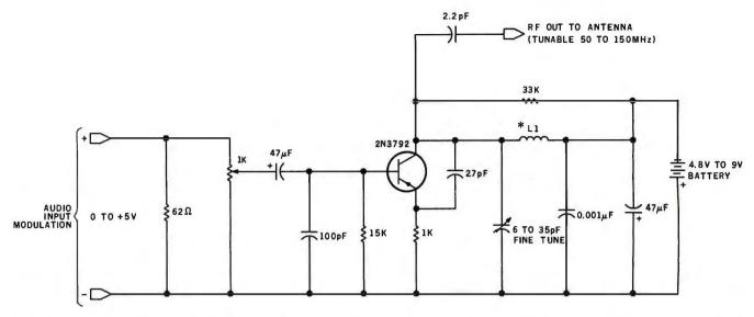
**Figure 5:** Schematic diagram of a VHF (very high frequency) transmitter, tunable 50 to 150 MHz, for use in the wireless remote-control system. This circuit is also suitable for use in wireless microphone systems. The coil L1 consists of eight turns of number-26 wire wrapped around a coil form with one-quarter-inch inside diameter.
