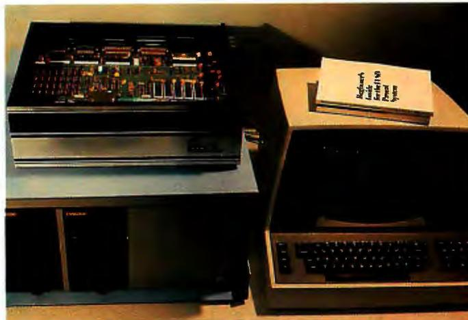
Figure 1: The Pascal Microengine is shown here in a system which includes two Shugart 8-inch disk drives in an Integrand cabinet and a Boroc IQ120 terminal. The computer uses a 16-bit processor chip and it executes p-code directly through the use of three integrated circuits on which the processor microinstructions are stored. The Microengine also includes 64 K bytes of memory, a 24-bit parallel port, and two RS-232C serial interfaces. The software provided is the UCSD extended Pascal system.
