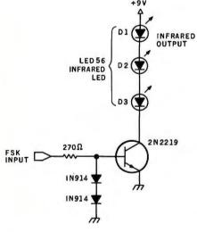
**Figure 6:** Schematic diagram of an infrared-light transmitter for use in the wireless control application, where use of the radio-frequency transmitter is impractical or undesirable. A series of LEDs emits bursts of infrared light that carry the control information to the phototransistor receiver illustrated in figure 9.
