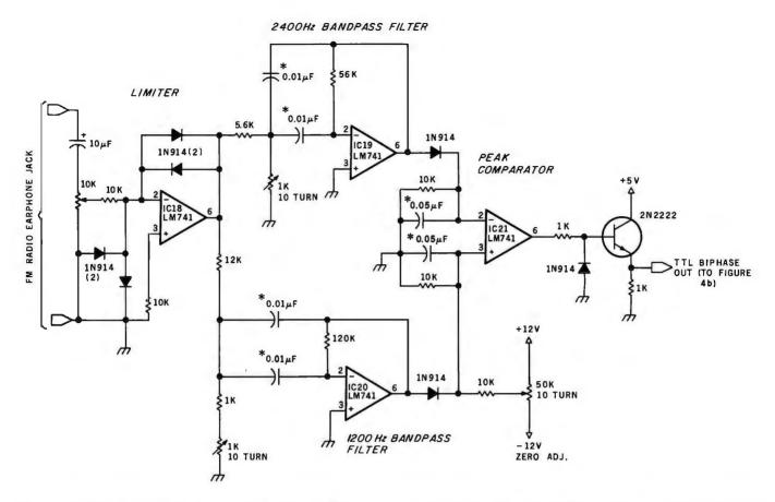
**Figure 4a:** Section of schematic diagram of the biphase FSK remote-control receiver. Here is the FSK demodulator, which connects to the audio output of an FM radio receiver and produces a TTL-level biphase output, which is further processed by the circuit in figure 4b. The capacitors marked with asterisks (\*) should be mylar or polycarbonate types.
