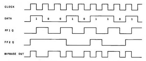
Figure 1b: Timing diagram of the biphase encoder of figure 1a. The clock and data pulses are combined into the biphase output.
