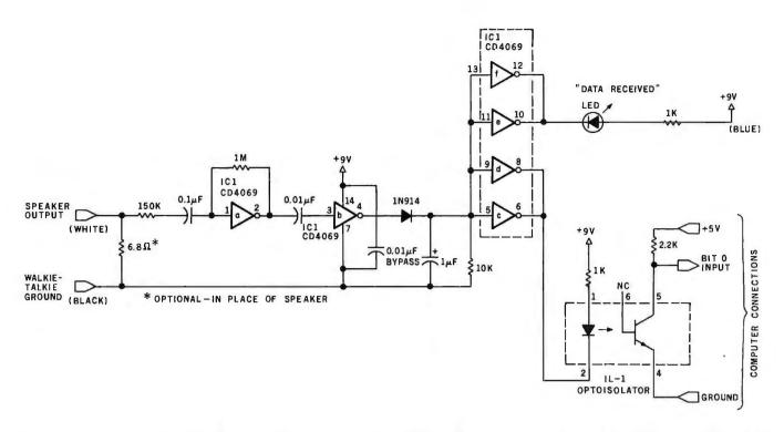
**Figure 10a:** A receiver circuit that allows use of inexpensive walkie-talkies for the transmission of control data. The two walkie-talkies used in this application were Radio Shack catalog number 60-4001 types, which have an integral Morse-code audio oscillator. One walkie-talkie is used as the handheld remote transmitter, the other as the receiver.
