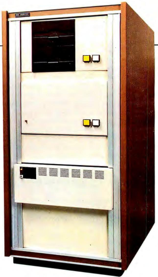
Series, the C3-B. Its specifications are the same as those of the C3-C. However, the C3-B offers a 74 Megabyte Winchester drive.
