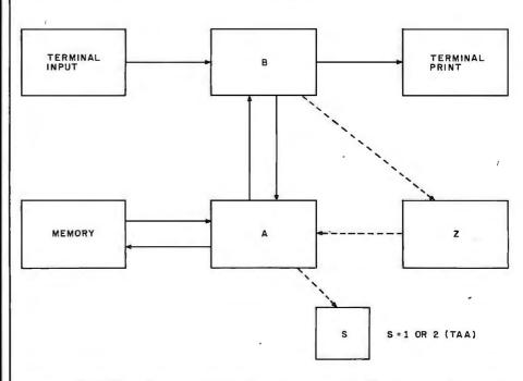
**Figure 1:** MICRO8 architecture. When the system is started, all registers and memory locations are cleared automatically. Arithmetic operations leave their results in register A. The exchange command (EXE) leaves the first value of B in Z. The maximum size of registers A and B is  $1 \times 10^{20}$ . The running time limit is five minutes, after which a dump command is performed. The limit on the number of machine cycles is 20,000.
