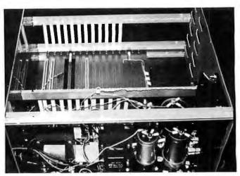
Photo 7: Side view of the system enclosure, showing the power supply and card cage.
