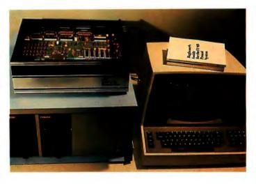
1: The Pascal Microengine is shown here in a system cludes two Shugart 8-inch disk drives in an Integrand cabinet Foroc IQ120 terminal. The computer uses a 16-bit processor and it executes p-code directly through the use of three integrated circuits on which the processor microinstruce stored. The Microengine also includes 64 K bytes of , a 24-bit parallel port, and two RS-232C serial interfaces. Itware provided is the UCSD extended Pascal system.
