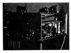
Photo 8: Front view of computer enclosure. The only switches are for power, run/stop, and system reset. The monitor in read-only memory handles other functions of a front panel.
