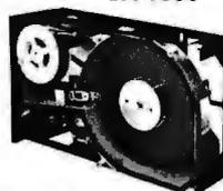
5 megs now expandable to 10, works alongside floppy disk drive for expanded storage. Use with controller below.
