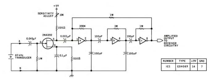
Figure 9b: Schematic diagram of a preamplifier circuit to be used with the ultrasonic remote-control receiver.
