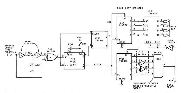
**Figure 4b:** Section of schematic diagram of the biphase FSK remote-control receiver; here is shown the biphase decoder and data discriminator, which decodes 4 bits of data and sends them to an input port on the computer. The period of the one-shot is set approximately equal to three-quarters of the transmitter clock period.
