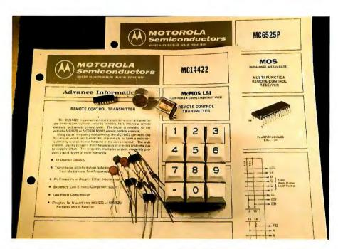
Photo 2: Assembled here are the parts needed to build a remote-control unit that uses the Motorola MC14422 CMOS LSI remote-control transmitter and MC6525 receiver.
