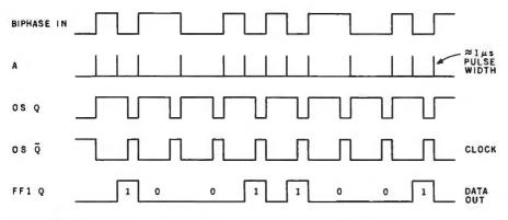
Figure 2b: Timing diagram of the biphase data decoder of figure 2a.
