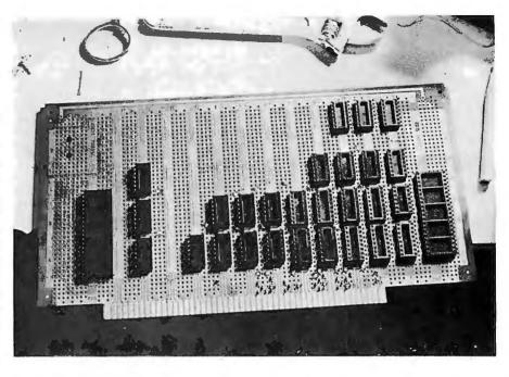
**Photo 3:** The parallel and serial I/O (input/output) board under construction. The sockets are attached with Eastman 910 adhesive.
