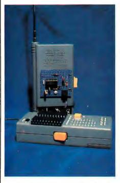
Photo 3: Two walkie-talkies can be used in a simple remote-control scheme. One walkie-talkie, used as the receiver, is modified by connection to the circuit illustrated in figure 10a. The new circuit is attached to the rear of the walkie-talkie's case, as shown. These walkie-talkies are sold by Radio Shack as catalog number 60-4001; they incorporate a Morse-code tone oscillator necessary to the control scheme. Transmission is on a frequency of 49.86 MHz.
