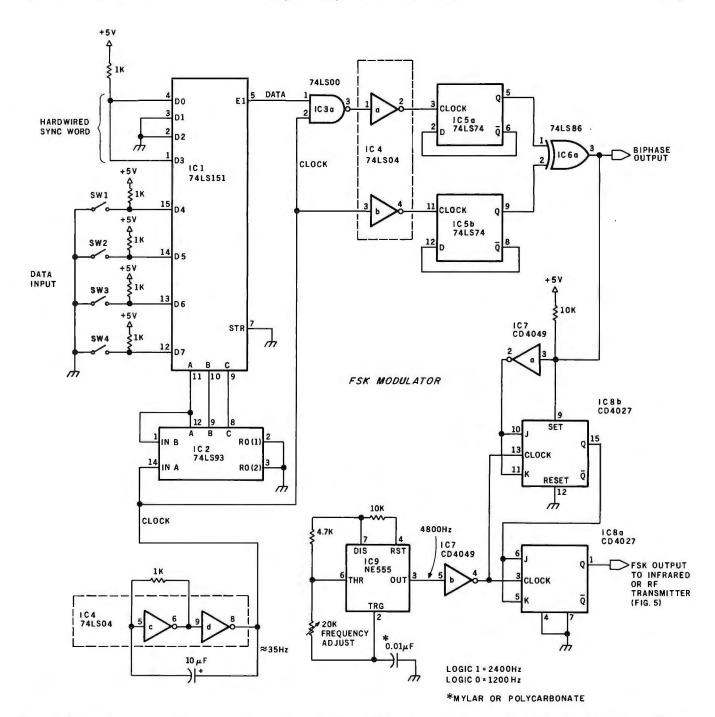
**Figure 3:** Schematic diagram of a functional sixteen-channel biphase FSK remote-control transmitter. This circuit, with the addition of an RF modulator, is packaged in the handheld unit illustrated in photo 1.
