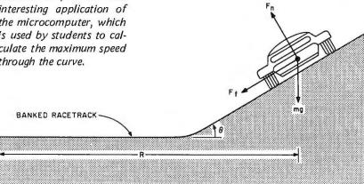
Consider the speedy sports car of figure 2 that is trying to round a banked curve with a radius of turn equal to R. A positively cambered, banked curve with angle of bank given by  $\theta$  is shown. Assume also that the curve is on a hill whose angle above the horizon is  $\beta$ , where  $\beta$  is positive if the car is going up the hill. Newton's equations of motion for the vertical (y) and horizontal (x) directions are:
