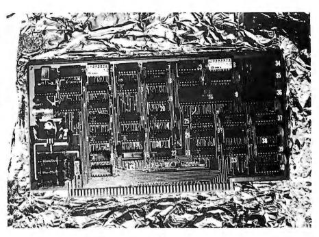
Photo 1: Ithaca Audio Z80 processor board for the S-100 bus.
