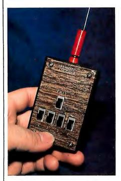
Photo 1: The handheld biphase FSK remote-control transmitter, which uses the circuit shown in figure 3. The transmit (XMIT) switch is a momentary power switch; the other four switches are used to set a 4-bit control-channel code.
