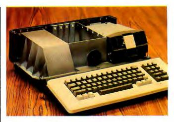
Photo 3: The Apple III with its plastic case removed to reveal the shielded aluminum chassis, designed for heat dissipation and RFI (radio-frequency interference) containment.
