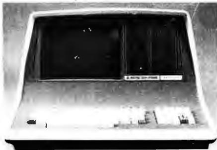
32K or 64K (Double or Quad Density units available). Uses two Z-80 CPU's. Commercial-type terminal with 12" monitor. Dual double density minifloppies. Over 350 kilobytes of storage (twice that with quad density drives). Two serial RS232 ports, I/O ports standard. Expandable with optional S-100 S-100 interface. Comes with CP/M<sup>™</sup> 2.2 operating system. MiniMicroMart includes BASIC interpreter and can supply a wide range of CP/M Development and Application software.
