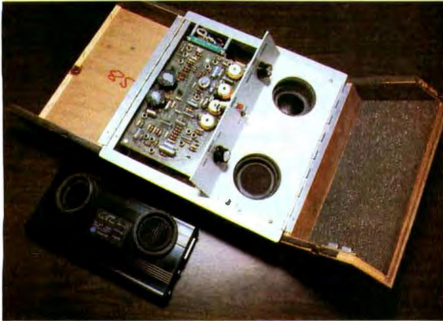
**Photo 2:** Comparison of two generations of modems. At right is an early model made by Anderson-Jacobson, shown with the covers open. The old modem uses discrete semiconductor components and toroidal inductors. On the left is an example of a current model of modem: a Novation Cat acoustic-coupled modem, which is popular with home-computer hobbyists.
