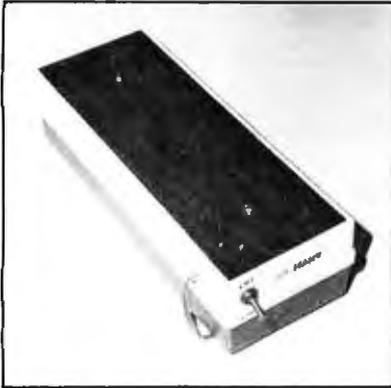
The QUV-T8 EPROM (erasable programmable read-only memory) eraser allows hobbyists to erase most industry standard ultraviolet EPROMs such as 2708, 2564, 2716, 2532, and 2704 series EPROMs. The device is capable of erasing up to twenty EPROMs at a time, with an erase time of approximately 25 minutes. The lamp has an estimated life of 7700 hours. It is available from Logical Devices Inc, 1525 N E 26th St, Ft Lauderdale FL 33305, (305) 566-6252.
