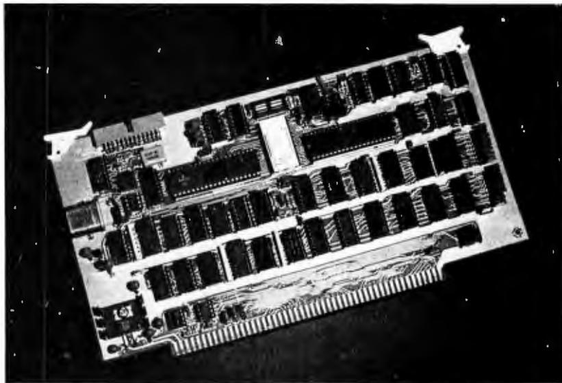
The 2810 Z80 single-board computer is designed for S-100 bus systems. It supports front panel operations and is fully compatible with the Altair and IMSAI computers. The board features easily selectable options including an RS-232 serial port that can be used for a console interface. Other options include I/O (input/output) address mirroring, a power-on jump to any location in memory, and wait states with optional wait state generation. Standard features for the 2810 include a 2 K-byte ROM
