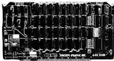
The Vector Graphic MP is a 5-by-7 dot-matrix, software-driven printer that can print at a speed of 150 cps (characters per second). The price of the MP is under \$1000 from Vector Graphic Inc, 31364 Via Colinas, Westlake Village CA 91361, (213) 991-2302. The Vector Graphic 64 K dynamic memory board is an 8-bit memory board which can be used with most Z80-based S-100 systems. The system offers bank selecting capability, allowing up to eight boards to be used in a system at the same time.
