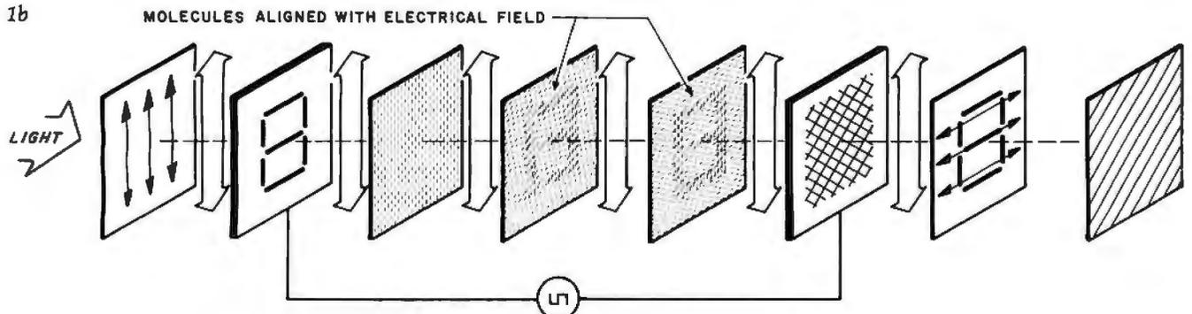
Figure 1: Block diagram of a field-effect liquid crystal. Field-effect liquid crystals are voltage-operated.
