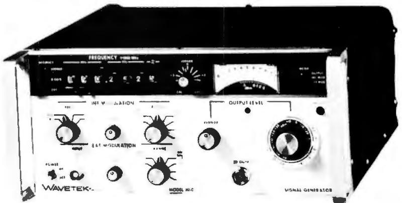
The Wavetek Model 3010 Signal Generator covers the entire frequency spectrum from 1 to 1000 MHz. It features 100 Hz resolution, 0.001% accuracy, complex modulation capabilities, and four internal modulation frequencies. Also featured are standard frequency programmability, Vernier controls for frequency and output level, and four FM (frequency modulation) and two AM (amplitude modulation) modulation scales. RF (radio frequency) power level is +13 to -137 dBm.
