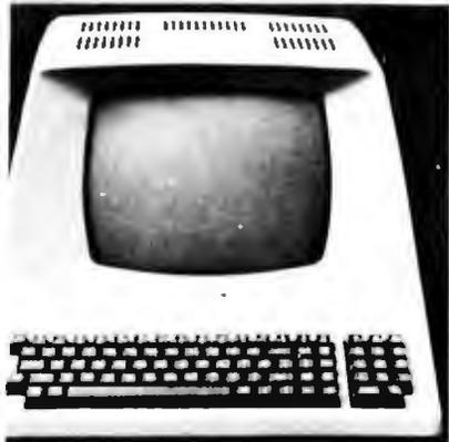
Upper and lower case, 15 baud rates: 75 to 1,000 baud, dual intensity, 24 x 80 character display, 12 x 10 resolution. Numeric pad. Programmable reversible video, auxiliary port, If-test mode, protect mode, block mode, scrolling, addressable cursor. Microprocessor controlled, programmable underline, line and character insert/delete. "C" version features typewriter-style keyboard. List \$950
