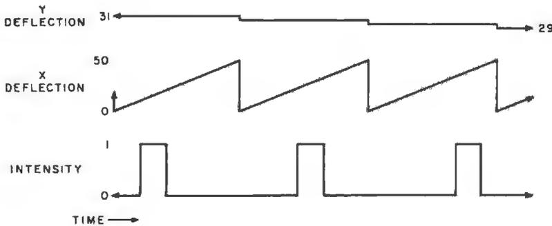
Figure 2: Example of plotting segment from (10,31) to (40,29) on a raster display. Since we have no control over the X and Y deflections, the intensity waveform is complicated. Also note the digitizing on the output display.
