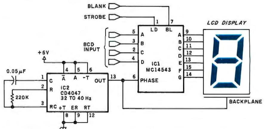
Figure 5: A single-digit, seven-segment LCD driver circuit.
