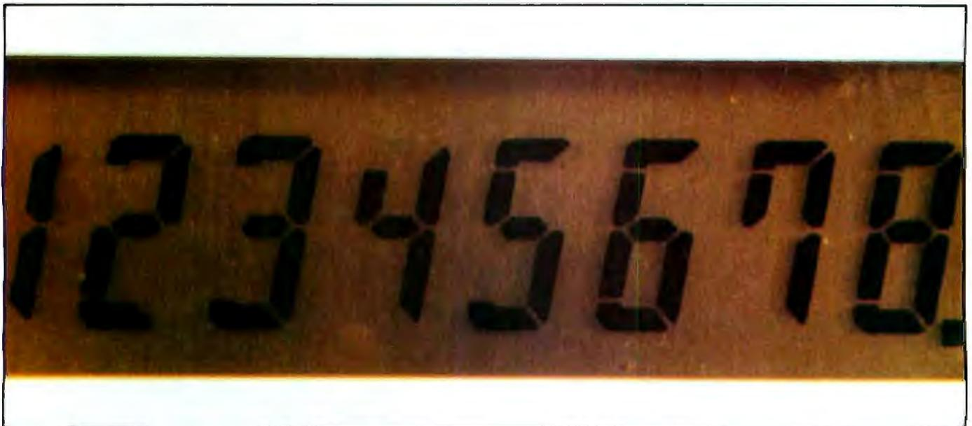
*Photo 8: Typical eight-digit, seven-segment LCD calculator display.*
