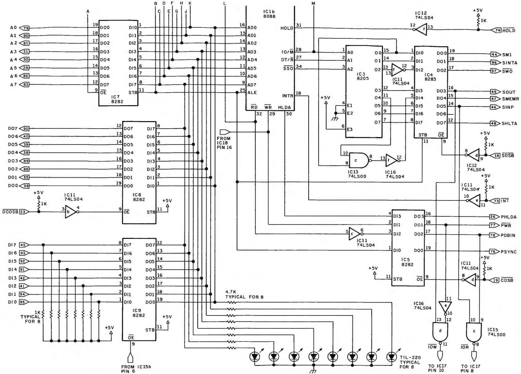
**Figure 1:** Schematic diagram of the 8088 processor board for the S-100 bus. This shows the logic necessary to provide a buffered, demultiplexed address bus, and input and output buses for the S-100 standard. Logic also produces
