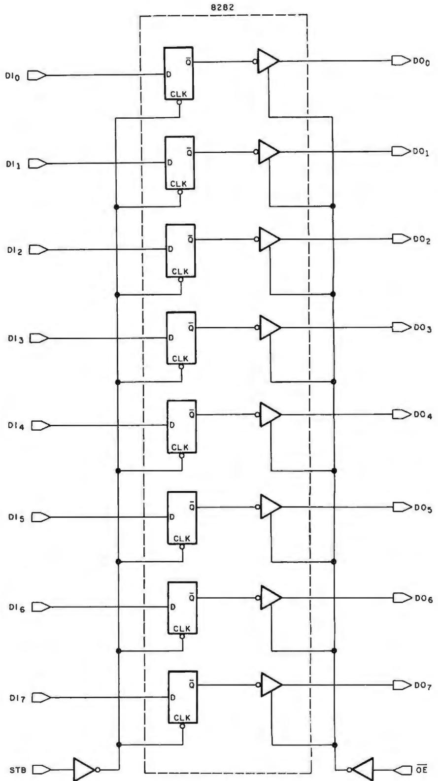
**Figure 2:** The 8282 8-bit buffer/latch. Similar to the familiar 8212, the 8282 has a greater drive capacity and comes in a narrower, twenty-pin dual-in-line package.
