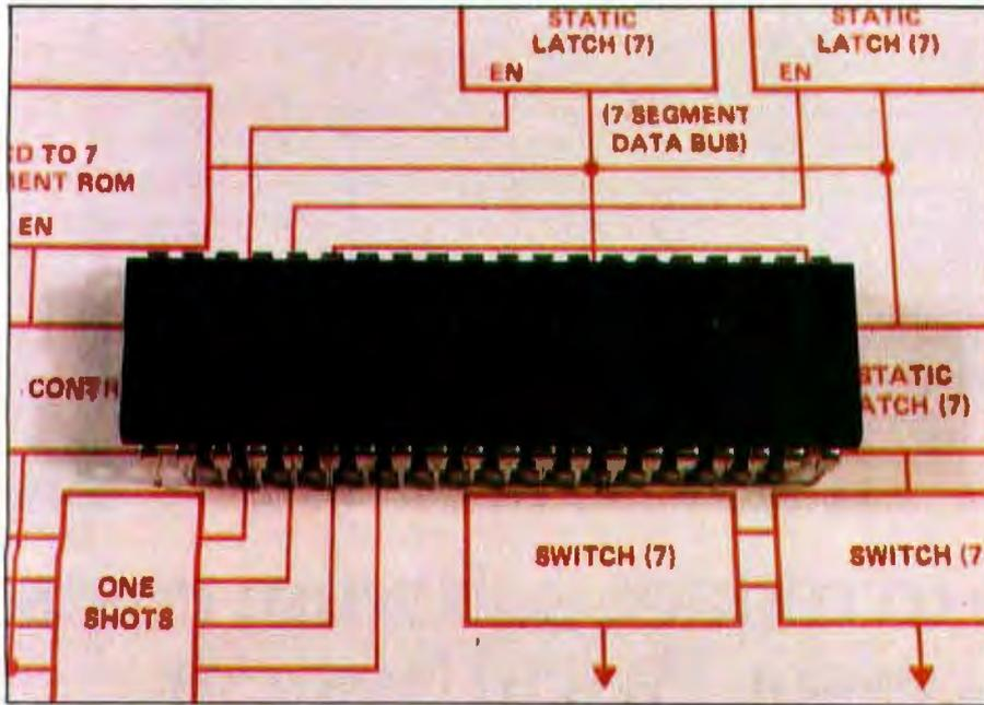
Photo 5: The Siliconix DF411 four-digit direct-drive LCD driver integrated circuit.
