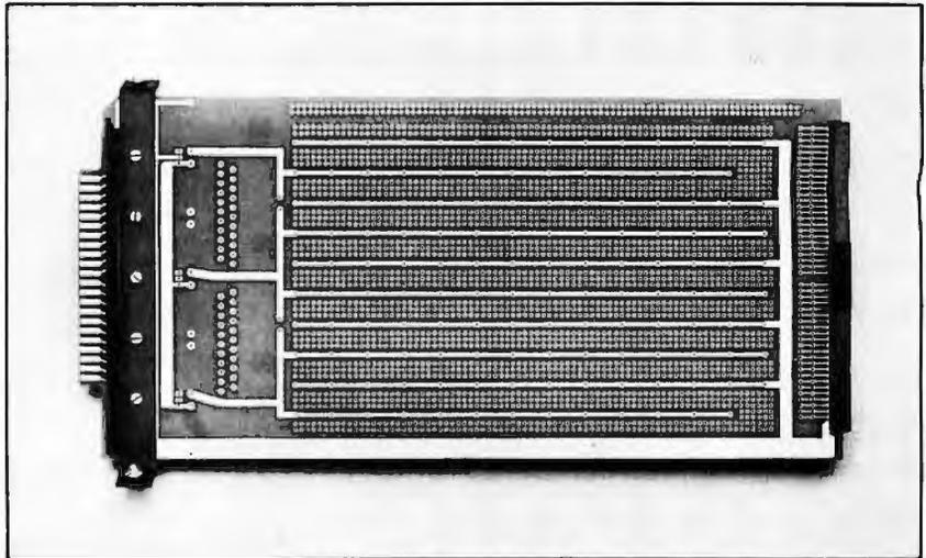
This prototype board will allow personal-computer users to build custom electronic interfaces for their Zenith/Heathkit H-8 personal computers. It is designed for use with a forty-four-pin edge-cable connector opposite the bus connector, or with many different Molex connectors from holes along the board top. There are locations
