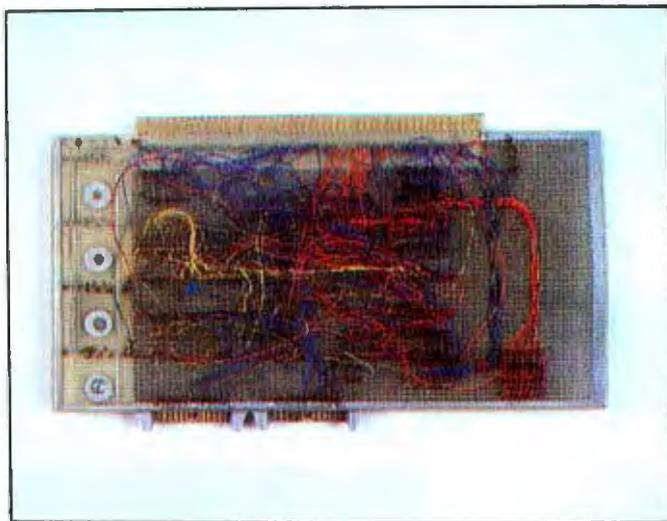
**Photo 1:** The processor board from front (photo 1a) and back (photo 1b). There is a large area left for design additions. Note that up-per pins on dual-in-line connectors are soldered to the ground plane for shielding. Multi-colored wiring makes debugging easier.
