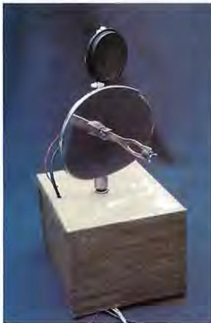
**Photo 1:** A computer-controlled, stepper-motor-driven infrared and ultrasonic ranging scanner. An infrared-sensitive photo Darlington transistor (GE L14F2) is mounted at the focus of a parabolic reflector, which is attached to the shaft of a stepper motor; the ultrasonic transducer is mounted above it.
