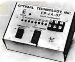
The Model EP-2A-87 EPROM Programmer has an RS-232 compatible interface and includes a 2K or 4K buffer. During the ON-LINE mode, another computer can download to the buffer. Only two easy-to-implement commands are available to an external computer. (Load buffer and read buffer.)
