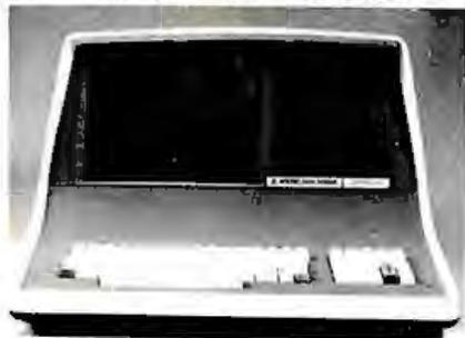
32K or 64K (Double or Quad Density units available). Uses two Z-80 CPU's. Commercial-type terminal with 12" monitor. Dual double density minifloppies. Over 350 kilobytes of storage (twice that with quad density drives). Two serial RS232 ports, I/O ports standard. Expandable with optional S-100 S-100 interface. Comes with CP/M™ 2.2 operating system. MiniMicroMart includes BASIC interpreter and can supply a wide range of CP/M Development and Application software.
