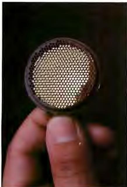
Photo 3: Close-up view of the Polaroid Ultrasonic Transducer.
