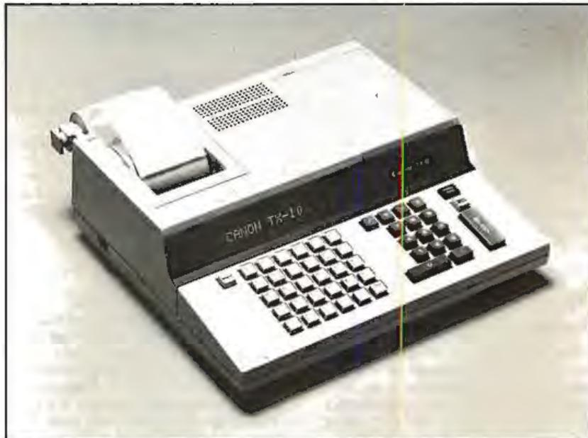
The TX Series microcomputers from Canon feature a 6809 microprocessor, extended BASIC and assembler language, a twenty-column alphanumeric video display, and a built-in twenty-six-column triple-copy impact printer. The models have 15 K bytes of user memory which can be expanded to 31 K bytes. Each model has an RS-232 interface port and a modem port. The TX-25 is a programmable machine with a full
