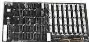
**CI-S100** — 16KB to 64KB. Transparent hidden refresh. No wait states at 4 Mhz. Compatible with Alpha Micro and all Major 8080, 8085 and Z80 Based S100 Systems. Expandable to 512K bytes thru Bank Selections. **64K x 8 \$750.00.**
