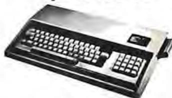
The SORCERER is a 280 CPU based micro-computer internally expandable to 48K, 4K ROM resident monitor, I/O connector for 5-100 expansion. Parallel and serial interface. Dual cassette I/O. Graphic resolution of 240 x 512, 30 lines of 64 characters, 8 x 8 dot matrix. Full ASCII set upper and lower case, plus standard graphic symbols. User may define up to 128 characters. Keyboard is 63-key data processing type, plus a 16 key numeric input pad.
