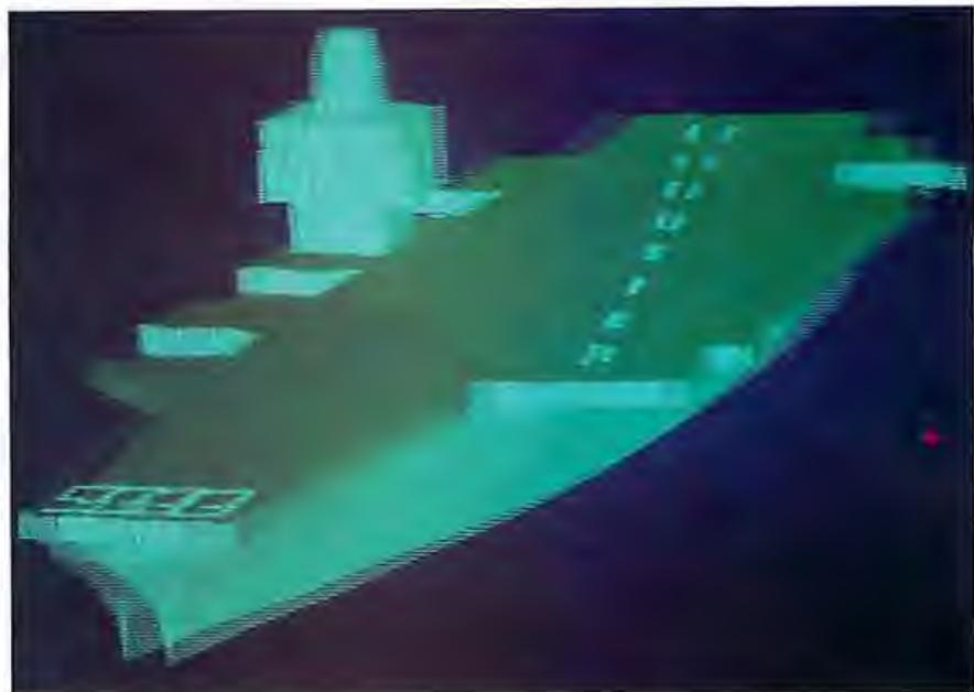
**Photo 10:** Interlaced left-eye and right-eye view of a computer-generated image of an aircraft carrier. The image is viewed in three dimensions when the user wears glasses with lenses made of PLZT (lead lanthanum zirconate titanate) ceramic. The lenses by the right and left are darkened alternately by voltage pulses synchronized to the display. Photo courtesy of John A. Roese and Larry E. McCleary, the Naval Ocean Systems Center.
