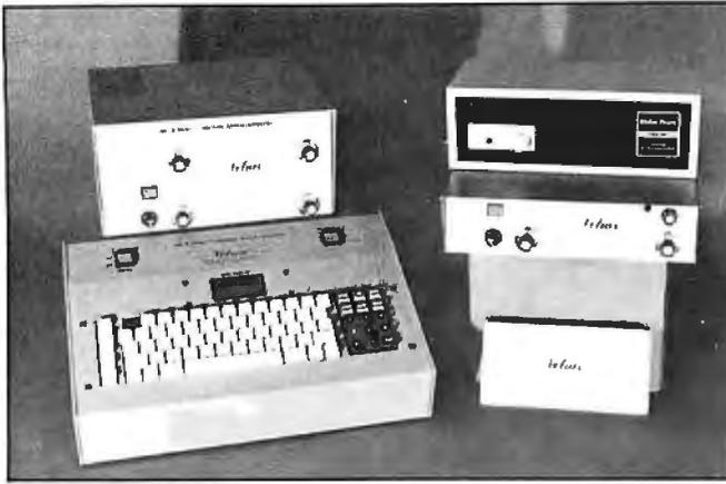
**Photo 1:** A selection of voice synthesizers. Top left: Votrax ML-1 multilingual synthesizer. Bottom left: phonetic keyboard for controlling a synthesizer without the use of a computer. Right top to bottom: Radio Shack TRS-80 Voice Synthesizer, Votrax VS6 synthesizer, Votrax VSK single-board voice synthesizer. Not shown: Votrax SC01 single-chip voice synthesizer.
