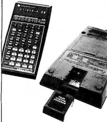
Stock market programs, oil field calculations, real estate software, and data for insurance rates are some of the many programs originally written for the TI 59/58 calculator and then converted to a custom Solid State Software™ module. Companies or individuals can permanently store up to 5000 program steps of their unique software in this nonerasable module.
