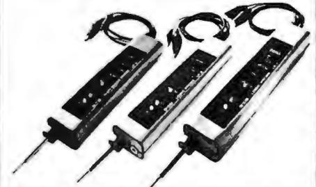
**LP-1 LOGIC PROBE**—Hand-held logic probe provides instant reading of logic levels for TTL, DTL, HTL or CMOS. Input Impedance: 100,000 Ohms. Min. Detectable Pulse: 50 ns. Max. Input Signal (Frequency): 10 MHz. Pulse Detector (LED): High speed train or single event. Pulse Memory: Pulse or level transition detected and stored. **GSLCP1 LIST PRICE \$50.00 SALE \$45.00**
