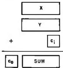
Figure 1: A pictorial model of the addition of  $X$ ,  $Y$ , and  $c_i$  to give  $SUM$  and the carry bit  $c_o$ .
