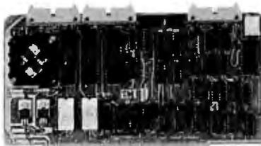
ECT's R<sup>2</sup>I/O is an S-100 Bus I/O Board with 3 Serial I/O Ports (UART's), 1 Parallel I/O Port, 4 Status Ports, 2K of ROM with the 8080 Apple Monitor Program and 2K of Static RAM.
