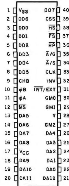
**Figure 5: Pin description of Motorola's MC6847 Video Display Generator.** In concert with the Synchronous Address Multiplexer (see figure 6), this device interprets the contents of a block of memory to create a color display (using either an internal character generator or an external one). The output signal is converted to composite video by an MC1372, while a device built of discrete components modulates the signal to radio frequencies for reception on a standard television.
