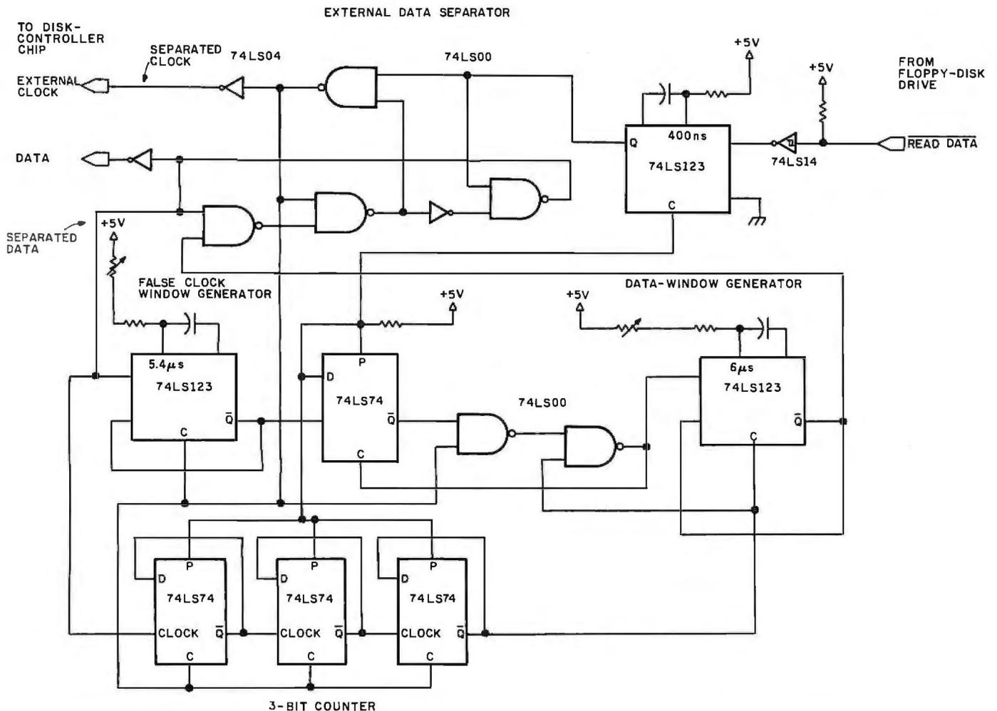
**Figure 5:** Simplified schematic diagram of a 5-inch floppy-disk external data separator. The internal data separator of the FD1771 is not recommended for use in such applications. This circuit can be added to any existing TRS-80 Expansion Interface (which does not have an external data separator) to improve performance.
