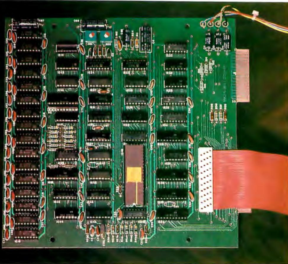
**Photo 2:** The Disk-80 printed-circuit board (circuit of figure 2). The red cable connects to the expansion connector on the TRS-80 keyboard/processor module. The 34-pin edge connector above the red cable is a 5-inch floppy-disk drive interface connector. The sixteen integrated circuits lined against the left side of the board are 32 K bytes' worth of type-4116 16 K-bit dynamic memory devices.
