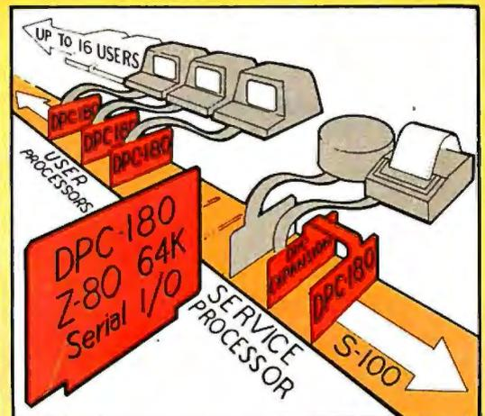
The ACE **DISCOVERY MULTIPROCESSOR** dedicates a complete, 64K Z-80 Distributed Processing single board Computer, the **dpc-180™** to each user. An expanded DPC coordinates all of the system activities.
