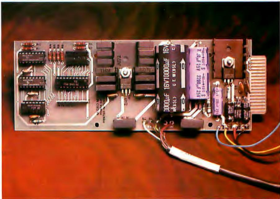
**Photo 3:** The Disk-80 power supply with the parallel printer interface. The power supply provides 1 A at +5 V, 400 mA at +12 V, and 50 mA at -5 V, and is designed for use with dynamic memories such as the 4116 that require sequenced application of power.
