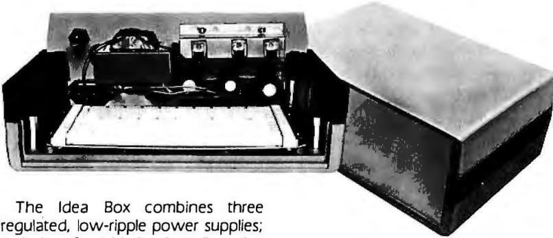
The Idea Box combines three regulated, low-ripple power supplies; a choice of a solderless breadboard, a pre-etched, pre-drilled printed-circuit board, or a blank foil board. This combination allows easy construction of a prototype or a built-once-only device. The Idea Box is priced from \$149.95. The circuit cards and printed-circuit
