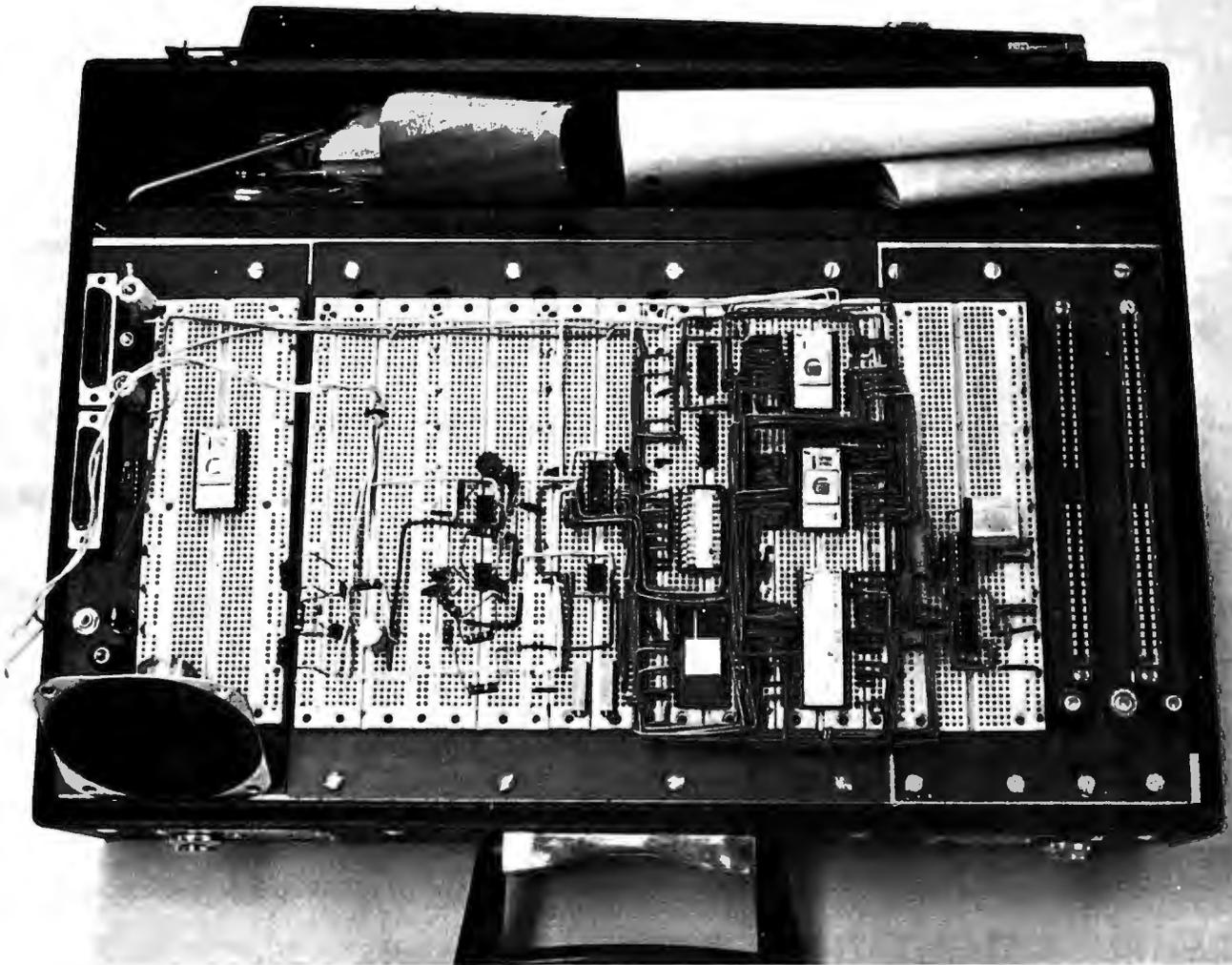
**Photo 1:** The author's microprocessor computer music system implemented in a breadboard prototype suitcase. A 2½-inch speaker (lower left) provides audio output for demonstrations. Best results were obtained by patching into the power amplifier of a high-fidelity receiver.
