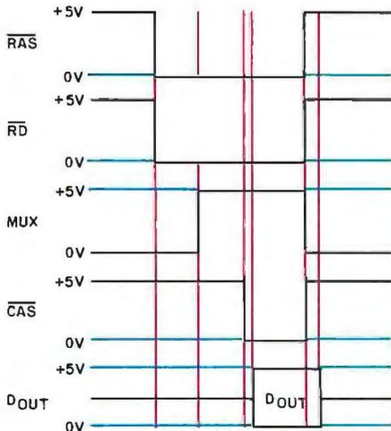
**Figure 3:**  $\overline{\text{RAS}}$ ,  $\overline{\text{CAS}}$ , and MUX timing diagram for 4116-type 16-pin dynamic-memory integrated circuit. A 14-bit address (16,384 by 1) is multiplexed into seven address pins. When MUX and  $\overline{\text{RAS}}$  are low, the row-address bits are read into the 4116. Later, when MUX is high and  $\overline{\text{CAS}}$  goes low, the column bits are read into the 4116, activating the data output for that memory cell.
