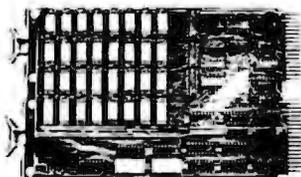
**CI-8080** — 16KB to 64KB on a single board. Plugs directly into MDS 800 and SBC 80/10. Addressable in 4K increments up to 64K. **16KB \$390.00. 64KB \$750.00.**
