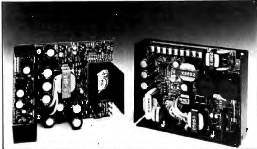
Sierracin/Power Systems has developed a series of 40 and 60 W open-frame switching DC power supplies. The 5A and 5B series, 40 and 60 W respectively, come in single and multiple-output versions. The single-output models 5A5 and 5B5 deliver 5 V at 7 A and 12 A at full load. Prices for these models are \$45 and \$75 respectively. The 40 W multiple-output 5AXMP delivers 5 V at
