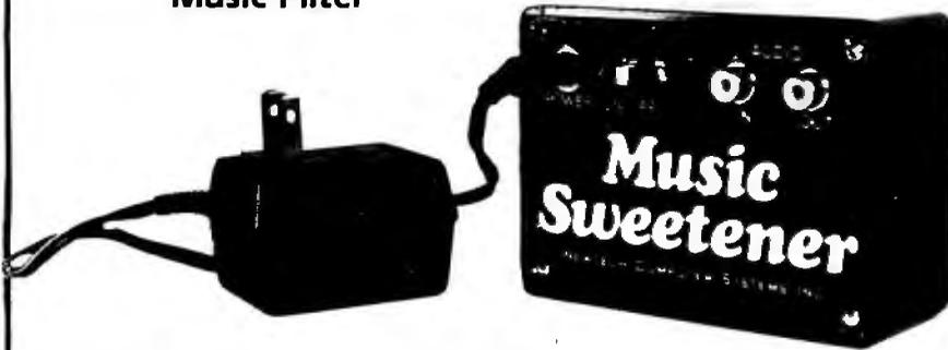
The Music Sweetener is a low-pass filter designed to enhance Software Affair's Orchestra-80 and other commercial and homebrew D/A (digital-to-analog) converter music synthesizers that do not already have a filter. The unit attenuates the unwanted high-frequency sampling noise better than a stereo system's treble tone
