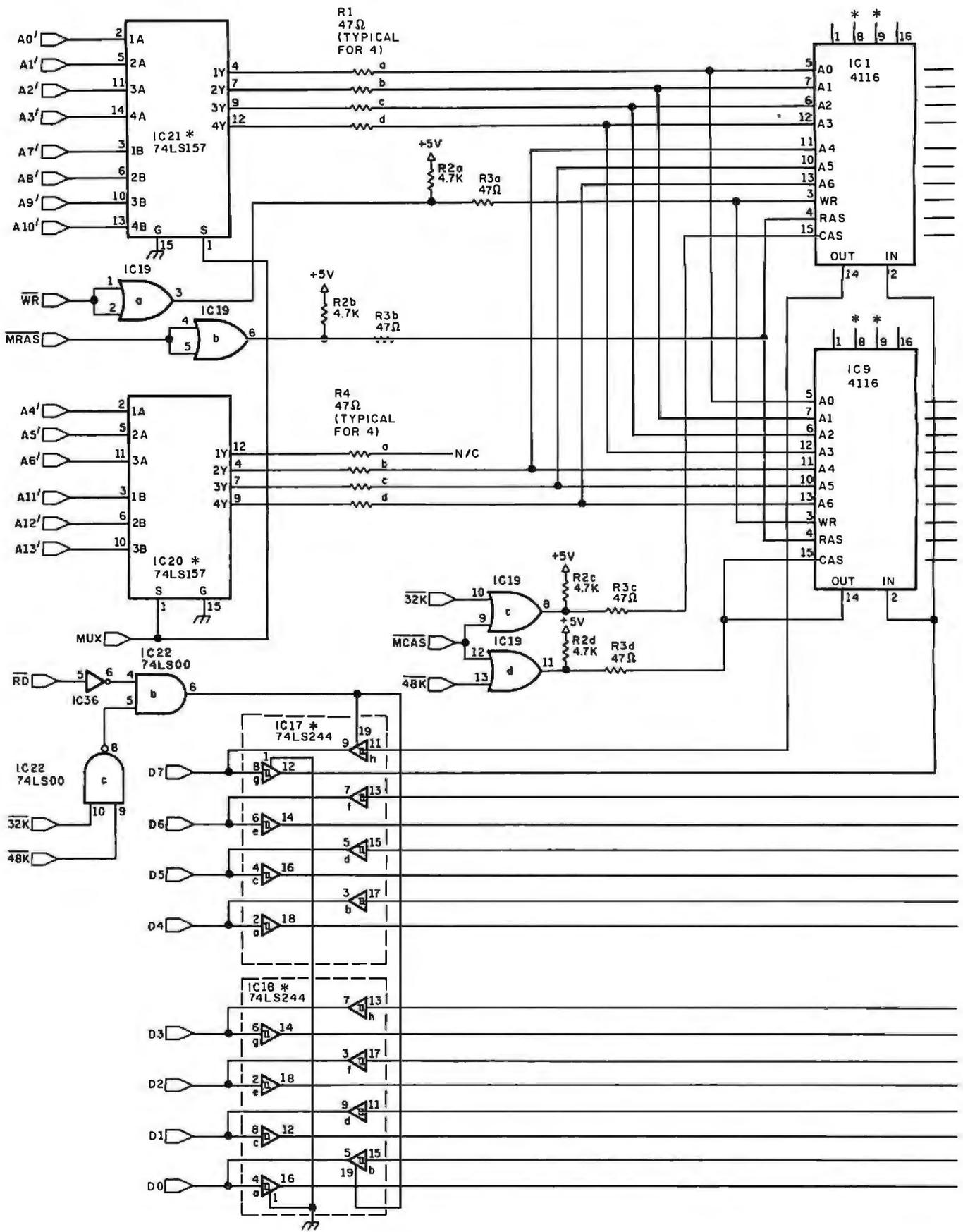
Figure 2b: The memory-expansion section of the Disk-80 module. See notes on page 44.
