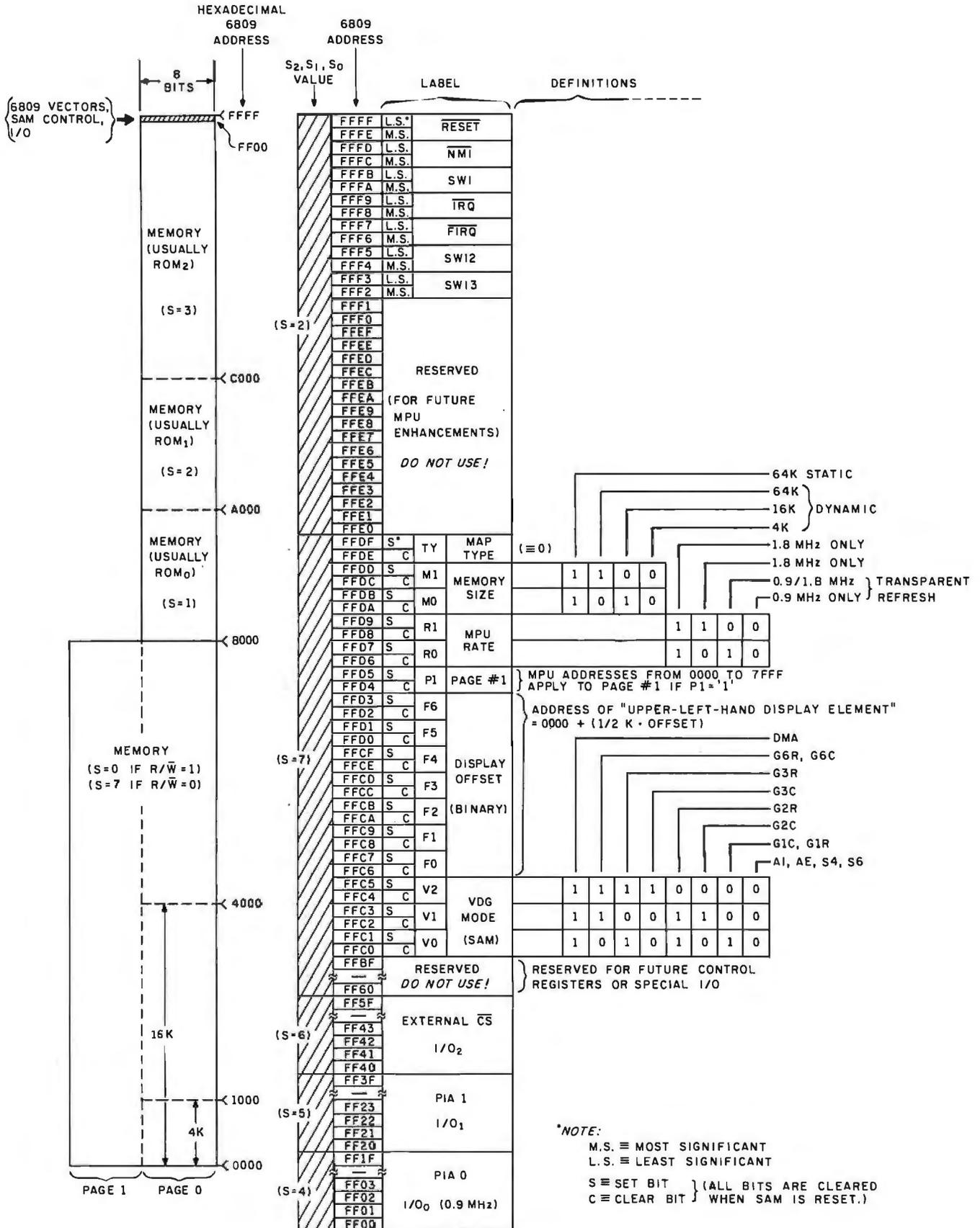
Figure 9: Memory map of the Color Computer address space. The general division of addresses is provided at the left, while the SAM programming registers and the processor-interrupt vectors are expanded at the right.
