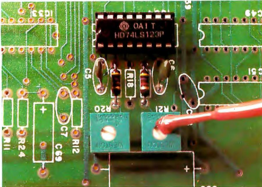
**Photo 4:** External-data-separator section of the Disk-80 board. An external data separator is recommended when using the FD1771 disk controller with the 5-inch floppy disks. This circuit (shown in figure 5) can also be added to the Radio Shack TRS-80 Expansion Interface to improve performance. After setting the adjustment potentiometers, use nail polish to lock their positions.
