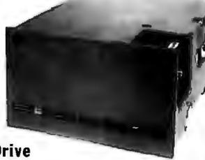
Packaged in the same physical size as the industry standard 5 1/4" minifloppy disk drive. The micro-Winchester stores thirty times as much data (6.38 megabytes unformatted), accesses data twice as fast (170 milliseconds) and transfers data twenty times faster (5.0 megabits per second.)
