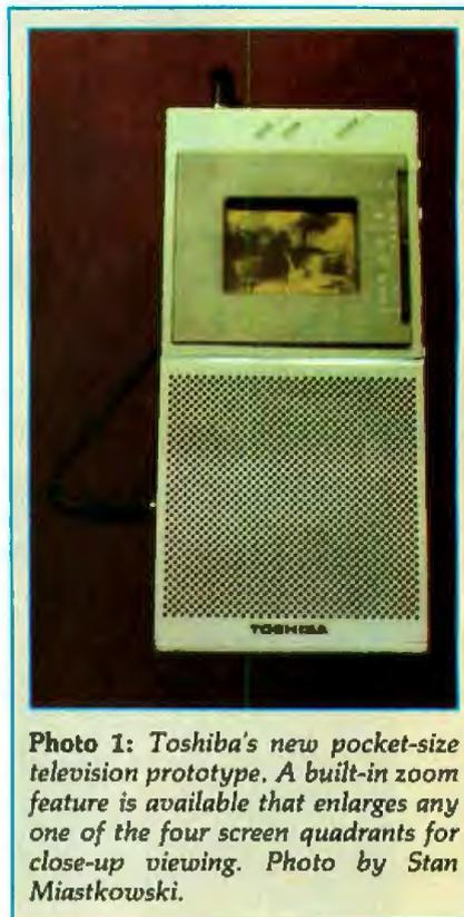
Photo 1: Toshiba's new pocket-size television prototype. A built-in zoom feature is available that enlarges any one of the four screen quadrants for close-up viewing. Photo by Stan Miastkowski.
