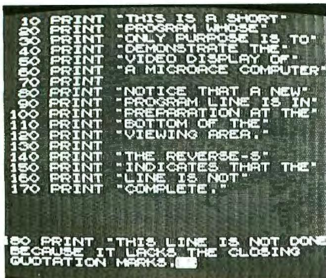
Photo 4: Sample program displayed on a standard color television set. The current program line is 180, as indicated by the reverse-video cursor.
