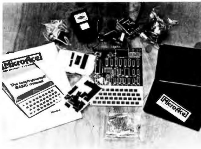
Photo 1: The MicroAce kit as shipped. Starting at the bottom and moving clockwise around the main circuit board are: the discrete components, the integrated circuit sockets, the integrated circuits themselves, voltage regulator, power supply, UHF modulator, antenna switch box, cable materials, and black plastic case. The 8- by 11 $\frac{1}{2}$ -inch instruction manual gives an indication of the size of this computer.
