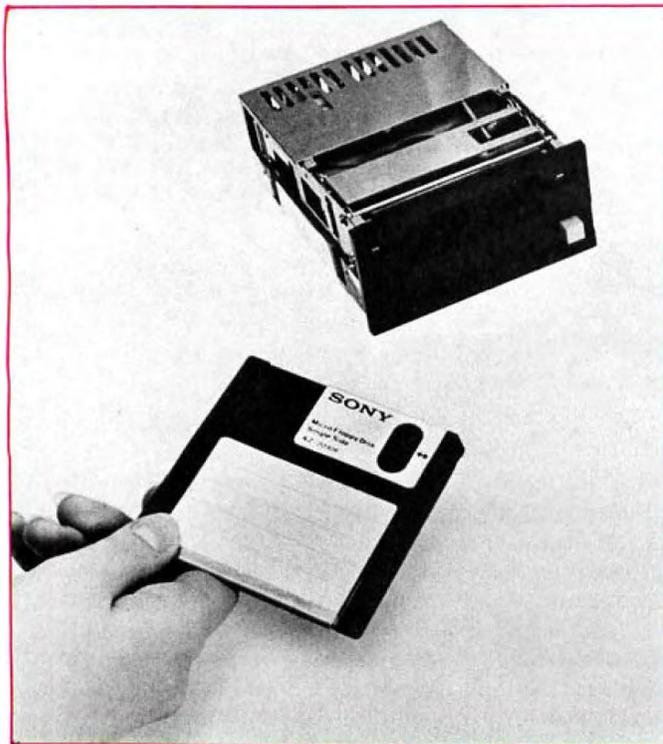
Photo 3: Sony's new 3 1/2-inch floppy disk and drive. Each double-sided floppy disk can hold up to 875 K bytes of information, unformatted. The recording density is 1.47 times that of the 5-inch disk.
