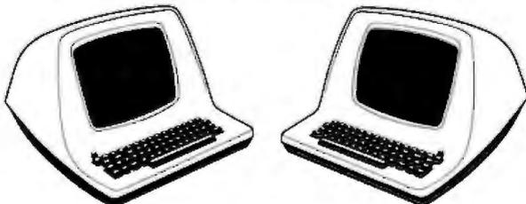
Display format 24 x 80—128 ASCII character set. Selectable transmission up to 19.2K baud. RS 232 interface. Typewriter standard type keyboard—59 keys.
