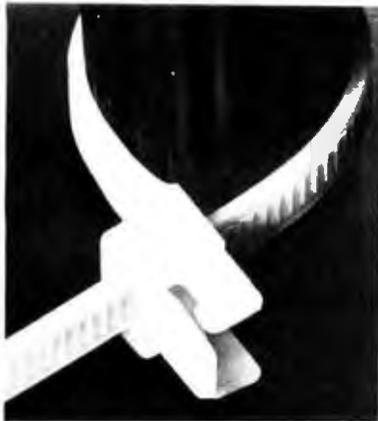
Courtesy Plastics has wire ties that feature release levers molded into locking heads. Squeezing this lever allows the tie to be adjusted or removed without damaging it. The tie can be reused later. These ties may be installed by hand or machine. They come in sizes for bundles up to 5 cm (2 inches) in diameter. The Release Wire Tie has a tensile strength of 50 lbs. For complete details, contact Courtesy Plastics, 250 Alice St, Wheeling IL 60090, (312) 541-7900. Circle 437 on inquiry card
