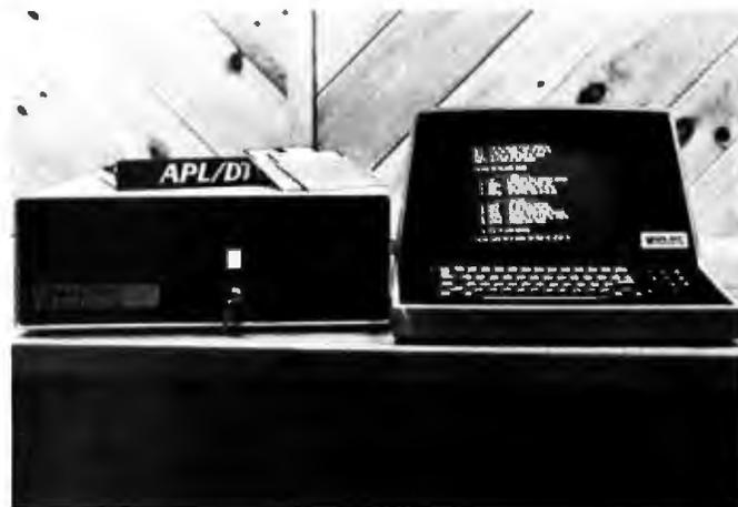
Photo 2: The Vanguard Systems Corporation APL/DTC. The system includes: the APL/DTC (desk-top) computer, on the left; its associated APL terminal, on the right; and, on top of the computer, documentation and two floppy disks of software—customized CP/M and Vanguard APL.
