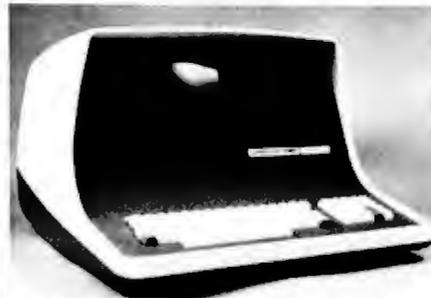
64K Double or Quad Density units available. Uses two Z-80 CPU's. Commercial-type terminal with 12" monitor. Dual double density minifloppies. Over 350 kilobytes of storage (twice that with quad density drives). Two serial RS232 ports, I/O ports standard. Expandable with optional S-100 S-100 interface. Comes with CP/M™ 2.2 operating system. MiniMicroMart can supply a wide range of CP/M development and application software.
