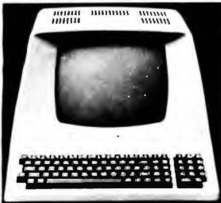
Upper and lower case, 15 baud rates: 75 to 19,000 baud, dual intensity, 24 x 80 character display, 12 x 10 resolution. Numeric pad. Programmable reversible video, auxiliary port, self-test mode, protect mode, block mode, tabbing, addressable cursor. Microprocessor controlled, programmable underline, line and character insert/delete. "C" version features typewriter-style keyboard. List \$950
