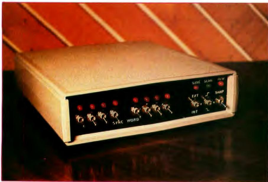
Photo 2: The prototype logic analyzer described in this article. The switches on the left are for setting the trigger (sync) word.
