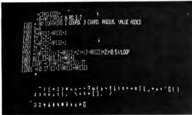
Photo 3: Listing of the APL function *CIRCLE* on the APL/DTC terminal screen and, below, a listing of special APL characters as they appear on the APL/DTC terminal. The last row is composed of characters that are created using an overstrike.
