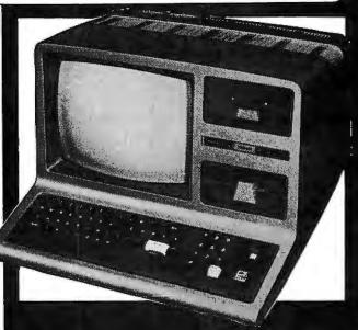
New low cost internal disk kit available to expand your storage capability. With this kit, now, you may expand your Model III computer up to four MTI 40 track disk drives, giving 175,000 bytes of storage per drive for a total of 700K.
