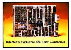
The secret behind our CompuStar DSS is its unique controller/multiplexor. It allows many terminals to "share" the resources of a single disk. So, not only can you use the DSS with your Super-Brain, you can configure multiple user stations using our new series of Compu-Star<sup>TM</sup> terminals, called Video Processing Units or VPU's<sup>TM</sup>.
