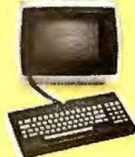
The new leader! Detachable keyboard, extra port, 3 function keys, numeric keypad, 24x80, RS-232C, built and backed by ADDS.
