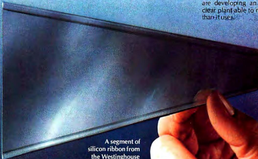
A segment of silicon ribbon from the Westinghouse dendritic web process
