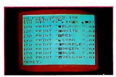
Photo 7: A VIC BASIC program utilizing color, graphics, and reverse video. This program produces the video display shown in photo 6b. The reverse character before each color word in the PRINT statements is a control character determining the color of everything displayed after it. See the text for details.
