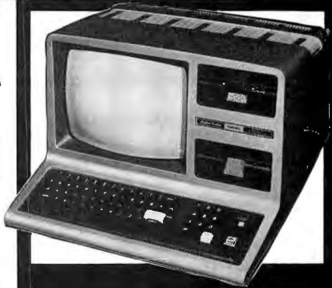
New low cost internal disk kit available to expand your storage capability. With this kit, now, you may expand your Model III computer up to four MTI 40 track disk drives, giving 175,000 bytes of storage per drive for a total of 700K.
