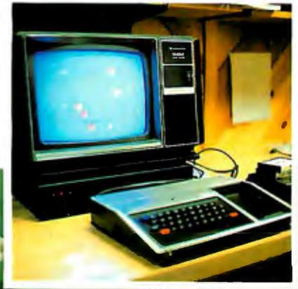
**Photo 1:** The TI Logo prototype (inset), including memory expansion, is contained in the black box under the monitor and behind the TI 99/4 computer. The final production version of TI Logo, which should be available later this year, will consist of a 32 K-byte memory expansion unit and a solid-state command module. (Photo courtesy of Texas Instruments.)
