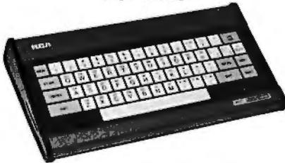
RCA's VP-3301 is a microprocessor-controlled terminal with color graphics, reverse video, programmable and resident character sets, selectable data rates and formats, a flexible-membrane keyboard, and audio feedback. The VP-3301 can be connected to modems for communication with most timesharing and data-base computer networks. The software-selectable character-display
