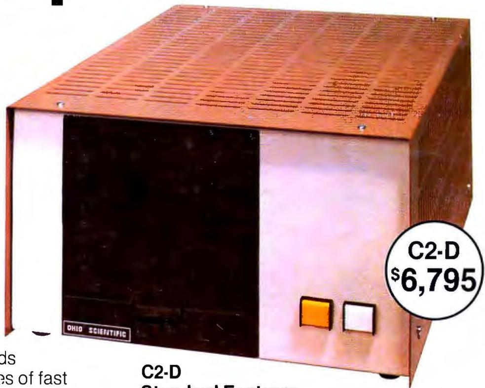
Ohio Scientific has put a low-cost, high-performance 8" non-removable hard disk together with its popular desk-top micro-computer system. This yields approximately 10 megabytes of fast hard disk capability at a tremendous cost/performance benefit over floppy based microcomputer systems.
