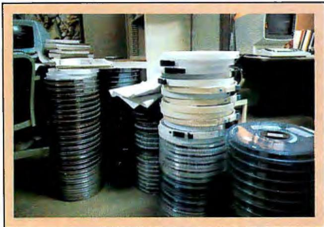
Photo 3: IBM reel-to-reel tape with new and updated data waiting to be placed on the Dialog system. Some twenty tapes arrive at Dialog each day from the outside organizations that prepare the data bases. Each tape contains approximately 20,000 individual references and/or abstracts.
