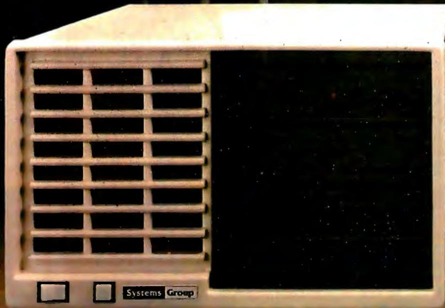
enhanced XIOS. The CP/M based System 2800 provides improved diagnostic reporting capability and increased sector sizes of 1024 bytes yielding disk performance throughput increases up to 400% over standard unblocked systems.
