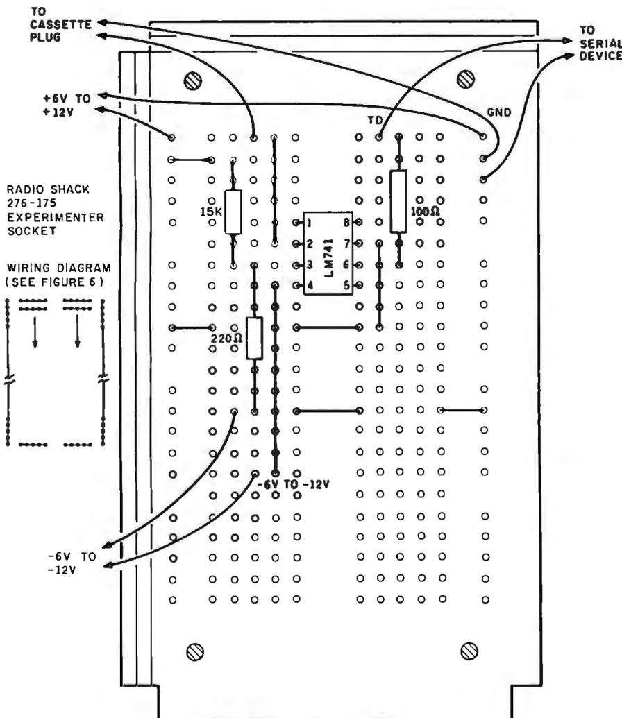
**Figure 16:** The SEROUT circuit is mounted on a project board. Two sets of power-supply connections are required.
