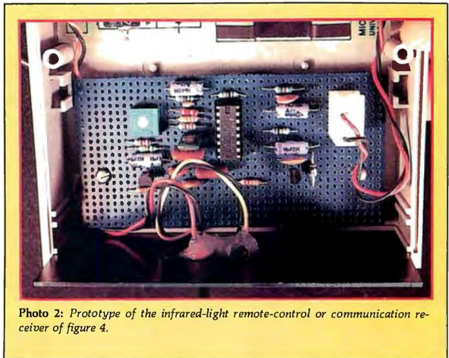
Photo 2: Prototype of the infrared-light remote-control or communication receiver of figure 4.
