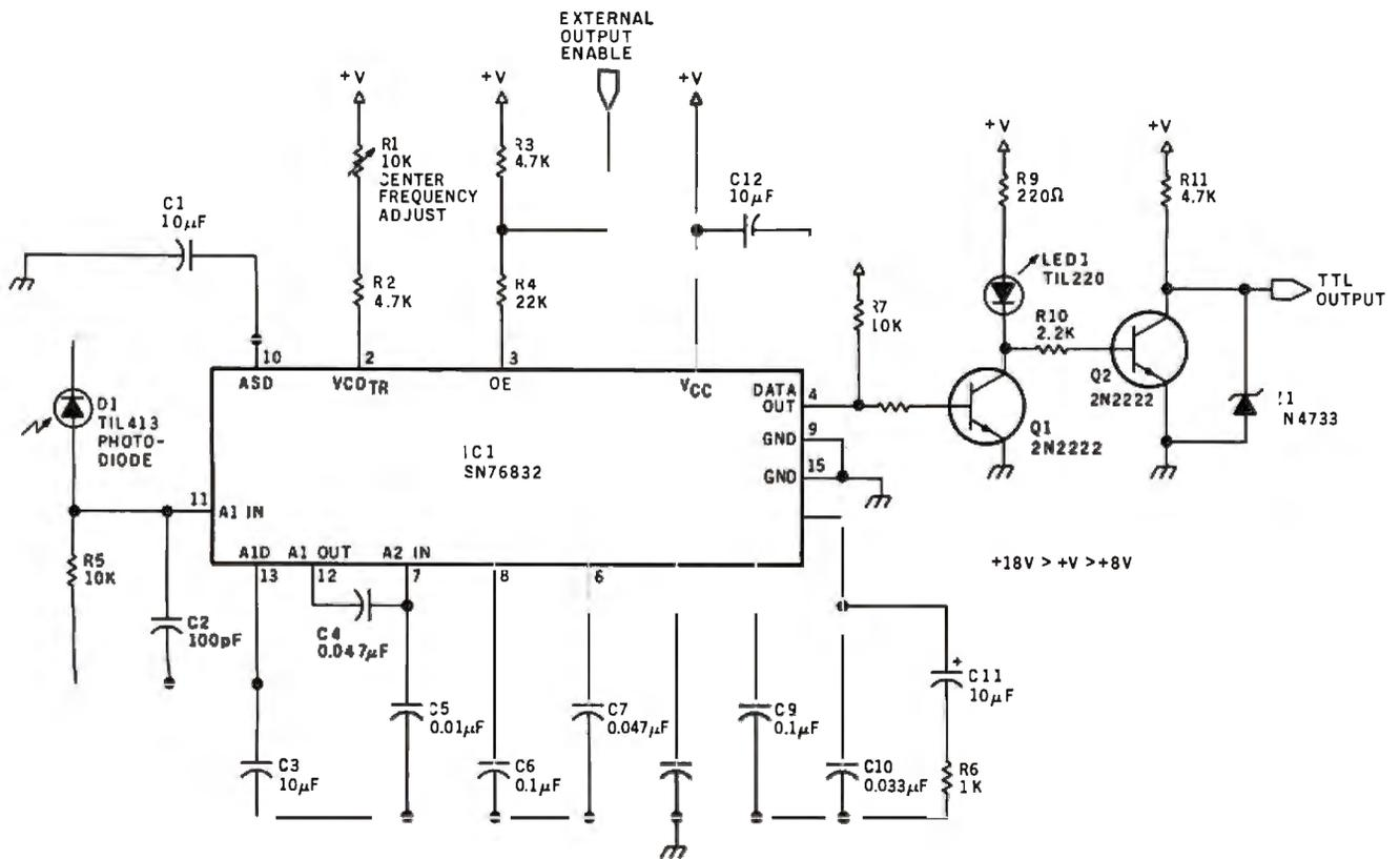
**Figure 4:** Schematic diagram of a remote-control or communication circuit based on the SN76832AN. This circuit is set up for use at 40 kHz, although the voltage-controlled oscillator can be adjusted from 20 kHz to 70 kHz. Any voltage from +8 V to +18 V may power the circuit.
