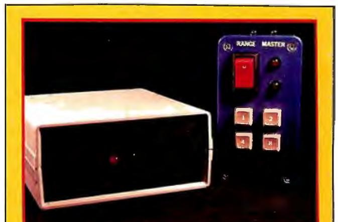
**Photo 4:** The assembled infrared remote-control/communication system. On the left is the infrared receiver; the transmitter is to the right. The TIL413 photodiode is the small projection to the right of center of the receiver's front panel; the small projection on the left is a visible red LED that lights when the infrared carrier is detected.
