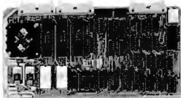
ECT's R<sup>2</sup>/O is an S-100 Bus I/O Board with 3 Serial I/O Ports (UART's), 1 Parallel I/O Port, 4 Status Ports, 2K of ROM with the 8080 Apple Monitor Program and 2K of Static RAM.
