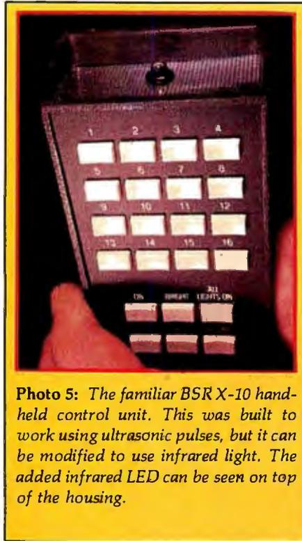
**Photo 5:** The familiar BSR X-10 hand-held control unit. This was built to work using ultrasonic pulses, but it can be modified to use infrared light. The added infrared LED can be seen on top of the housing.
