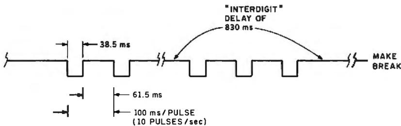
Figure 11: TELDIL breaks the circuit for 38.5 ms. Pulses are spaced at 100-ms intervals, representing 10 pulses per second. An interdigit delay of 830 ms separates the pulse trains for each digit.
