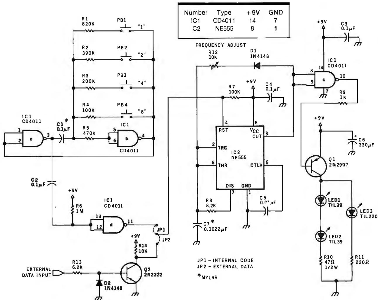
**Figure 5:** Schematic diagram of a handheld infrared remote-control transmitter. Four pushbutton switches actuate a NAND gate wired as an oscillator; different frequencies may be selected for testing or in communicating simple command functions. Two high-power infrared and one visible indicator light-emitting diodes are modulated at a carrier frequency of 40 kHz; control signals are sent as a simple on/off modulation of the 40-kHz-modulated light beam.
