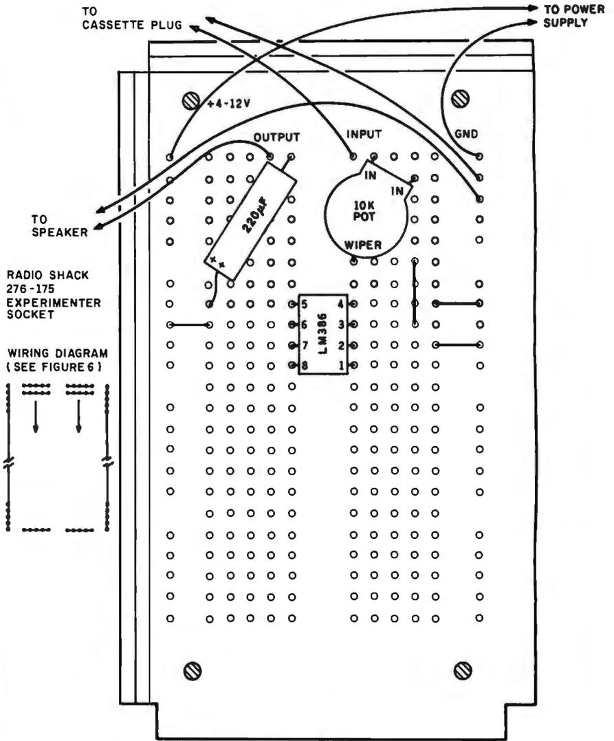
Figure 7: The TONOUT circuit is mounted on a project board. It uses three components. The 10-kΩ potentiometer can be adjusted for a comfortable volume.
