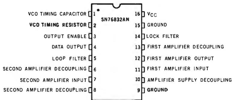
**Figure 3:** Block diagram of the internal structure of the Texas Instruments SN76832AN Infrared Remote-Control Receiver.
