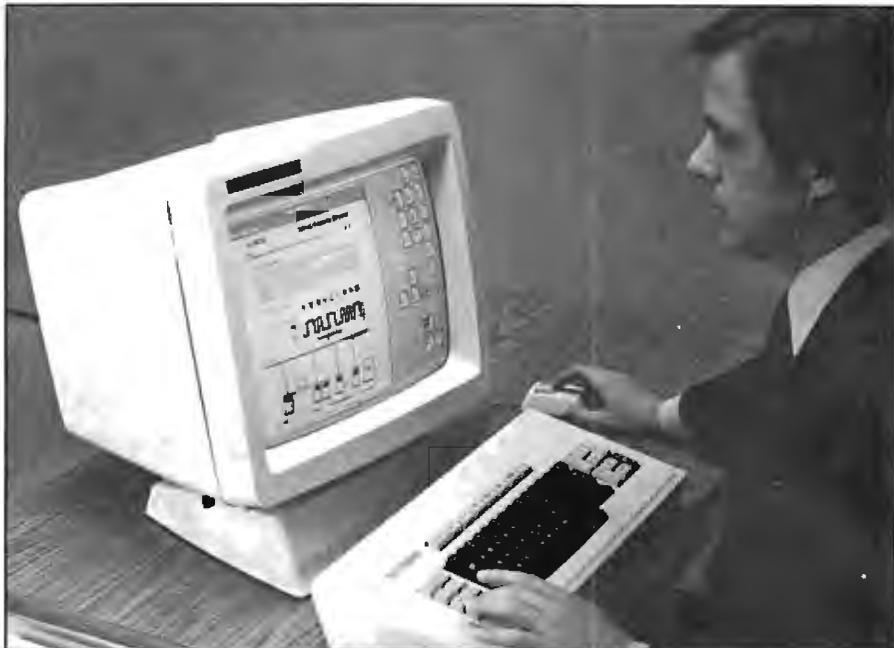
Photo 1: A Star work station showing the processor, display, keyboard, and mouse.
