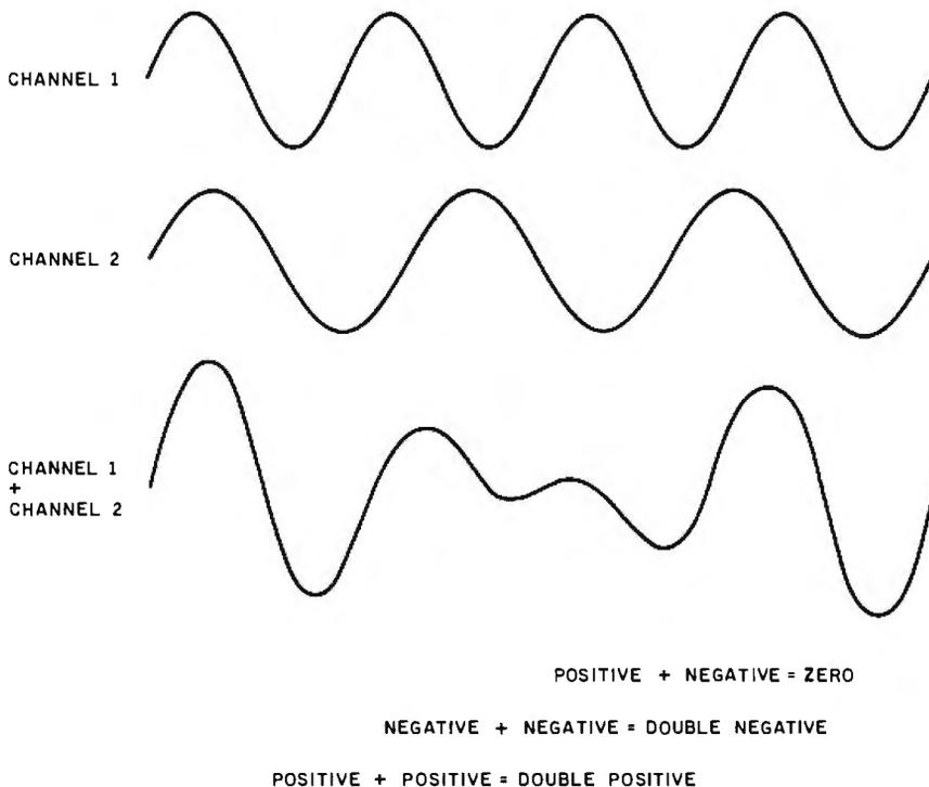
**Figure 1:** Complex waveform generation from the addition of waveforms.
