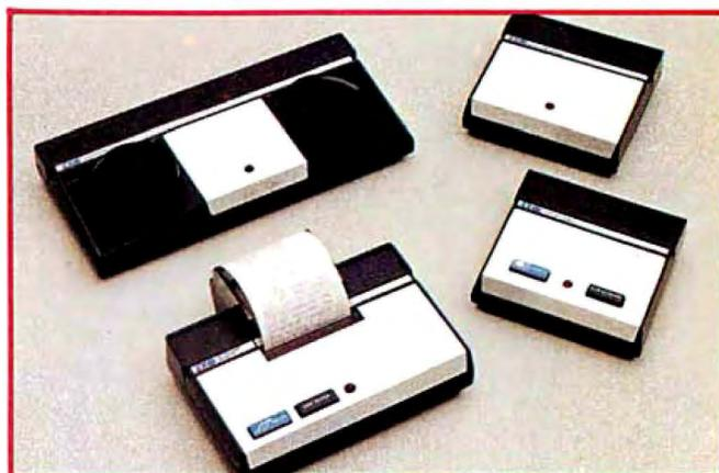
Photo 4: Four peripherals for the Telecomputer (clockwise from upper left): an acoustic interface (not the same as an acoustic coupler because the modem circuitry is already contained inside the terminal); the RS-232C interface, a video interface; and a 20-column printer.
