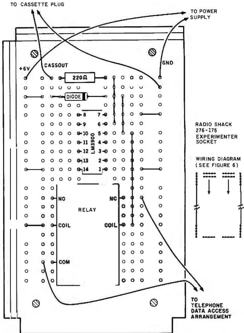
Figure 13: The TELDIL circuit is mounted on a project board. The relay leads can be trimmed, "built-up" with solder, and pushed into the project-board holes.
