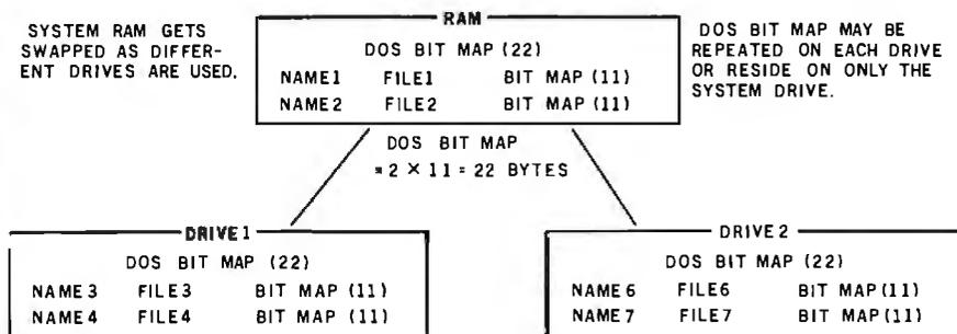
Figure 8: Swapping disk directories. As each disk is accessed, the disk directory is read from the disk and placed into RAM.
