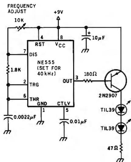
**Figure 6:** A simple circuit that provides only a 40-kHz carrier modulation for an infrared beam. This may be used for simple beam-breaking intrusion-detection schemes.
