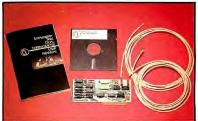
Photo 1: Strawberry Tree's complete package of temperature-monitoring equipment for the Apple.
