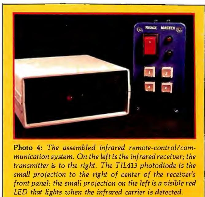
**Photo 4:** The assembled infrared remote-control/communication system. On the left is the infrared receiver; the transmitter is to the right. The TIL413 photodiode is the small projection to the right of center of the receiver's front panel; the small projection on the left is a visible red LED that lights when the infrared carrier is detected.
