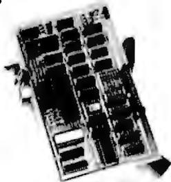
This printed circuit, small enough to fit inside the case of an IBM Model 50, 60, or 75 electronic typewriter, will interface with any RS232C computer system. The typewriter is still a typewriter, *and* an electronic communications system as well, with:
