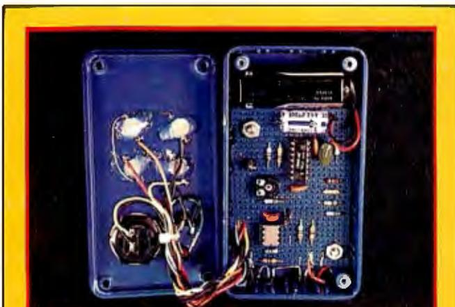
**Photo 3:** Prototype of the infrared transmitter assembly, internal view.
