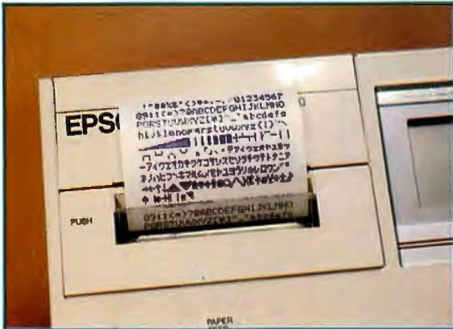
Photo 2: The HX-20 printer and a printout of its character set. The Japanese katakana characters will be replaced in the U.S. version of the unit by geometric symbols that can be combined to make larger graphic images.
