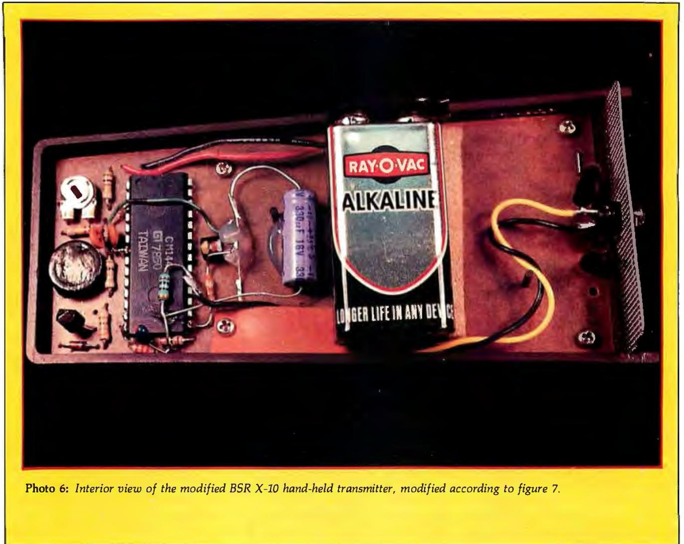
Photo 6: Interior view of the modified BSR X-10 hand-held transmitter, modified according to figure 7.
