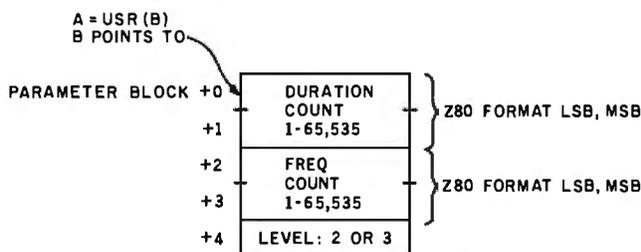
**Figure 5:** Three parameters are used to interface to TONOUT from BASIC. A duration count is held in two bytes, a frequency count in two bytes, and a level in one byte. The counts are in standard Z80 address format: least significant byte followed by most significant byte.
