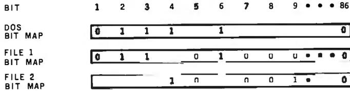
Figure 2: FORTHDOS bit map and file activity bit map. FILE1 is shown as using blocks 2, 3, and 6, while FILE2 is shown using blocks 4 and 9. The DOS bit map indicates which blocks are in use regardless of what file the blocks belong to; blocks 2, 3, 4, 6, and 9 are therefore indicated by the DOS bit map as being in use.
