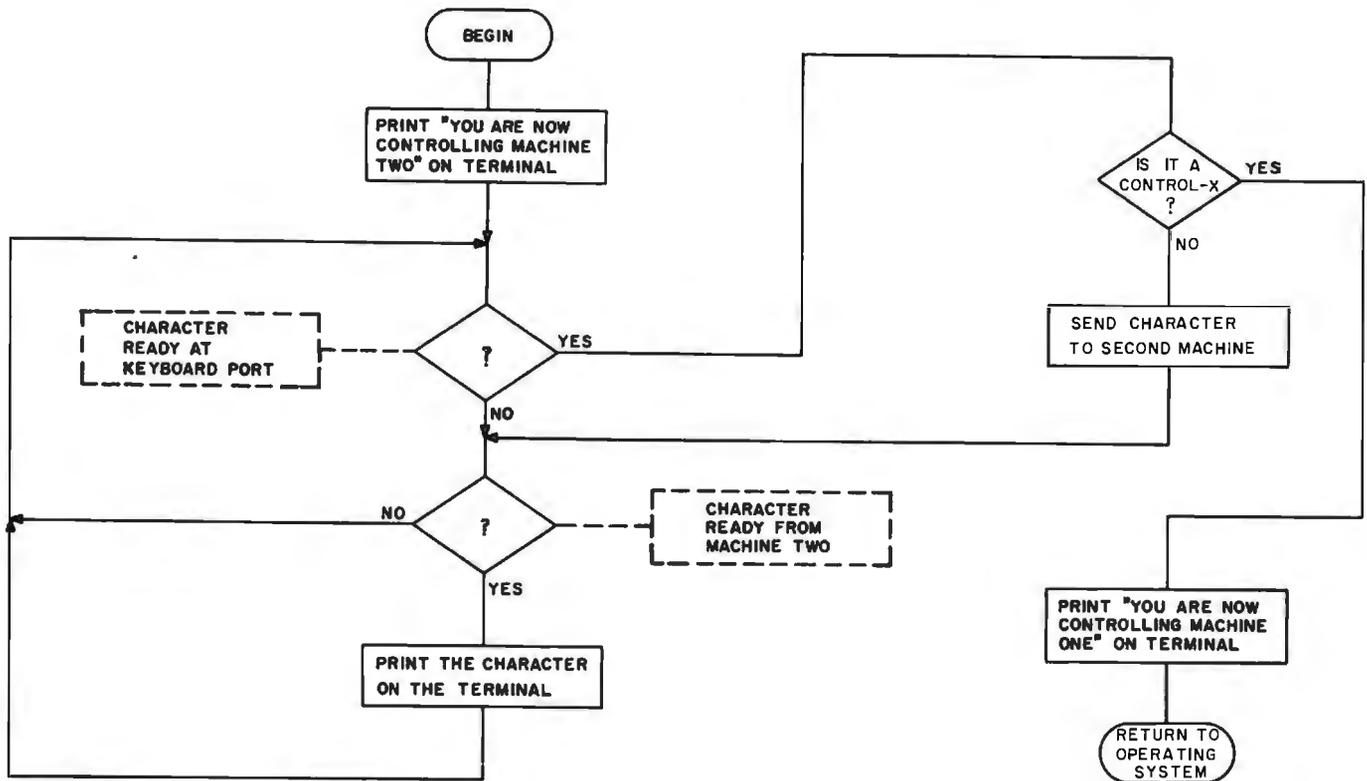
Figure 3: Flowchart of the algorithm used in the communications and control program given in listing 1.
