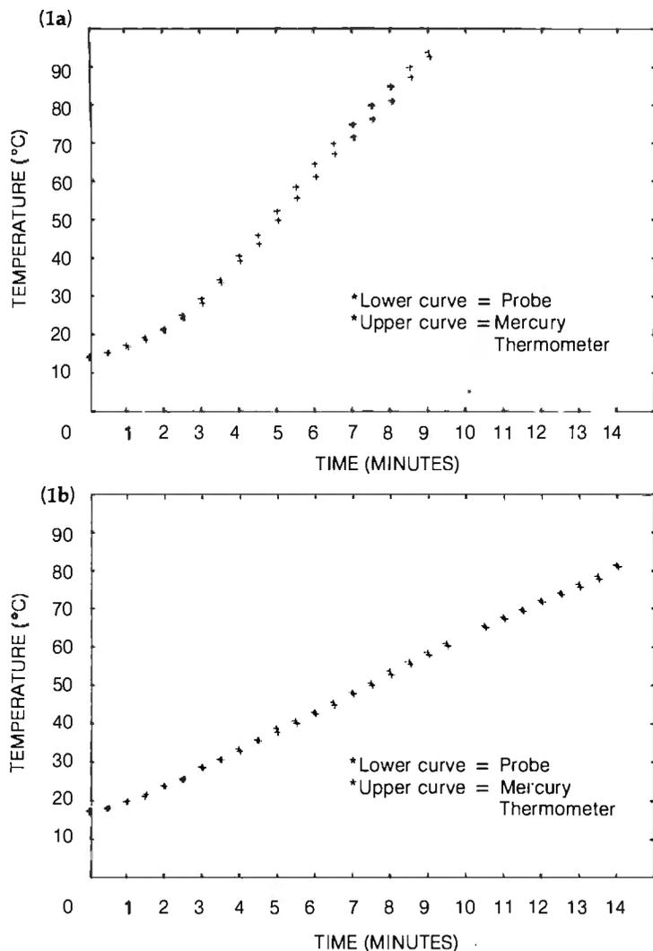
**Figure 1:** Tracking Strawberry Tree's thermometer probe versus a laboratory mercury thermometer. Figure 1a shows responses to an 8.89°C/minute rate of change; figure 1b shows responses to a 4.57°C/minute rate of change.
