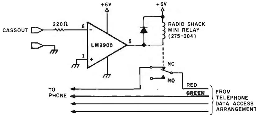
Figure 10: The telephone-dialing circuit uses an operational amplifier to trigger a small relay. The relay opens and closes the telephone line through the Data Access Arrangement to simulate a rotary-dial pulse.
