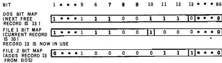
Figure 3: Using DNXT to find the next free record. As indicated in the DOS bit map, the next free record is 13. DNXT will scan the DOS bit map, find the free record, and change its corresponding bit to a 1.
