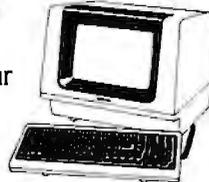
TV-Setup provides a user-friendly menu for setting up the terminal features and programming the function keys. The entire setup - including function keys - is then saved in a file for easy reprogramming each time you start up your system. You can have one setup for Wordstar, another for dBase II, another for SuperCalc, as many different setups as you want.
