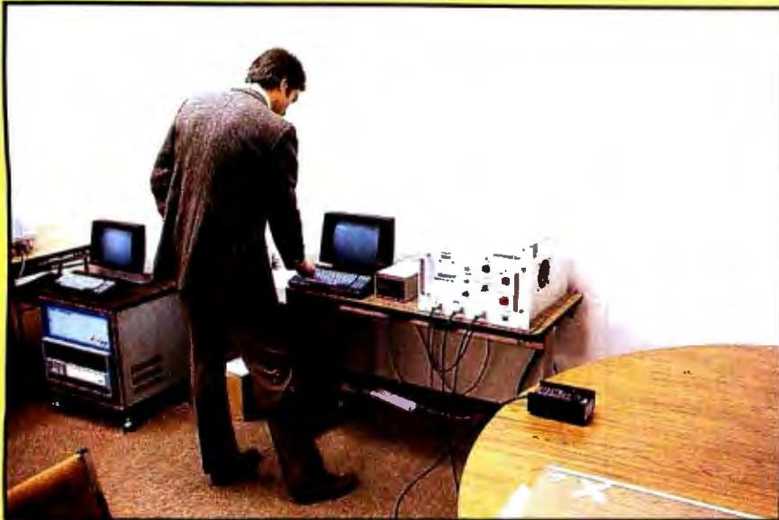
**Photo 8:** The control system of the Puma robot resembles a personal computer system.
