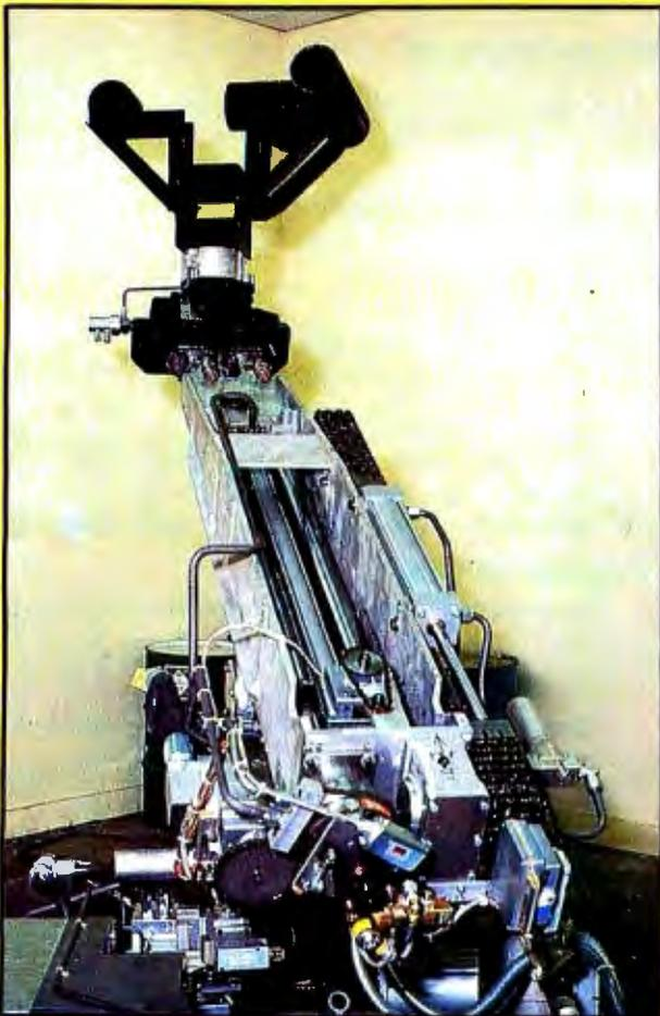
**Photo 6:** All Unimation robots are thoroughly tested before they are shipped to a customer. This robot is executing a sequence of steps with a 450-pound weight attached in order to test all motions.
