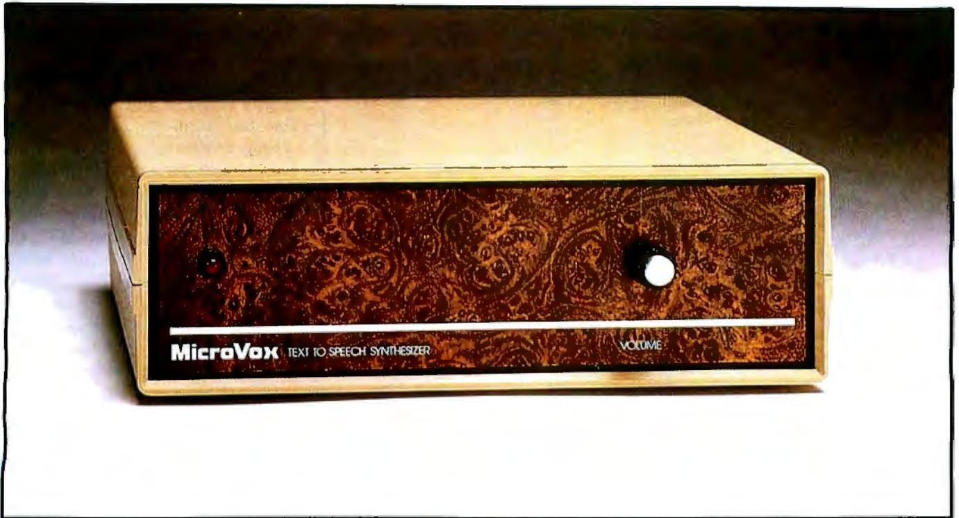
Photo 1: An assembled Microvox speech synthesizer, which can pronounce texts consisting of English words from their representation as ASCII characters according to fixed pronunciation rules. The Microvox contains a general-purpose 6502-based microcomputer programmed to control the Votrax-SC-01A-based speech-synthesis circuitry.
