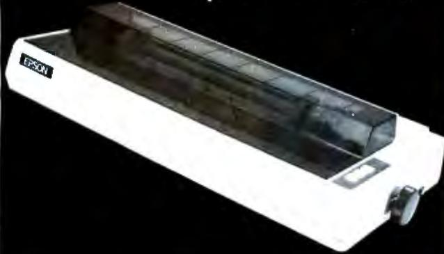
80 CPS, Bi-directional logic seeking 9x9 dot matrix, full 96 ASCII char. Set with true descenders, centronics-style parallel port (RS232 optional), 136 col., includes grafrax plus dot addressable graphics, friction feed and removable tractor feed. 21 lbs., 110 volt only.
