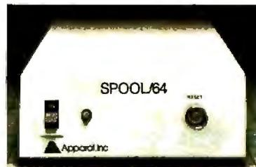
SPOOL/64 utilizes 64k of dynamic RAM, a Z-80 CPU, a 2716 ROM and a copy of the source program for the object code in the ROM is included.
