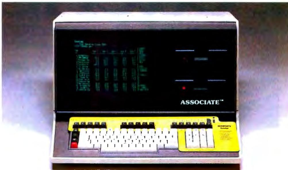
The ASSOCIATE is a field proven desktop microcomputer with many features: 64K memory plus 2K PROM; 720K bytes of floppy disk storage; Z80A 4Mhz processor; DMA disk controller, interrupt controller and timer; unique anti glare screen; typewriter style keyboard, numeric keypad and 10 function keys; and 2 RS232C ports. Optional parallel, IEEE 488, and RS449 ports give added flexibility. The remote or integrated hard disk option offers you needed growth capability.
