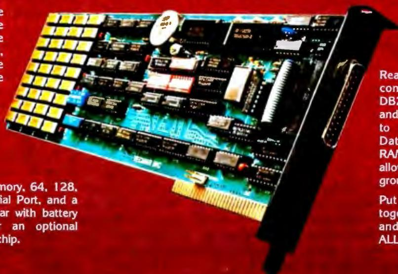
ALL IN ONE™ gives you memory, 64, 128, 192 or 256K bytes, a Serial Port, and a Parallel Port, Clock/Calendar with battery backup and circuitry for an optional Programmable Array Logic chip.
