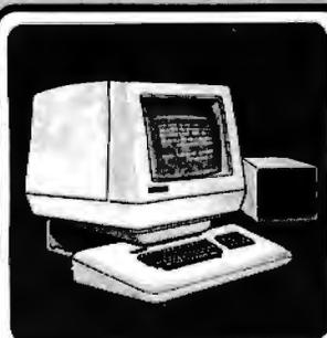
**FEATURES:** 4MHz, 280A, CP/M BASED, 64K RAM, 12" HI RES SCREEN (24 x 80), DD DISK CONTROLLER, THIN LINE GRAPHICS, ENHANCED SCREEN FEATURES (H/L INTENSITY, REVERSE VIDEO), TONE GENERATOR, 2 RS-232 PORTS, ONE PARALLEL PRINTER PORT, ALSO BOOTS AS INTELLIGENT TERMINAL.
