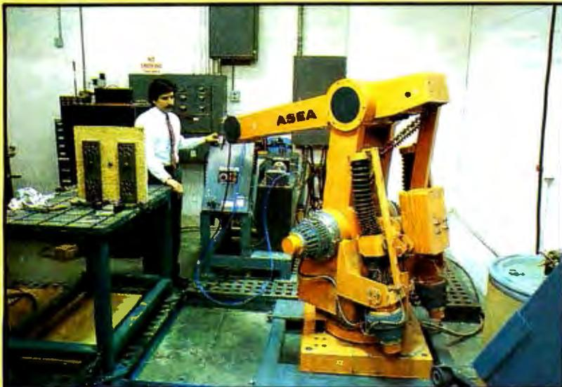
Photo 3: The ASEA robot model number IRb-60 shown here at the ASEA application laboratory in White Plains, New York, illustrates the revolute-arm geometry.
