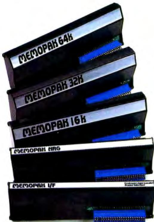
**Memopak 64K RAM** The 64K RAM extends the memory of your Sinclair by 56K to a full 64K. It is directly addressable, user transparent, is neither switched nor paged and accepts such basic command as 10 DIM A (9000). The Memopak 64K turns your Sinclair into a powerful computer suitable for business, recreational and educational use. No additional power supply is required.
