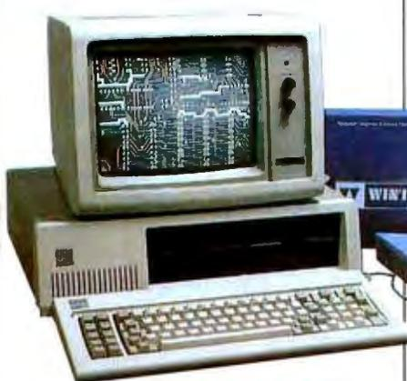
smARTWORK™ transforms your IBM PC into a CAD system for printed-circuit-board artwork. Display modes include both single-layer black and white and dual-layer color.
