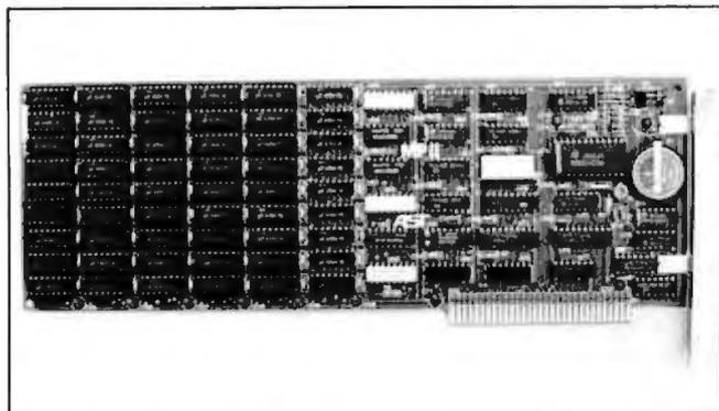
AST Research calls its MPII a "no frills" expansion card for the IBM PC XT. The MPII comes with 64K bytes of dynamic RAM, utility software, and a clock/calendar. Its memory capacity is upgradable to 348K bytes in 64K-byte increments. The price for the MPII ranges
