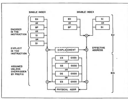
Figure 2: Addressing modes in the execution unit and bus-interface unit combine to form the physical address (see reference 4).
