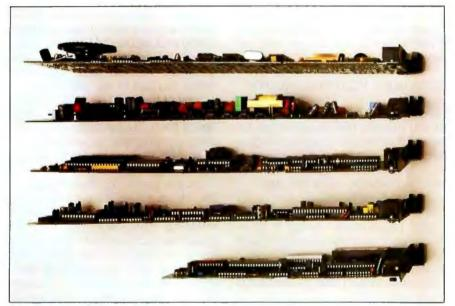
Photo 1: The thickness of the board configured with a speaker may concern you if you own an XT. From the top: Haues, Microcom, Novation, Bizcomp, and Cermetek.
