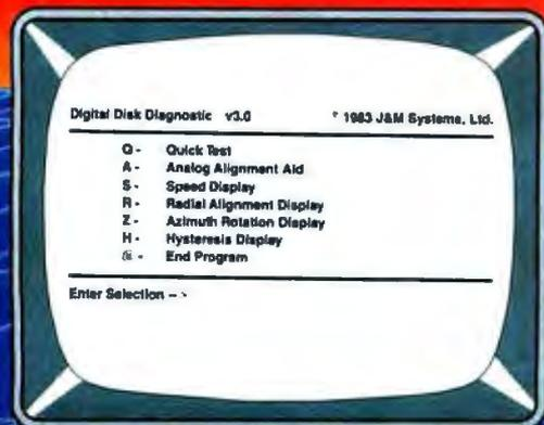
Select any one of seven tests to perform preventive maintenance or to isolate problems. Simple, single-letter commands make DDA easy to use! Use DDA to align the head, or adjust the speed.
