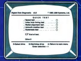
Use the Quick Test to quickly and automatically test five of the most important performance parameters of your drive. Monitor your drives for long term drift. Isolate problems quickly and automatically!
