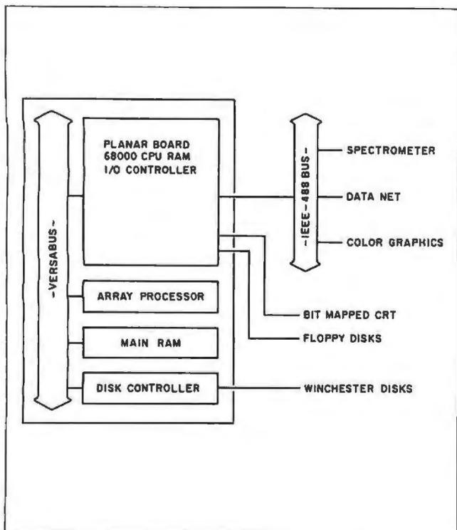
Figure 1: The architecture of the S9000 computer system used in the MIT NMR project. The 68000 CPU and SKY MNKV array processor share access to memory over the VERSAbus. You can use as much as 2 megabytes of memory in imaging applications.
