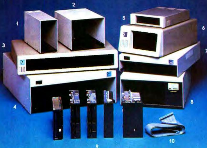
1. **Model # 5SVA&T** - Designed to house one full size or 2 half height 5 1/4" floppy disk drives in the vertical position. As an added feature, the mounting holes are duplicated in reverse so the user can mount the drives door left or door right. The power supply is a custom linear, proven in thousands of installations over the years!
