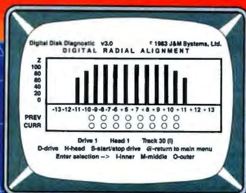
Use the DDA Radial Alignment Test to check the head alignment of your drives. No need for an oscilloscope or other expensive test equipment!
