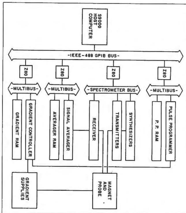
Figure 2: The electronics of a state of the art NMR imaging spectrometer. Nuclear spins in the sample probe are excited by RF pulses from the transmitter, and their response is recorded by the receiver and signal averager.
