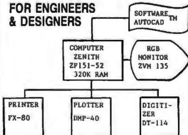
AutoCAD™ is a two-dimensional computer-aided drafting and design system suitable for many applications including drawings for architectural, mechanical, electrical, PCB layout, chemical, structural, and civil engineering.
