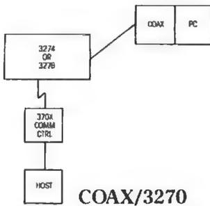
For instance, one solution is our Coax/3270. This single-slot expansion board lets you connect your IBM PC directly into virtually any IBM 3270 environment. And with our 3278/79 emulation software, it's easy to share information between your mainframe and IBM PC.
