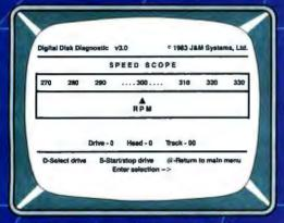
Check the motor speed of your drives. Or, you can even use the Speed Test to adjust the drive speed. No need for any test equipment!
