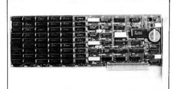
AST Research calls its MPII a "no frills" expansion card for the IBM PC XT. The MPII comes with 64K bytes of dynamic RAM, utility software, and a clock/calendar. Its memory capacity is upgradable to 348K bytes in 64K-byte increments. The price for the MPII ranges
