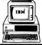
256K, one floopy Drive, Keyboard 10 MB Hard Disk with Controller
