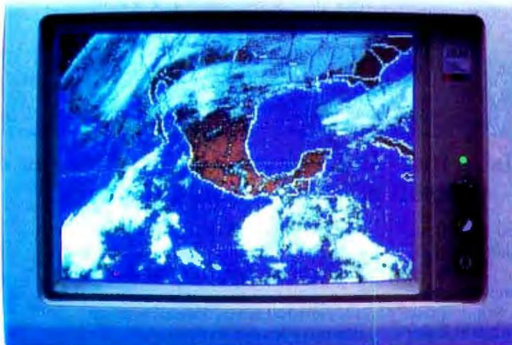
\*The B&W pictures are taken with a 35mm SLR camera. The pictures were captured with an RCA TC 1005 video camera on an IBM XT and sent to the monitor with a Tecmar Graphics Master™ graphics adaptor in the 640 x 400 x 16 level mode via its composite output
