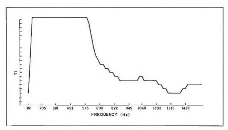
Figure 13: Frequency response with loudness filter on.
