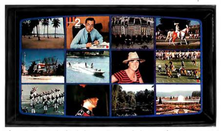
Photo 2: An example of multiple-picture-in-picture display using the  $5\frac{1}{3}$ : 3 aspect ratio CRT. The red dots in the two corners of the small windows indicate high-definition television display availability.
