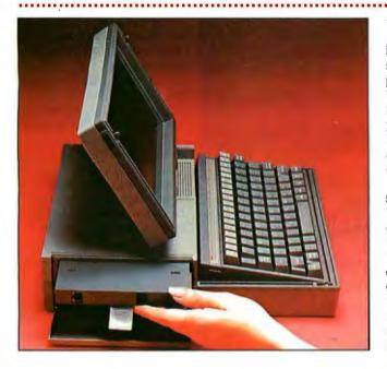
The briefcase-size Pro-Lite portable computer is compatible with Texas Instruments' Professional Computer. Pro-Lite includes one 720K-byte 3½-inch floppydisk drive, an 80C88 microprocessor, an 80-column by 25-line liquid-crystal display, and 256K bytes of memory, expandable to 768K.
