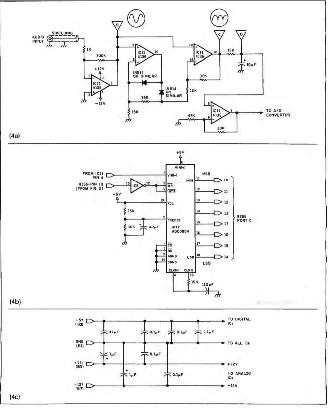
Figure 4: Audio input and full-wave rectifier (a), ADC (b), and power connections (c).
