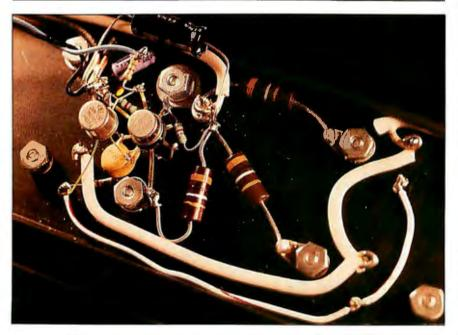
**Photo 1:** Short leads in the regulator sections limit noise pickup and add to overall stability. In my prototype, 1 connected the op amp and other discrete components directly to the regulators on the bottom side of the heatsink.
