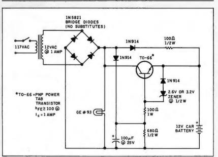
Figure B: A high-intensity lamp modification with backup power source and battery-charging capabilities. Schottky diodes must be used in the bridge in order to maintain adequate lamp brilliance. Any PNP power-tab mount (TO-66) transistor with a gain of 100 at 1 ampere will work with this design.
