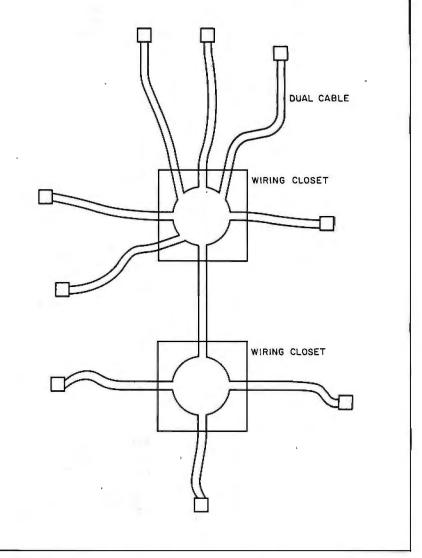
**Figure** 2: IBM's predicted local network uses a logical ring topology imposed on a star-shaped physical wiring setup, with a token-passing access protocol. Centralized wiring closets in the cabling system are well suited to use of optical fibers.
