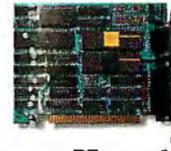
It gives you a parallel printer port and a size small enough to fit in one of the XT's or Portable's short slots.
