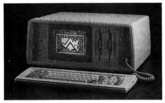
The Sanyo's screen accommodates 80 by 25 characters in regular mode and 40 by 25 characters in double-sized mode. The machine has 16-color graphics capabilities with 640- by 200-pixel resolution in color mode. In black-andwhite mode, resolution is 320 by 200 pixels. Bundled software for the MBC 775 includes EasyWriter 2, EasyMailer, EasyPlanner, and EasyFiler. Its operating system is MS-DOS 2.11, and it also features GW-BASIC.
