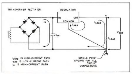
Figure 10: The proper power-supply layout.
