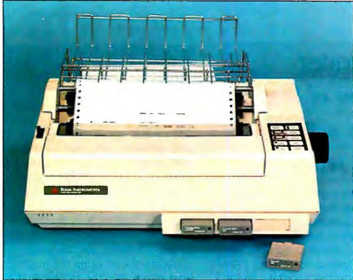
The Texas Instruments Omni 800/Model 855 printer provides both near letter-quality and draft-quality printing, with a variety of type styles available in removable font modules.
