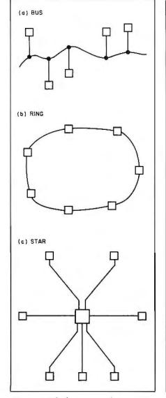
**Figure I**: The bus, ring, and star topologies (or connection configurations) shown in their idealized forms.
