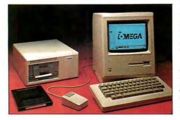
and 20-megabyte versions of the Bernoulli Box for the IBM PC and compatibles; the Mac Bernoulli Box is not compatible with the IBM version. Mac Bernoulli Box cartridges can be exchanged with any other Macintosh. however, allowing transfer of large quantities of data on a single disk. The 5-megabyte cartridges are physically smaller than the 10- and 20-megabyte cartridges.
