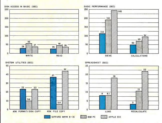
The graph for Disk Access in BASIC shows how long it takes to write a 64K-byte sequential test file to a blank floppy disk and how long it takes to read this file. (For the program listings, see the June BYTE, page 327, and the October BYTE, page 33.) The BASIC Performance graph shows how long it takes to run one iteration of the Sieve of Eratosthenes prime-number benchmark. In the same graph, the Calculations results show how long it takes to do 10,000 multiplica-
