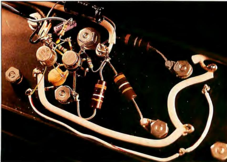
Photo 1: Short leads in the regulator sections limit noise pickup and add to overall stability. In my prototype, I connected the op amp and other discrete components directly to the regulators on the bottom side of the heatsink.
