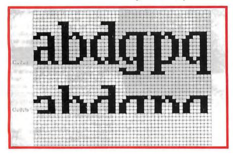
forms on most computer terminals usually provides a single size of a single style of coarse-resolution dotmatrix letters. Character-generator technology usually does not let the user modify the fonts because the character images are contained in hardware or firmware.
