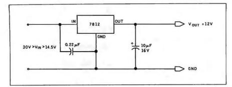
Figure 5: A typical +12-V fixed-voltage output regulator.
