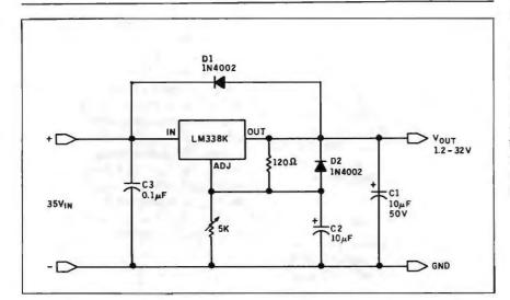
Figure 6: A typical variable-voltage three-terminal regulator.
