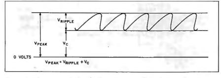
Figure 4: The components of peak voltage,  $V_{peak}$ , are the steady-state voltage,  $V_c$ , and the ripple voltage,  $V_{ripple}$ .
