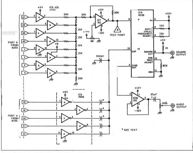
Figure 3: Voltage-controlled oscillator and driver circuitry.
