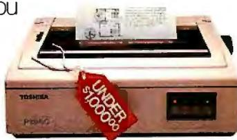
**An impressive eye for detail.** The Toshiba P1340 doesn't just give you high speed, letter-quality type. At 180 x 180 dots per square inch, it also gives you high-resolution graphics that lead the industry.
