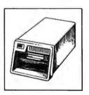
ADS 8218 5.25 inch tape backup system is designed to back-up data from an IBM PC with an internal or external hard disk system or an IBM XT. ADS 8218 offers an easy to use, A1. AUS belt oners an easy to use, reliable high speed tape backup at an affordable price. The system is attached to the PC externally and comes complete with interface and controller boards, cables and easy step-by-step instructions for a fast and simple installation. Available in 40/60 MB formatted.
