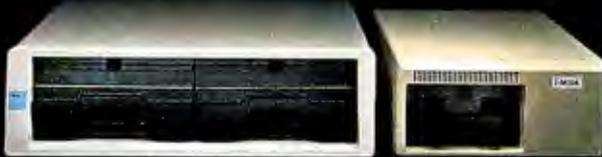
With one notable exception. The Bernoulli Box™ from IOMEGA. Available for the IBM PC, XT, most compatibles, the TI Professional, and Apple's Macintosh,™ the Bernoulli Box delivers unparalleled data base dynamics. Thanks to its removable 10-megabyte cartridges (5-megabyte for the Macintosh) and its proprietary removable disk technology.
