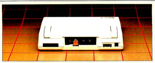
The rear panel of the HP 110: From left to right are the HPIL's in and out ports, the AC recharger connector, the battery compartment (usually covered), the serial port, and the modem phone jack.
