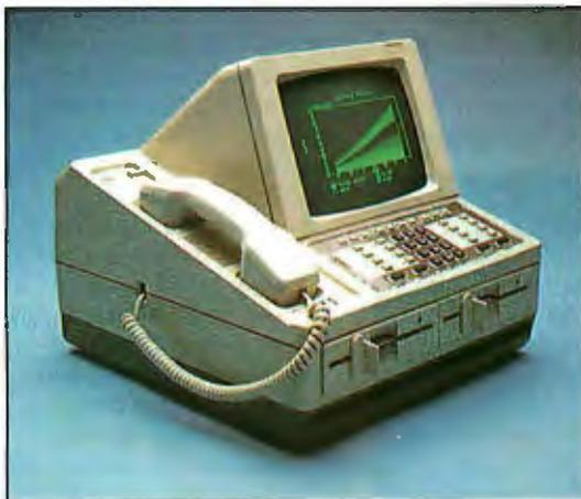
tached to the CBX system to communicate with the outside world. The system includes 512K bytes of memory, two 5¼-inch disk drives, a 9-inch monitor, and MS-DOS 2.11.
