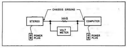
Figure 6: Potential ground problem test configuration.
