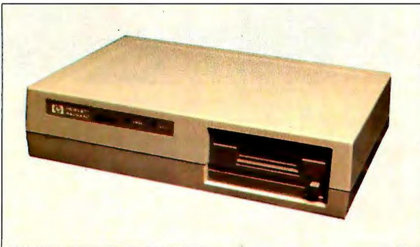
Photo 5: The HP 9114 portable disk drive contains a 3½-inch, double-sided Sony disk drive capable of storing over 680K bytes of data. Also included is a lead-acid battery and interface electronics.
