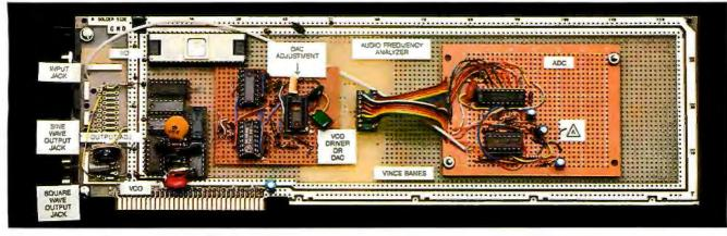
Photo 1: Audio-frequency analyzer board.
