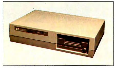
Photo 5: The HP 9114 portable disk drive contains a  $3\frac{1}{2}$ -inch, double-sided Sony disk drive capable of storing over 680K bytes of data. Also included is a lead-acid battery and interface electronics.
