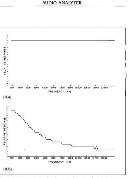
**Figure** 10: Straight connection through a resistor divider network (a);  $0.47 \mu F$  capacitor across the input (b).
