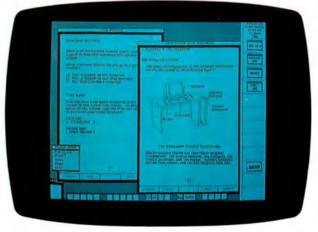
Photo I: Display screen of the VAX station 100, a workstation made by Digital Equipment Corporation. The proportionally spaced screen fonts on the VAX station are members of the Pellucida family, a set of original typeface designs optimized for legibility and clarity on bit-mapped computer displays. The characteristics of the Pellucida digital letterforms were developed by Charles Bigelow and Kris Holmes.
