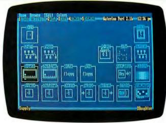
an optional mouse. With Port, network users can share printers and other peripherals. Diskless workstations can download software, including the operating system, through the network.
