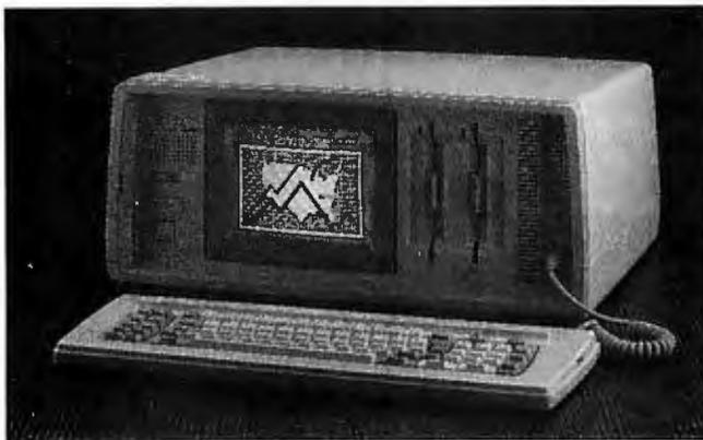
The Sanyo's screen accommodates 80 by 25 characters in regular mode and 40 by 25 characters in double-sized mode. The machine has 16-color
