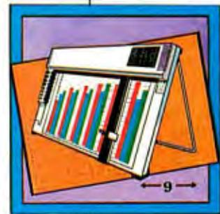
**I**s limited desk-top space a problem? The DXY-880 also stands up to run at a 60 degree angle—perfect for a bookshelf. You can even reverse the plotting process and use the DXY-880 as an input device by activating the built-in multi-speed digitizer.
