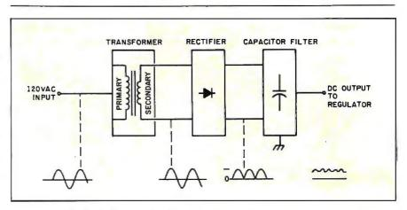
Figure 3: The block diagram of a filtered power supply.
