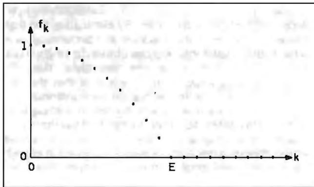
Figure 1: When the digital filter function is incorporated into the FT algorithm, it eliminates all frequencies corresponding to  $k \geq E$  from the discrete Fourier transform spectrum. Frequencies corresponding to  $k < E$  are gradually attenuated.
