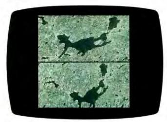
Photo 2c: Upper portion is original data, lower portion has been rectified to a base map.
