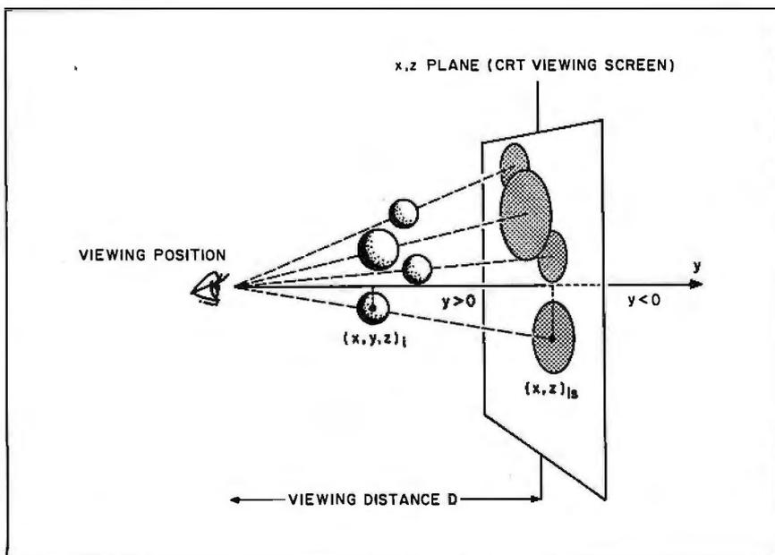
Figure 1: A perspective view of a three-dimensional object as projected onto a two-dimensional CRT screen. The point  $(x,y,z)_i$  represents the center of a 3-D sphere, and  $(x,z)_is$  represents the projected screen coordinates.
