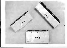
For connecting several printers to one computer port or for connecting one printer to several computers. Our Centronics and RS232 transfer switches are designed to last a lifetime. The internal slide switch is a high quality dust sealed type with a life expectancy of 15.000 operations (sliver/sliver alloy contacts). The RS232 and IBM compatible parallel transfer switches employ female connectors (DB25S style) with gold plated contacts and have hex female stand offs installed.
