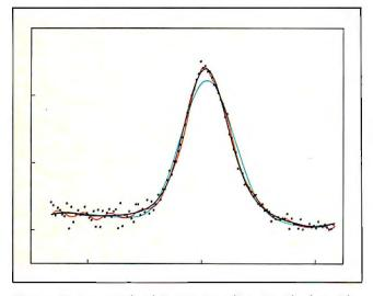
Figure 2: An example of Fourier smoothing scientific data. The data represents a derivative neopolarogram at a static-mercurydrop electrode. The black line, showing proper smoothing, was obtained by N = 72, E = 8. In the red line, showing undersmoothing, E = 20. In the oversmoothed blue line E = 4.
