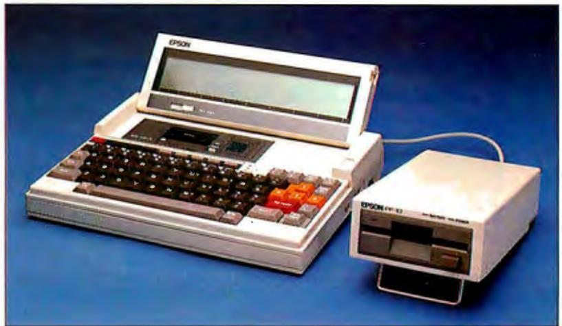
Photo 1: The Epson Geneva PX-8 computer, shown with optional battery-powered 3 1/2-inch floppy-disk drive. Note the internal microcassette drive located between the keyboard and the display.
