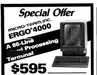
ERGO® 4000 is the ASCII Terminal featuring 80-column by 66-line format for full-page display capability. Features include: 15 downloadable function keys, four video attributes, pass-through printer port, screen saver, alternate character generator, settable tabs, 24-line display, and user-definable custom mode. (Compatible with VT100 codes.) Most popular word processing packages are already modified to run on the ERGO® 4000.
