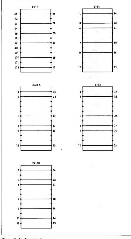
Figure 5: Configuration jumpers.
