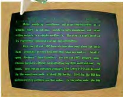
TTL Monochrome Mode: 640 dots x 350 lines
