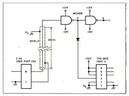
Figure 2: TTL (transistor-transistor logic) to RS-232C-level conversion.
