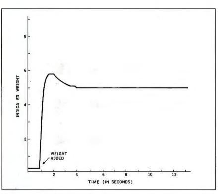
Figure 9: The integral partially offsets the effect of rate damping so you get quicker response and some overshoot, which is quickly damped out. You can't see the reduction of the weight beam's angular error in this plot of indicated weight versus time, but including the integral Q increases the scale's accuracy.
