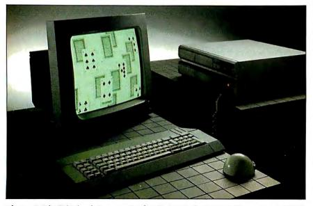
Photo 1: The Whitchapel Computer Works MG-1 uses the National Semiconductor 32016 32-bit virtual-memory processor chip.
