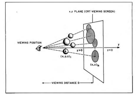
**Figure 1:** A perspective view of a three-dimensional object as projected onto a two-dimensional CRT screen. The point  $(x,y,z)_i$  represents the center of a 3-D sphere, and  $(x,z)_i$  represents the projected screen coordinates.
