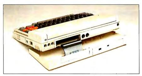
Photo 4: The optional memory-expansion module for the Epson PX-8, shown ready to attach to the bottom of the computer.
