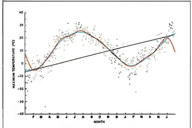
Figure 3: Daily maximum temperatures at the Peterborough, Ontario, weather station from January 1982 through June 1983. The red line ( $N = 546$ ,  $E = 9$ ) provides an example of false smoothing due to an "end effect." To correct for this effect, subtract a straight line (black) joining the ends of the unsmoothed data. The resulting "normalized" smoothing is shown by the blue line ( $E = 7$ ).
