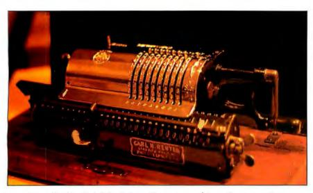
Photo 2: A hand-cranked desk calculator, like the one used by Wilkinson to perform numerical analysis during World War II. This machine was manufactured by Brunsviga.
