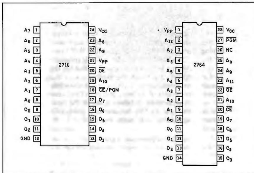
Figure 1: Pinouts of the 2716 and 2764 EPROMs.
