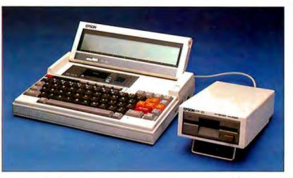
Photo I: The Epson Geneva PX-8 computer, shown with optional batterypowered 31/2-inch floppy-disk drive. Note the internal microcassette drive located between the keyboard and the display.
