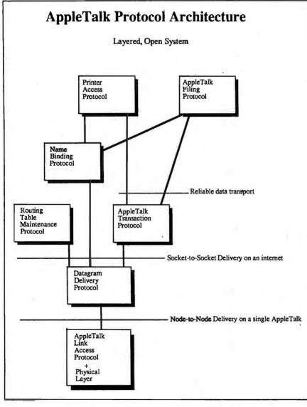
Figure 1: A diagram of AppleTalk's protocol architecture. printed by the LaserWriter.
