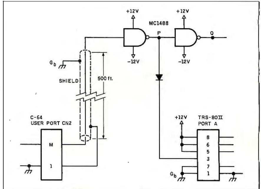
Figure 2: TTL (transistor-transistor logic) to RS-232C-level conversion.
