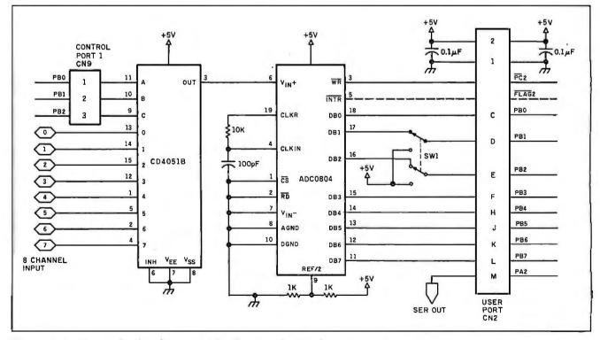
Figure 1: A schematic for the A/D converter for the Commodore 64 data-acquisition system.
