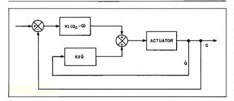
**Figure 6:** A proportional-plus-rate system uses the output variable's rate of change as part of the control calculation.
