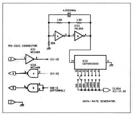
Figure 3: Serial interface and data-rate generator.
