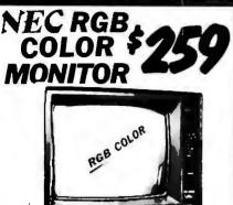
The NEC JC-1401D s a 13<sup>°°</sup> medium/high resolution RGB monitor suitable for use with the Sanyo MBC-550/555 or the IBM/PC. The monitor features a resolution of400 dotsby240 lines. Colors available are Red, Green, Blue, Yellow, Cyan, Magenta, Black and White. These monitors are currently being used in applications tar more
