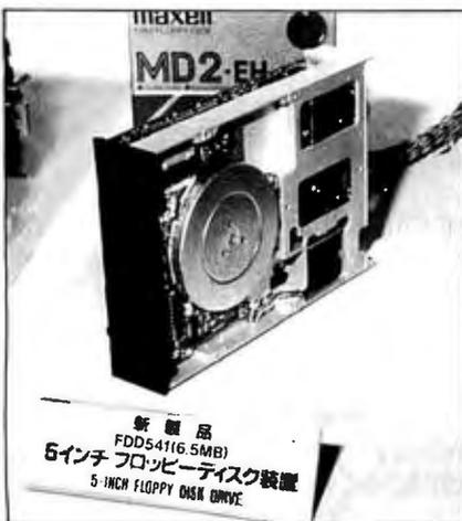
Photo 1: The 6.5-megabyte floppy-disk drive from Hitachi.
