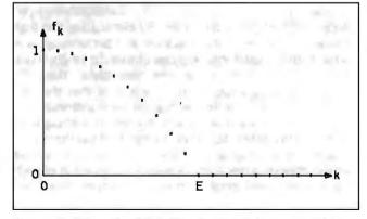
Figure 1: When the digital filter function is incorporated into the FT algorithm, it eliminates all frequencies corresponding to  $k \ge E$  from the discrete Fourier transform spectrum. Frequencies corresponding to k < E are gradually attenuated.
