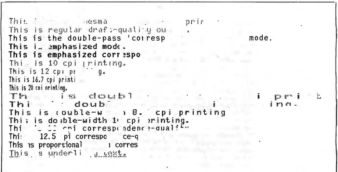
Figure 1: Print samples from the Mannesmann Tally MT 160 printer.
