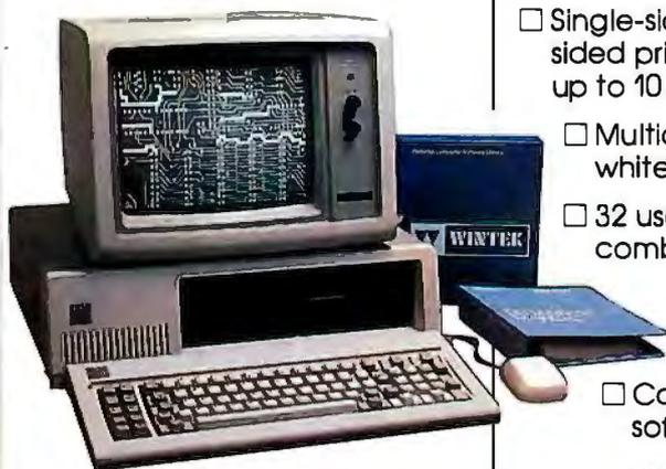
smARTWORK™ transforms your IBM PC into a CAD system for printed-circuit-board artwork. Display modes include both single-layer black and white and dual-layer color.
