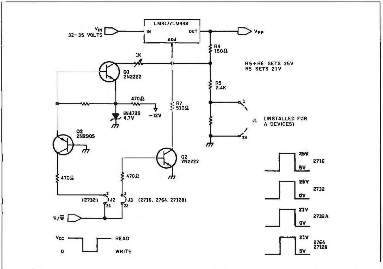
Figure 6: Close-up of the programmable  $V_{pp}$  supply.
