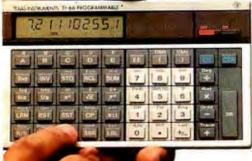
from Texas Instruments. The TI-66 offers full programming power and flexibility so you can handle complex and repetitive math problems quickly, easily, and with fewer keystrokes.
