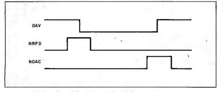
Figure 2: The logic flow of the IEEE-488 handshake squence. Low is true.
