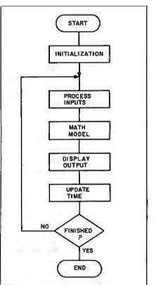
Figure 3: A typical simulation-program flowchart.
