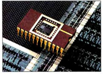
information in a given frequency range: Kurzweil says that dozens of filters—or many 2408 chips—would be needed to divide up the frequency spectrum of the human voice enough to make speech recognition possible.
