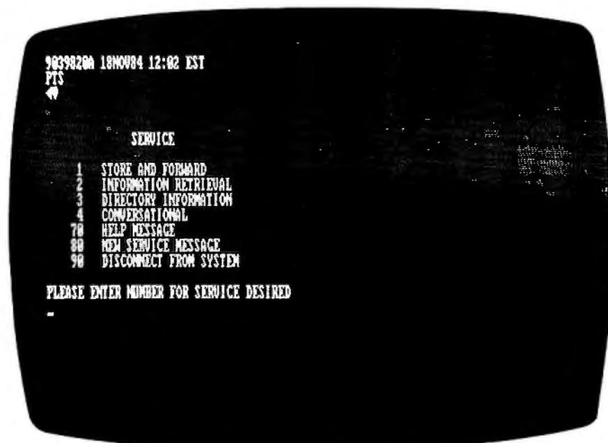
Photo 2: Entry-level prompt and help menu for EasyLink. You enter commands by typing a slash and a command word, such as /SCAN to list all messages, /READ to read a message, or /HELP for the help files.
