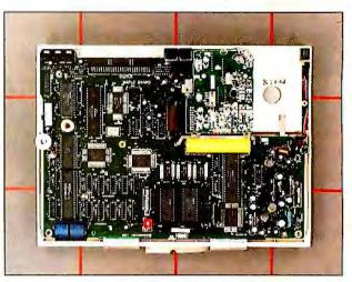
A look inside the PX-8 shows the processor chips (left) and the ROM chips (lower center).
