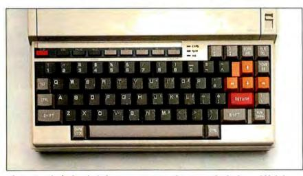
Photo 3: The keyboard of the Epson PX-8. In this picture the display is folded down over the microcassette drive. Note the second Control key to the right of the space bar and the caps-lock, num-lock, and insert-mode indicators above the zero key.
