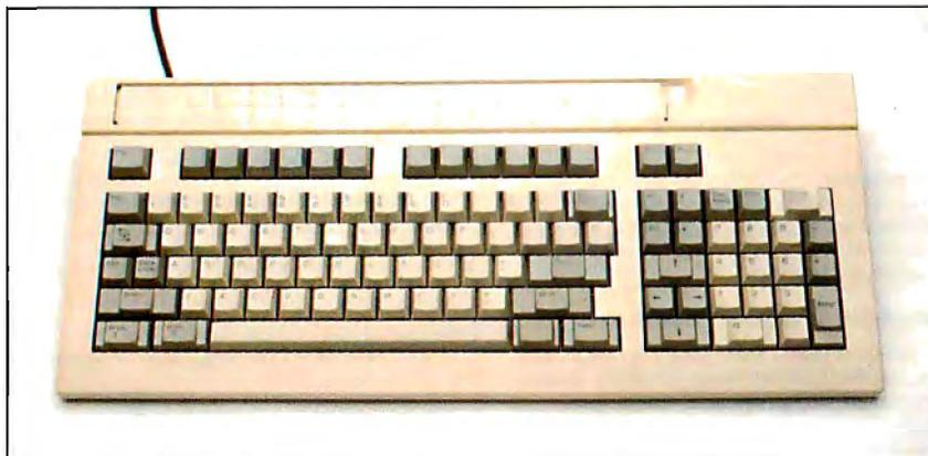
Photo 4: The APC III keyboard. Note the 12 unlabeled programmable function keys and the template for recording the functions.
