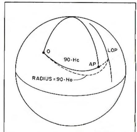
Figure C: In this case  $90 - H_o$  is greater than  $90 - H_c$ . Your actual position lies on an arc (LOP) of a circle of center  $O$  and radius  $90 - H_o$ .
