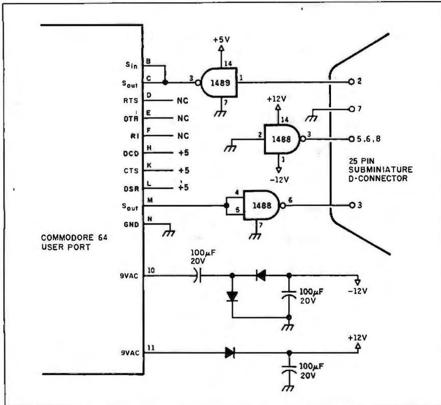
Figure 3: A schematic of the RS-232C interface.
