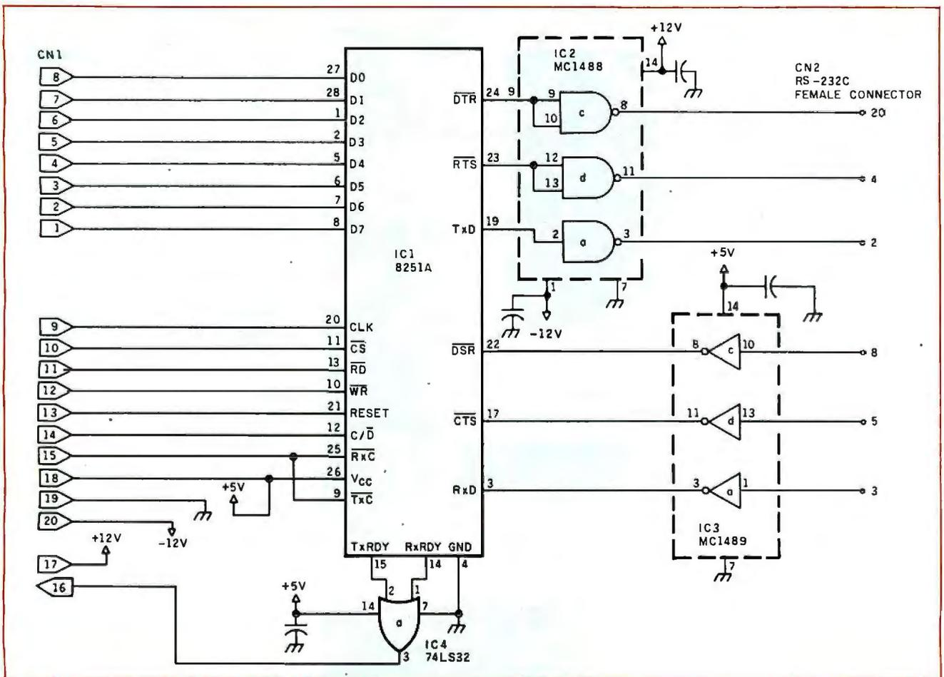
Figure 1: The serial-card schematic for the Sanyo MBC 550.
