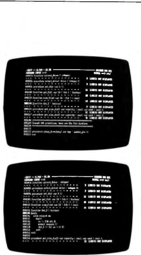
Photo A: With the SPFeditor's show/exclude feature, you can compress text display to show just vital function and procedure declarations (top), then expand it as needed to allow work on a particular module (bottom).
