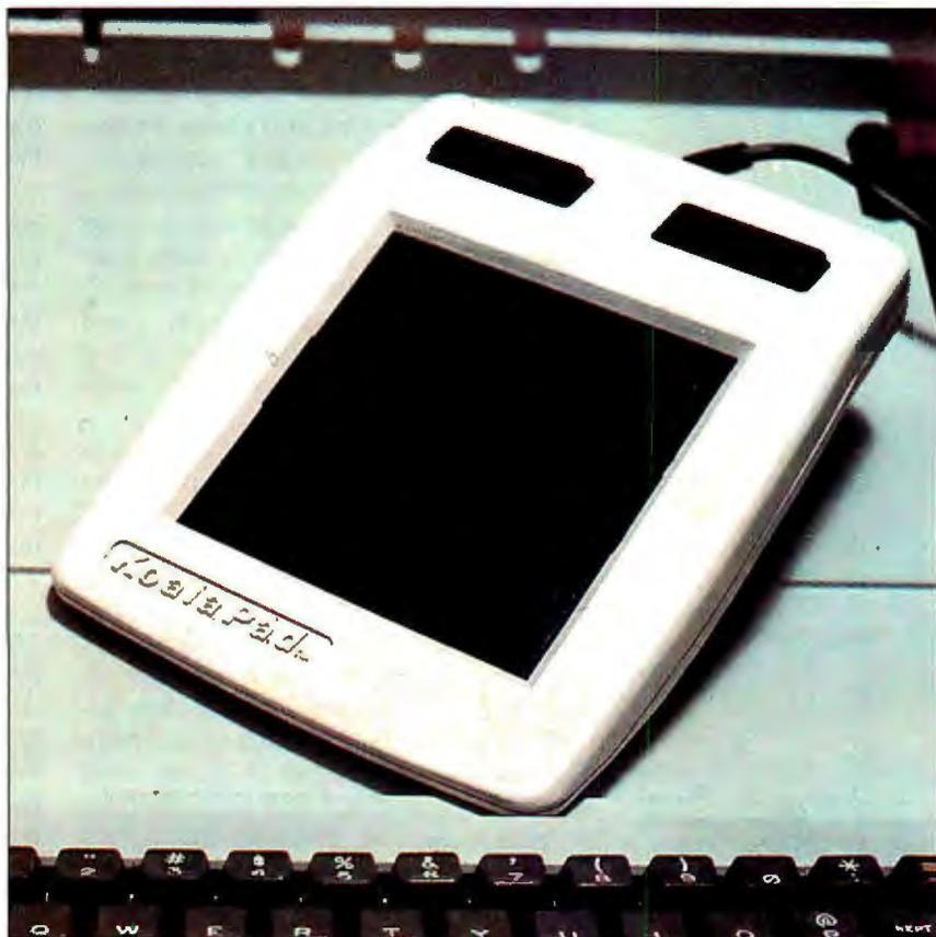
Photo 1: The KoalaPad provides a method for entry of data or for making selections from the screen using touch rather than the keyboard.
