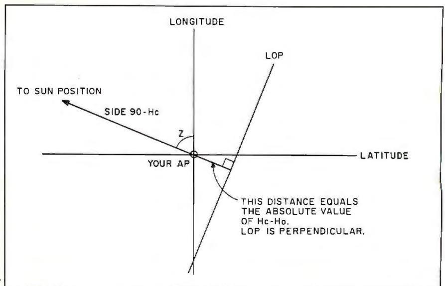
Figure D: Your assumed longitude and latitude form a coordinate system that contains the lower right corner of the triangle in figure B. The corner is formed by  $90 - H_c$  and your longitude. The LOP is a line drawn perpendicular to the radius of length  $90 - H_o$ . This drawing is hypothetical in that it assumes  $90 - H_o$  is greater than  $90 - H_c$ .
