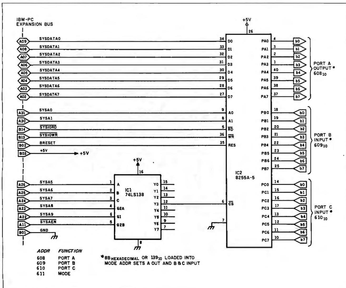
Figure 8: Parallel port for the IBM PC.
