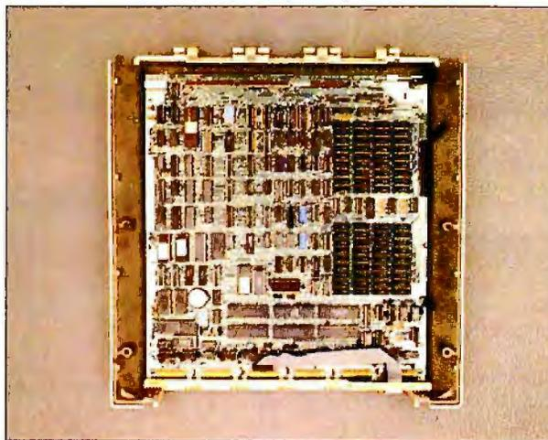
The upper board (with disk drives) attaches at the hinges along the top of the board. The units swing apart for access.
