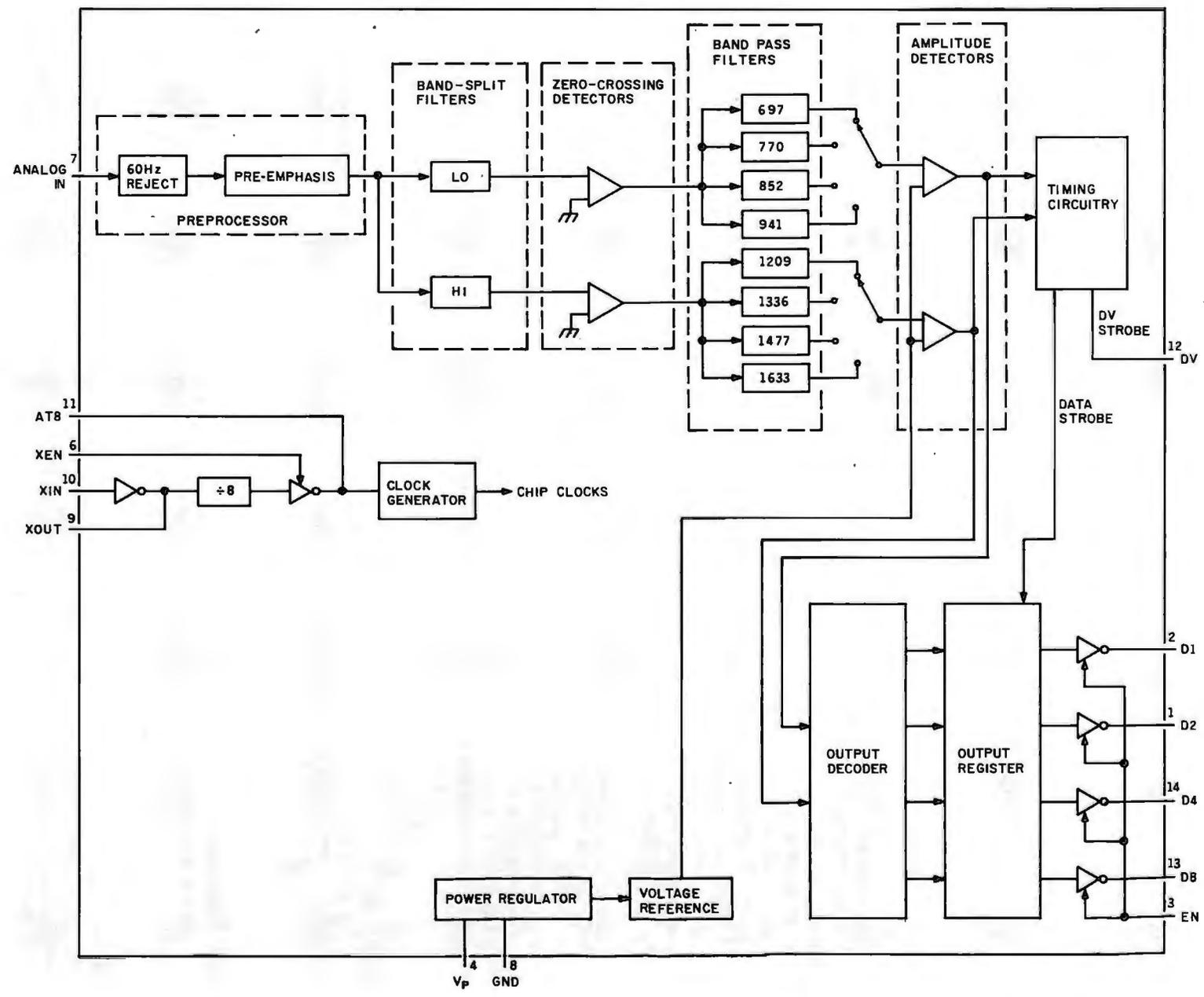
Figure 4: The Circuit Cellar DTMF decoder board.
