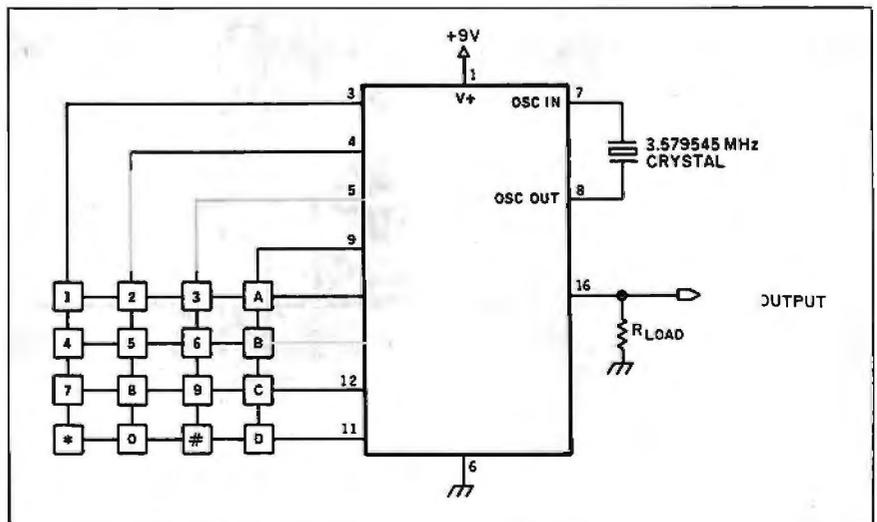
Figure 2: Schematic diagram of a DTMF-encoding circuit.
