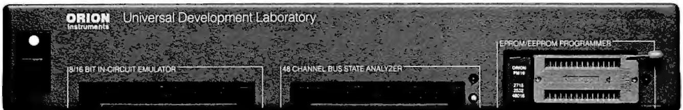
Up to 128K bytes of EMULATION ROM (8K standard) allows you to make program patches instantly. Since the target ROM socket connects data and address lines to both the analyzer and the emulator, no expensive adaptors or personality modules are needed.
