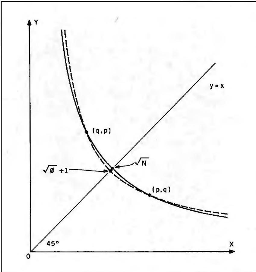
Figure 1: Graphic representation of equations (1) and (2). The solid curve is  $pq=N$ , and the dashed curve is  $(p-1)(q-1)=\phi$ . Because values of  $N$  worth factoring are not perfect squares, the hyperbolas will not intersect at the 45-degree line. Because of symmetry, it doesn't matter which factor we call  $p$  and which we call  $q$ .
