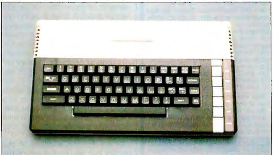
Photo 2: The keyboard of the 800XL. Note the better placement of the inverse-video key in the lower right corner.
