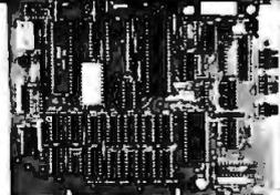
The Ampro Little Board is a single board Z-80A microcomputer with on board 512K disk controller, 64K/bytes of memory two serial ports along with a Centronics parallel printer port. This computer is supplied with enhanced CP/M 2.2 with well documented user manual. APO-LB1A
