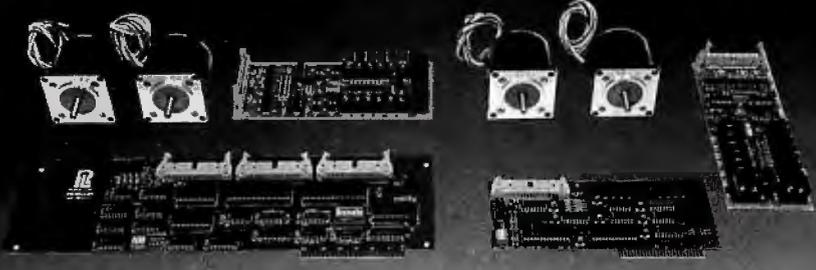
**Complete 2 axis systems using 2 size 23 stepper motors with R2D23 dual-axis driver; cable & powerful system software, expandable to 4 axis.**
