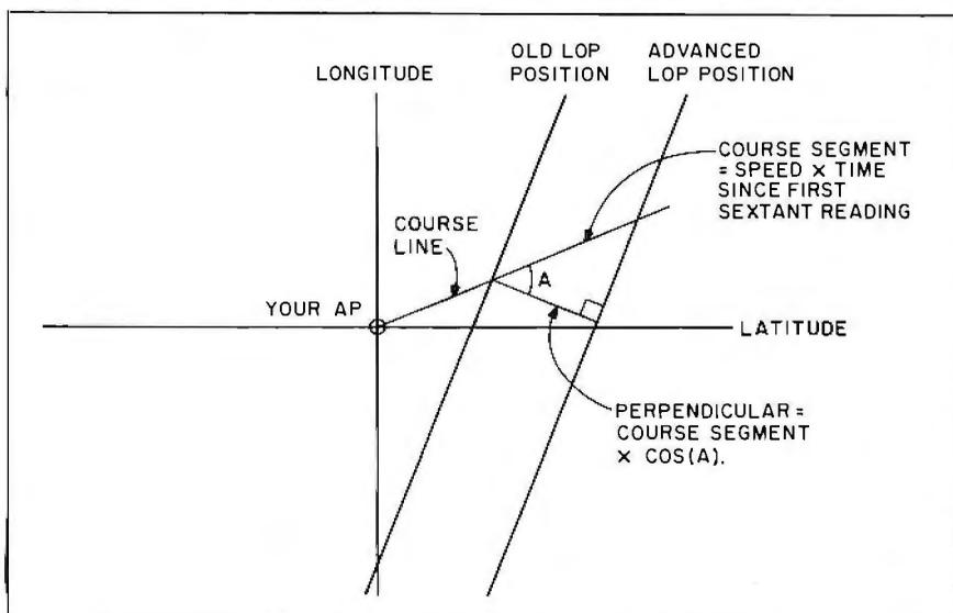
Figure E: Advancing or retiring the LOP is done by moving the line along a perpendicular to itself, a distance equal to the course segment  $\times \cos(a)$ . The course segment equals your speed multiplied by the time elapsed since the last sextant reading.
