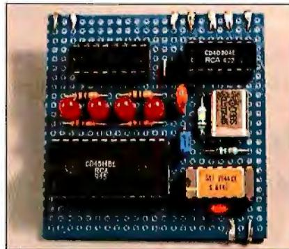
Photo 1: Prototype of the DTMF receiver board.
