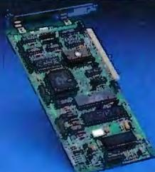
AT compatible disk controller handles 2 floppies, 2 Winchester.
