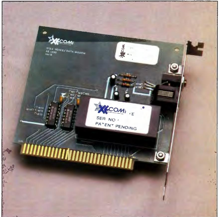
Photo 2: The Xecom IBM PC MOSART evaluation board.
