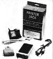
The Printer Jack™ is a device that will enable you to use the Apple IIc, which is not equipped with a parallel port, with any standard parallel printer. The Printer Jack can also be used with other computers with an optional cable. The Printer Jack set, Model A1250 includes: a CPU unit (the big box), a 9V power supply and a 5 pin to a 25 pin cable.
