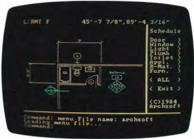
**Photo 4:** An architectural drawing using Archsoft's AE/CADD Master Template displayed using the standard IBM graphics card with 4 simultaneous colors at 320- by 200-pixel resolution.
