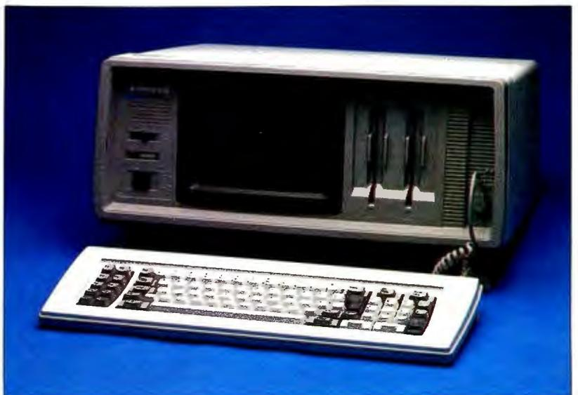
Photo 1: The Sanyo MBC-775 with built-in color monitor, keyboard, and two floppy-disk drives.
