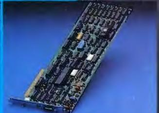
High res color and monochrome video controllers are fully interfaced with system.
