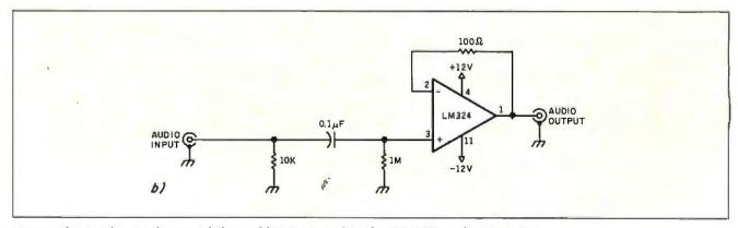
Figure 7b: A schematic diagram of the amplifier circuit used in the AVMUX's audio-output stage.
