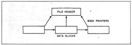
Figure 4: A file header can be reconstructed by reading pointers in the data blocks.
