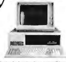
This standard system is as compatible with IBM as it can be. Featuring a 4-layer motherboard, 8-slot expansion, up to 640K memory on the motherboard, and the 6.67 MHz **TURBO** mode. Also included: DOS 3.1, keyboard, 19.5 watt power supply, TTL 720 x 348 resolution video card, green or amber monitor, serial & parallel ports, Real Time Clock and software.
