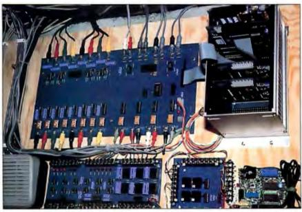
Photo 2: The finished AVMUX joins the HCS in the Circuit Cellar storage area. The card cage to the right contains the BCC-52, a Term-Mite video-display board, and a couple of analog-to-digital converter boards.
