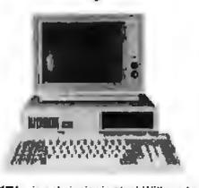
The **XT jr.** is only junior in size! With up to 640K memory on the motherboard and four expansion slots, this stand-alone system is also great for workstations in a networking environment. It can be upgraded to the **TURBO** two speed motherboard and you can also add up to 2 serial & 2 parallel ports or any IBM compatible expansion card. A perfect word processing/data entry system.
