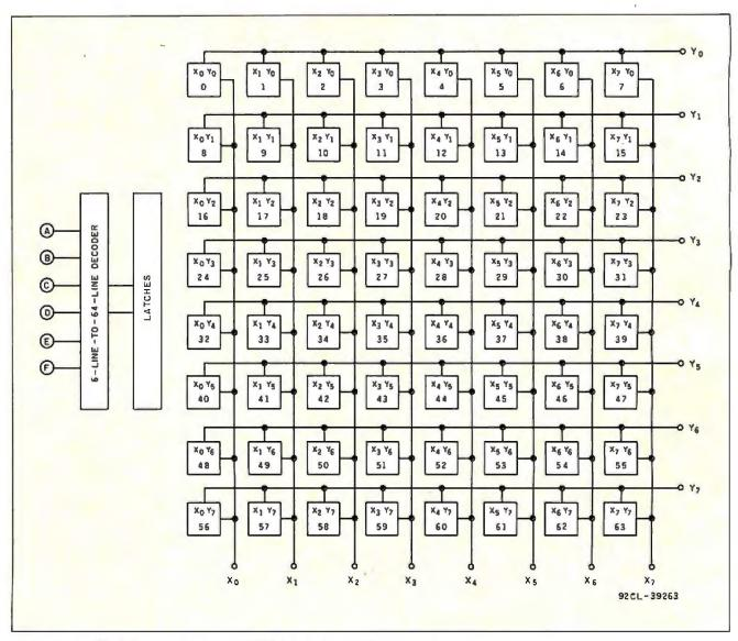
Figure 5a: A block diagram of the 74HC22106 8 by 8 crosspoint-switch 1C.
