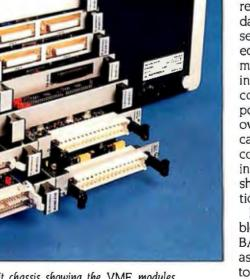
Photo 1: The rear view of the control-unit chassis showing the VME modules.
