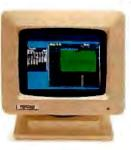
HX-9/9E. Nine inch, high resolution RGB monitor non-interlaced -.28mm dot pitch tube -9E compatible with IBM Enhanced Graphics Adapter -Nonglare screen -Green/amber switch -Apple/IBM colors - Etched dark glass screen -\$650/\$750 (9E)
