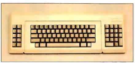
Photo 2: The MacCharlie function keys and numeric keypad attach to the Macintosh keuboard.
