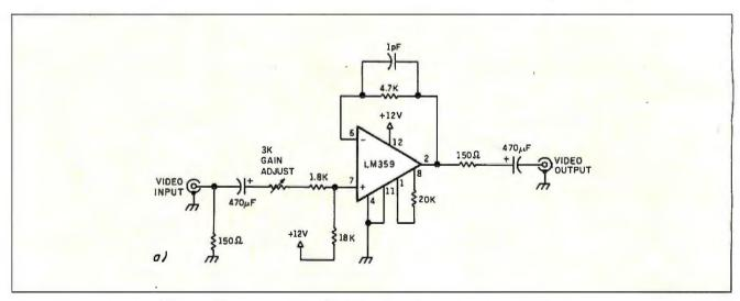
Figure 7a: A schematic of the amplifier circuit used in the AVMUX's video-output stage.
