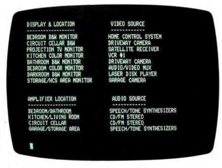
Photo 3: Using the BCC-52 and a video-display controller, a display of the AVMUX's configuration by location and source is easier to read than LEDs.
