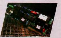
AppleMate 1200 Modem - A Hayes<sup>™</sup> compatible internal modem card designed for the Apple " II, II+, Ile with intelligent features and built-in diagnostics.
