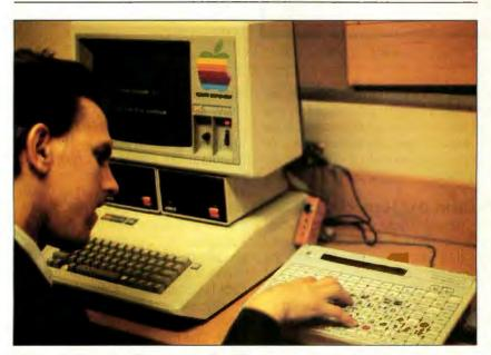
Photo C: Tony Miralles using Touch Talker. In this case the keyboard is not being used to generate speech; it interfaces with the computer to lower the number of keystrokes required to enter information. (Photo by Robin Schwartzmiller.)
