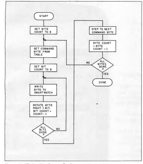
Figure 14: The SmafTime firmware flowchart—a routine to write a command string or data to the SmartWatch.
