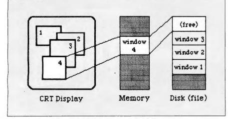
Figure 3: If you run out of RAM for storing window buffers, you can save some of those buffers to disk.
