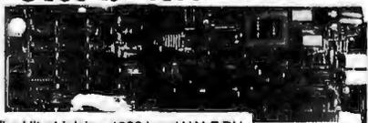
The UltraLink is a 1200 baud HALF DUPLEX bell 202 compatible internal modem card for the IBM/PC. This unit operates full duplex at 300 baud.
