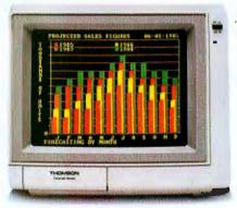
Model CM 31311SI. 12\*diagonal, 31mm dot pitch RGBI color monitor with text switch and non-glare tinted screen.
