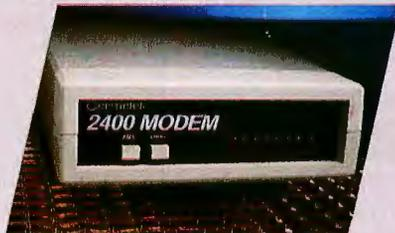
2400 Modem - A Hayes™ compatible 2400 bps modem with intelligent features and built-in diagnostics. MNP error control is available on the 2400 EP Modem.
