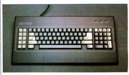
Photo 1: The Kaypro 286i keyboard uses the IBM PC AT layout.
