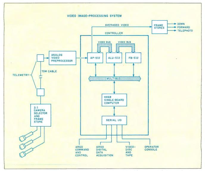
Figure 3: The video image-processing system on the Argo and Knorr. The cameras and frame stores on the Argo are shown on the left and the processing and display hardware on the Knorr to the right.
