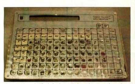
Photo B: The Touch Talker keyboard. Note the keyguard to prevent those with motor-coordination difficulties from activating the wrong key. This device also requires a pressure of 4½ ounces to initiate a keystroke, enabling those who have problems controlling fine movements to select only the key they really want. (Photo by Robin Schwartzmiller.)
