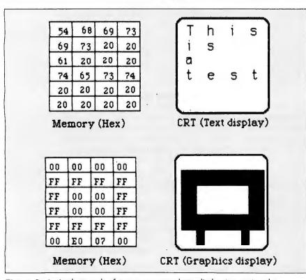
Figure 2: A simple example of a memory-mapped text display (top row) and a memory-mapped graphics display (bottom row).
