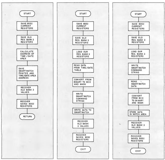
Figure 11: The SmarTime firmware flowchart—the initialization routine.
