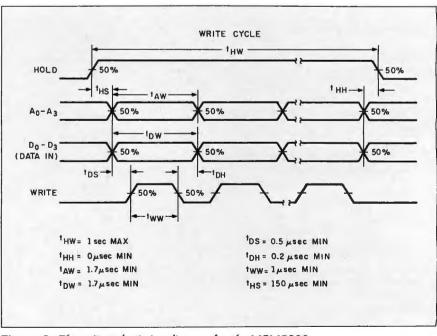
Figure 3: The write-cycle timing diagram for the MSM5832.
