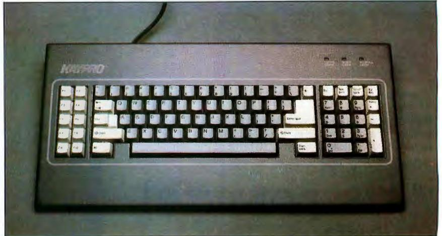
Photo 1: The Kaypro 286i keyboard uses the IBM PC AT layout.
