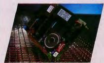
1200 SPC Modem - The 1200 SPC Modem provides Hayes1st compatibility - designed for the short slot in the IBM \*\* PC/XT/AT or clone.
