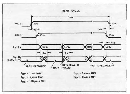
Figure 2: The read-cycle timing diagram for the MSM5832.
