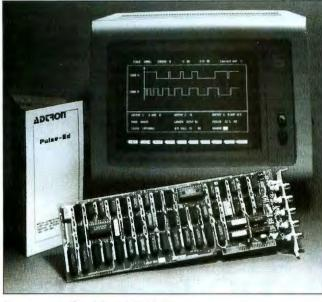
Data-generator board from Adtron's system.
