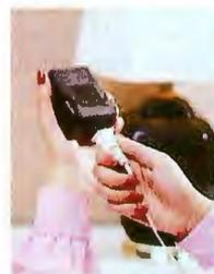
and then plug the Module into an outlet. The Interface can control up to 256 Modules throughout your home and won't interfere with normal use of lights and appliances.
