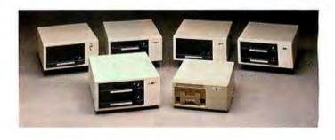
\*The Bernoulli Box for Macintosh is available in a 5-megabyte single-drive version and a 20- megabyte dual-drive version for AppleTalk."
