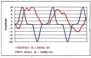
Figure C: A graph of displacement (X(2)) and driving force (FNX(7)) versus time for a system with Coulomb damping and nonlinear spring force.
