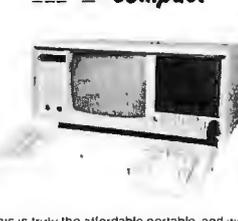
This is truly the affordable portable, and will build it to your specifications. Need a 20 meg hard disk and 20 meg tape with E-DK memory in your portable? No problem! The **XPC Compact** comes standard with a 9" amber TTL monitor, 135 watt P.S., 256K memory, two 360K drives, Real Time Clock, Calendar w/ battery Back-up, serial and parallel ports, and our **TURBO** Motherboard.
