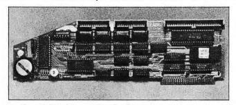
Xcalibur's XAD5 data-acquisition board.
