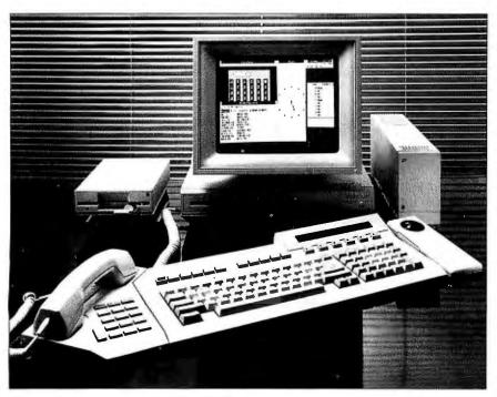
Photo I: The new Apricot XEN 80286-based business microcomputer. It is shown with a 360K-byte 5½-inch floppy-disk unit and an expansion box, which can house up to two IBM expansion cards; these units provide some compatibility with the IBM PC and the PC AT. The optional combination trackball/mouse and telephone are also shown. The XEN is seen running Microsoft Windows, which is its standard operating environment.
