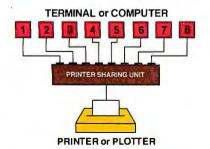
Our 4 or 8 port Printer Sharing Units work automatically. No cable switching or knobs to turn. Software changes are usually unnecessary since they use standard Ready/Busy or XON/XOFF handshaking.
