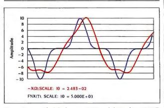
Figure B: A graph of displacement (X(2)) and driving force (FNX(T)) versus time for the startup of the system with Coulomb damping.
