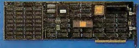
The **TurboACCEL-286** features a high-speed, 8MHz, 80286 processor, 512Kbytes of RAM (expandable to 1Mbytes), a switch for 8088 operation, and facilities for an 80287 math co-processor. It occupies one expansion slot, is completely compatible with most PCs and is software transparent. End your search for AT performance. Order the **TurboACCEL-286** today! Call or write:
