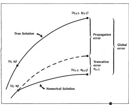
Figure 1: An illustration of errors in a numerical solution.
