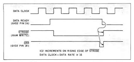
Figure 2: RAM load timing.
