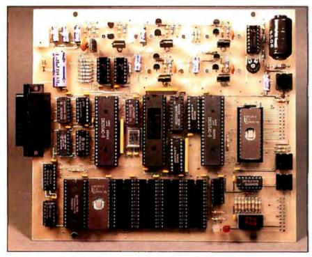
**Photo I:** Finished printed circuit prototype of the serial EPROM programmer. The digital section and memory buffer are at the bottom center. The analogvoltage-level switching section is at the top center.
