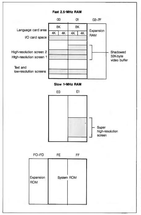
Figure 2: The Apple 11 GS memory map. Shaded areas indicate shadowed memory, where any write operation is duplicated to the corresponding location in banks EO and E1 hexadecimal. The super hi-res screen does not need shadowing, but it is included as a convenience to Applesoft and 6502 programmers, who can only work with banks OO and O1. Memory areas are not drawn to scale.
