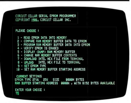
Photo 2: Typical menu display presented when operating the serial EPROM programmer through a serial terminal or computer running in terminal-emulation mode.
