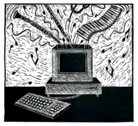
microcomputers is sort of a trick. For example, when a microcomputer makes a clarinet sound, it actually produces a square wave. The result sounds like a clarinet because a clarinet's waveform is close to a square wave. But the waveform of a piano or a flute is more complex and can't be created easily with most microcomputers.
