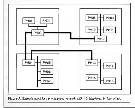
1. If two phones are connected to the same local line (e.g., PH01 and PH02), the call will be routed through directly. One local call is charged.
