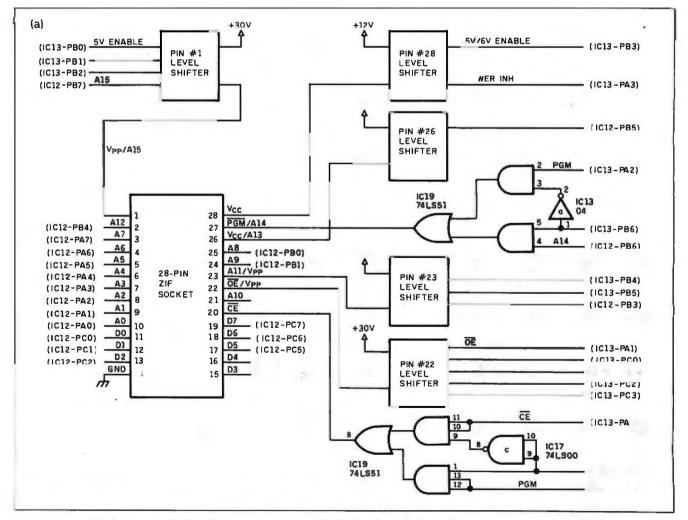
**Figure 3**: (a) Block diagram showing the connections to the ZIF socket. Note the level-shifter circuitry connections for those pins that require programming voltages or that differ across EPROM types.
