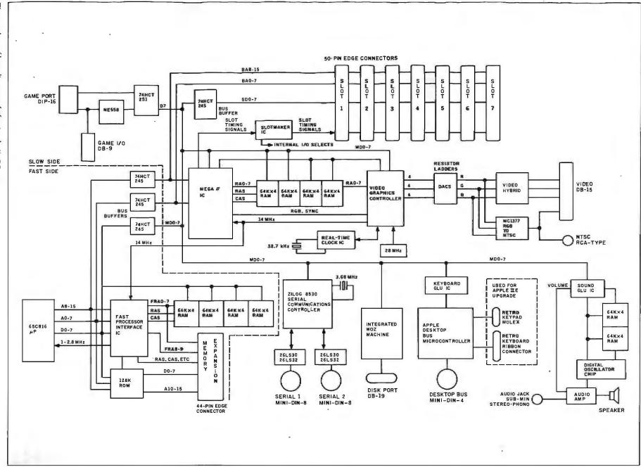
00 or 01), then slow itself down to I MHz and write to the location and its equivalent in bank E0 or E1 hexadecimal. In many locations (video display memory, for example) read operations from the same location have no timing constraints and can proceed at the higher 2.5-MHz speed. Because other locations (like the ones associated with peripheral card I/O) must always be written to and read from at I MHz, the speedup of Apple
