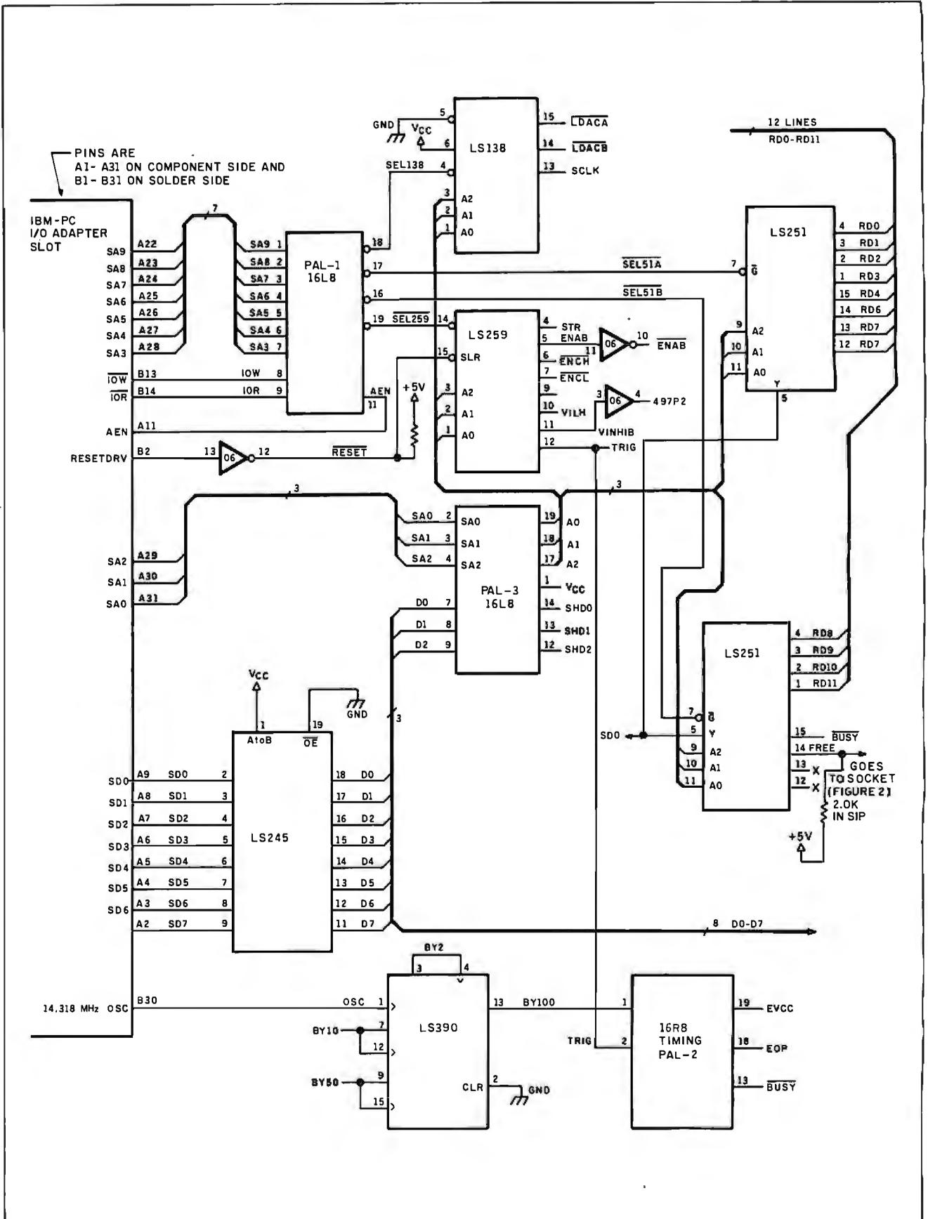
Figure 6: Schematic of the IBM PC interface to ZAP-A-PAL.
