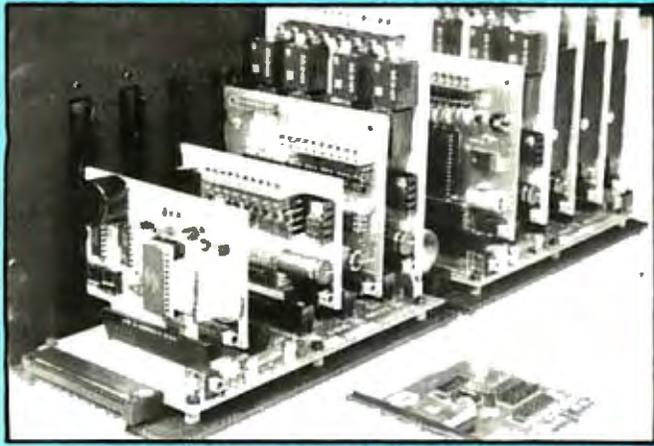
An A-BUS system with two Motherboards
