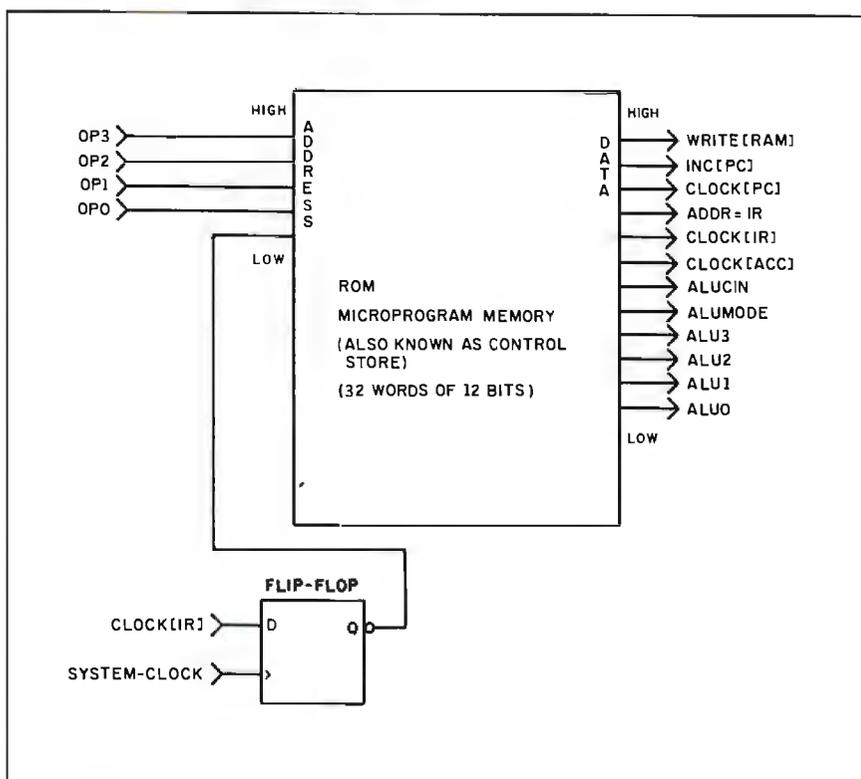
Figure 6: Microcoded controller schematic.
