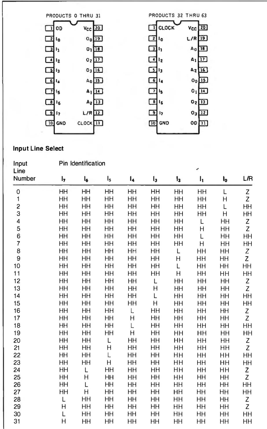
Figure 1: Voltage configuration to program a 20-pin PAL. Adapted from The PAL
