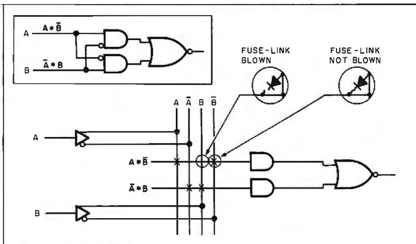
**Figure D:** The PAL device implementation of the function  $\text{Output} = A \cdot B + \bar{A} \cdot \bar{B}$ . The standard combinational logic diagram of the function  $\text{Output} = A \cdot B + \bar{A} \cdot \bar{B}$  is shown in the inset to figure D above.
