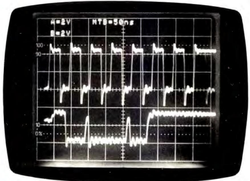
**Photo 1:** The AS output of the DPORT20 PAL. The top trace is the Q0 input; the bottom trace is the AS output. Notice the 9-ns-wide glitches in the AS output between Q0 counts 4 and 5 and counts 8 and 9.
