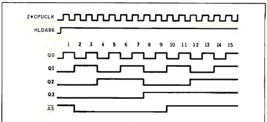
Figure 3: Timing diagrams for the DPORT20.
