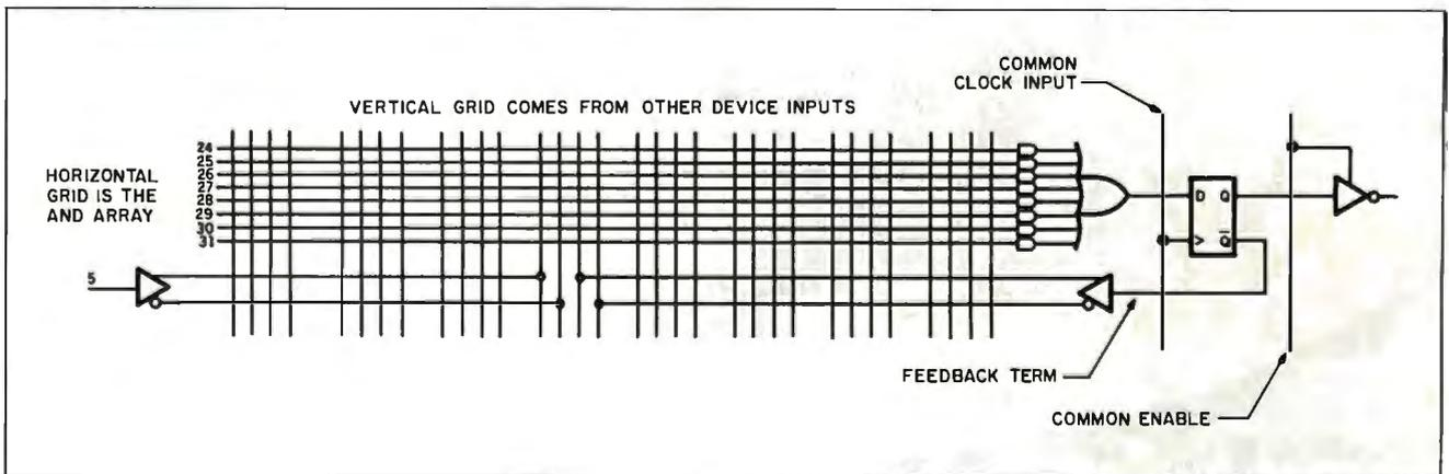
Figure 7: Clocked logic cell from a 16R4 PAL.
