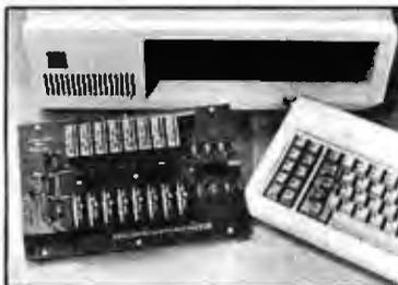
The boards allow you to Control/Monitor high voltage AC/DC power lines with your IBM-PC/XT/AT or compatible while providing optical isolation.
