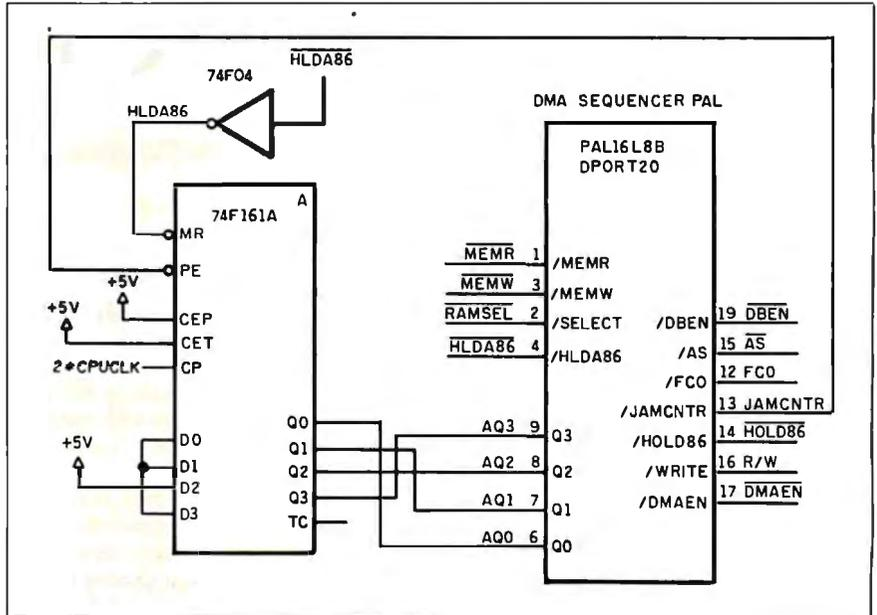
Figure 2: The DPORT20 portion of the DSI-020 schematic.
