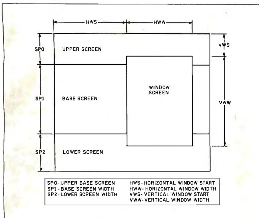
**Figure 1:** Besides establishing basic CRT timing, the timing control registers partition the screen into the upper, base, lower, and window portions. The upper, lower, and base screens are all background screens that are overlapped by the foreground window. The vertical specifications (SP0, SP1, SP2, VWS, and VWW) are in units of rasters, while horizontal specifications (HWS, HWW) are in units of display cycles. Usually, only the base (covering the entire CRT screen) need be defined.
