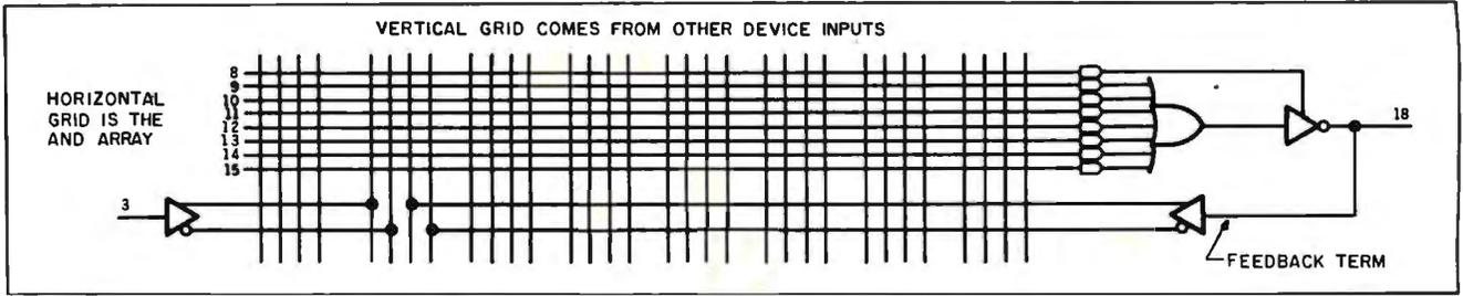
Figure 1: A logic cell from a 16L8 PAL. Notice the inverter between the OR gate and the output.
