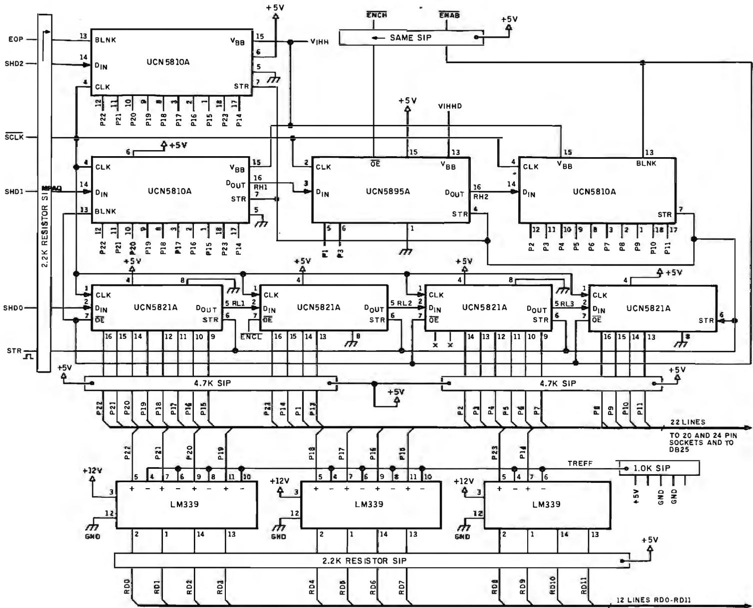
Figure 3: Schematic for the pin drivers and verify circuits.
