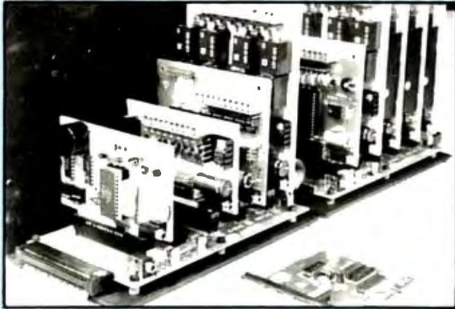
An A-BUS system with two Motherboards
