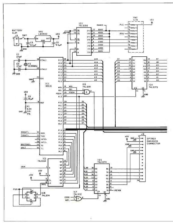
Figure 1: Master Controller schematic diagram.
