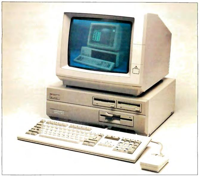
**Photo 1:** The Amiga A2000 computer. The A2000 comes with 1 megabyte of memory and one 3<sup>1</sup>/<sub>2</sub>-inch floppy disk drive. You can also substitute internal hard disks for the second (left) 3<sup>1</sup>/<sub>2</sub>-inch and the 5<sup>1</sup>/<sub>4</sub>-inch drives that are installed in this machine. The image of the IBM PC shown on the screen was captured using NewTek's Digi-View software.
