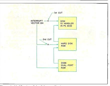
**Figure 6:** Modification of the disk controller interrupt vector to support a hard disk drive. This sequence of modifications allows you to use any type of PC hard disk with the A2088 board.
