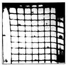
Another problem with the cameras was photometric nonlinearity. When aimed at a uniform white or gray field, the cameras displayed a brightness in the center and a darkness around the edge caused by a
