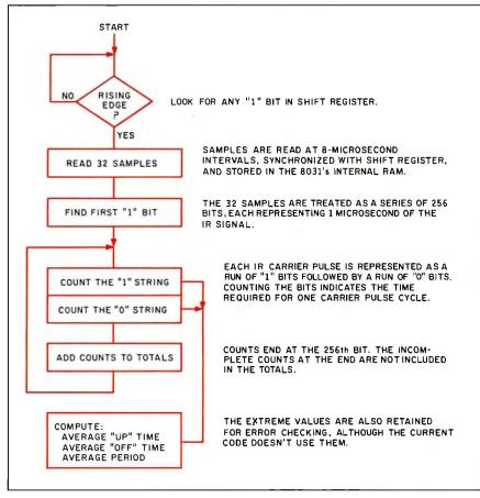
Figure 2: Carrier-frequency measurement flowchart.
