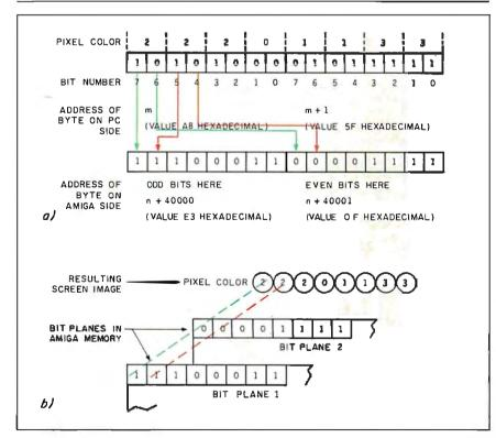
**Figure 4:** Graphics access of the dual-port RAM. Two adjacent bits on the PC side make up a pixel, but these bits must be in different bit planes to recreate the same pixel on the Amiga side. Figure 4a shows how 2 bytes on the PC side (top) are mapped into the Amiga side (bottom). Figure 4b shows how the 2 bytes on the Amiga side are placed in different bit planes to recreate the pixel pattern created on the PC side.
