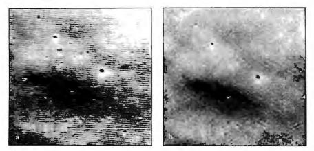
**Photo 2:** To remove oscillation noise from Ranger images, JPL researchers isolated an area of the image that showed the noise pattern (a) and used that pattern as a filter to subtract the pattern from the rest of the image (b).
