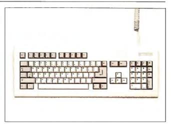
**Photo 3:** The A2000 keyboard. All the keys on the keypad are labeled on their front face with the IBM PC-related functions associated with them.
