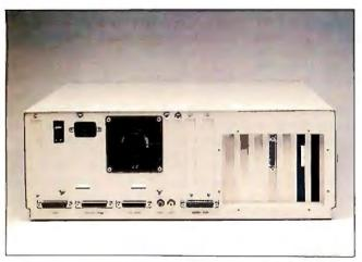
**Photo 2:** The A2000 back panel. Notice the cutouts for outputs from peripheral cards.
