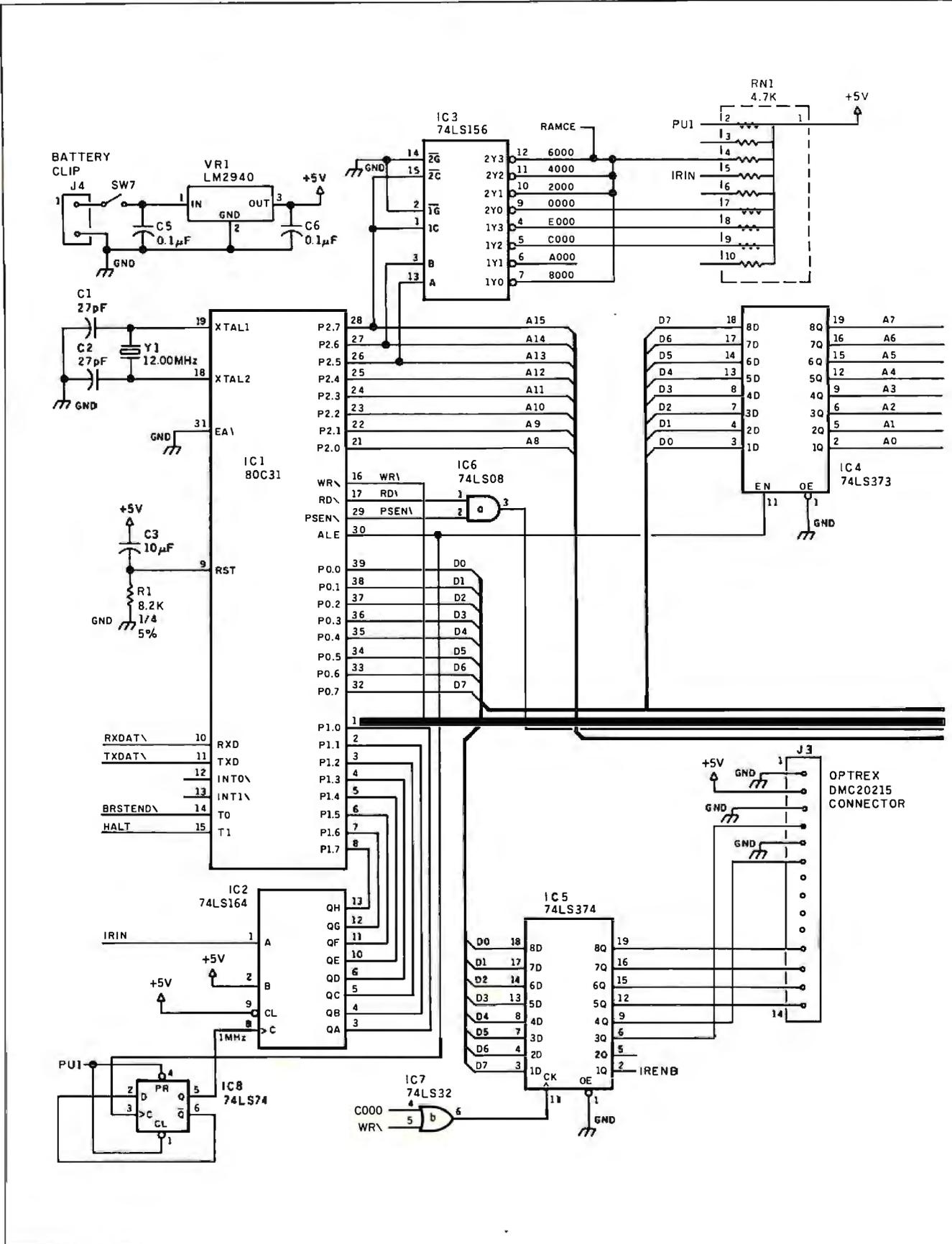
Figure 1: Master Controller schematic diagram.
