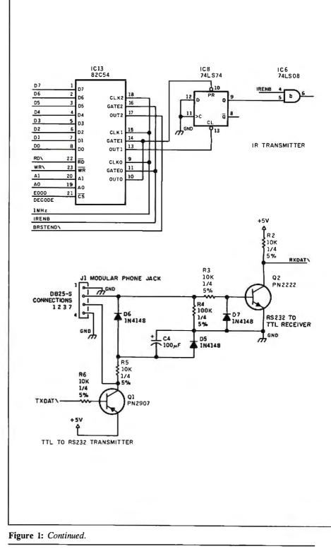
Controller software uses all three of them, as well as a timer inside the 8031, during the IR playback.
