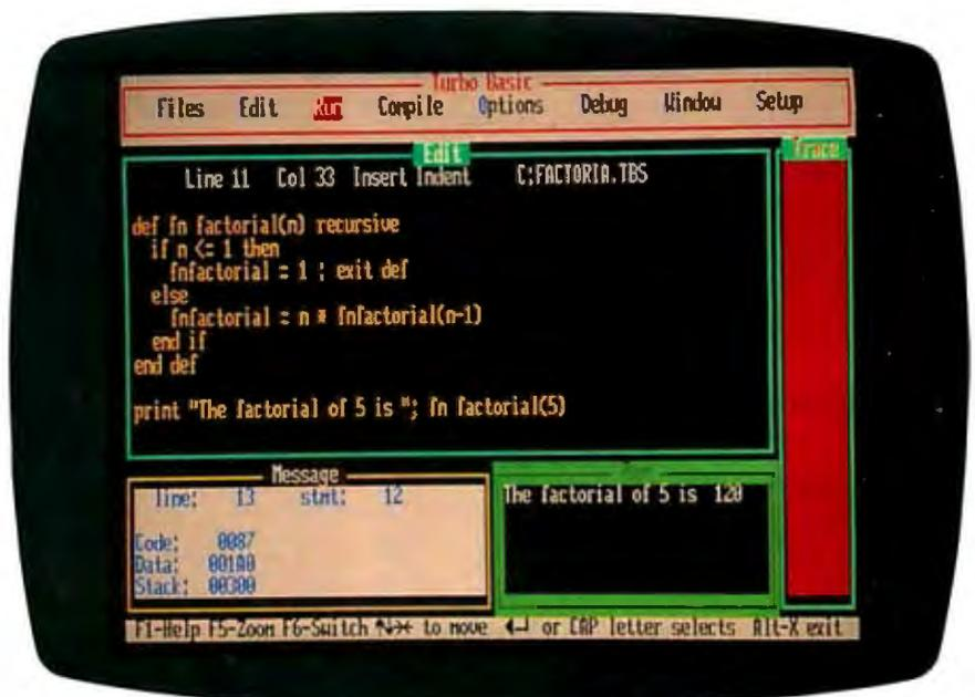
Photo 2: Turbo BASIC screen showing a recursive factorial program.
