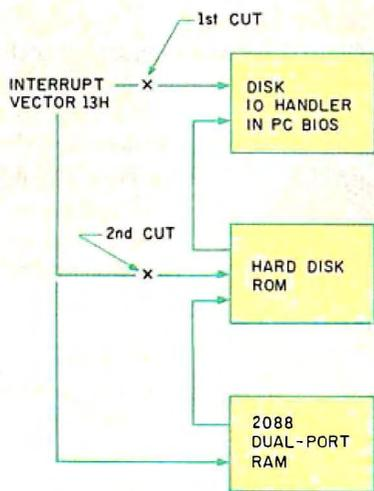
**Figure 6:** Modification of the disk controller interrupt vector to support a hard disk drive. This sequence of modifications allows you to use any type of PC hard disk with the A2088 board.
