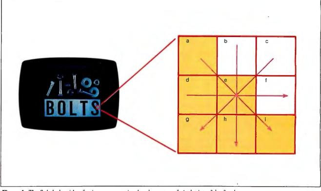
Figure 1: The Sobel algorithm for image processing breaks arrays of pixels into 3 by 3 subarrays.
