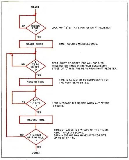
Figure 3: Signal-capture flowchart.
