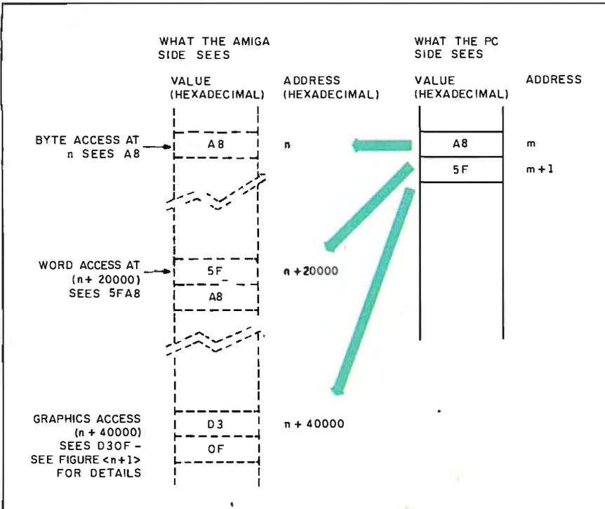
**Figure 3:** Three modes of access for the Amiga 2088 board's dual-port RAM. Though each memory location in the dual-port RAM has only one address on the PC-compatible side, it appears at three different locations in the Amiga's address space. The dual-port RAM maps the bits to the Amiga side in a different order based on the location accessed.
