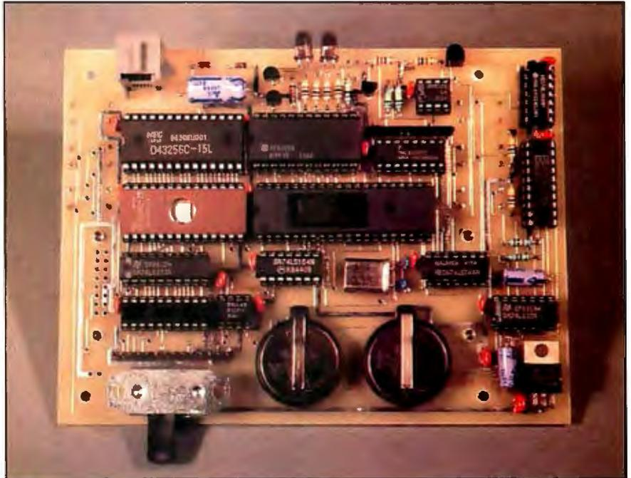
**Photo 2:** Component side of the Master Controller, showing the 2764 EPROM and 8031 CPU (center left and right). The backup batteries and Dallas Semiconductor DSI210 battery controller are in the bottom center and right.
