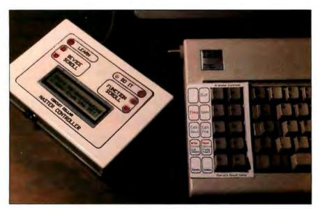
**Photo 4:** The Master Controller and the IBM PC keyboard showing the MASTER program function-key template.
