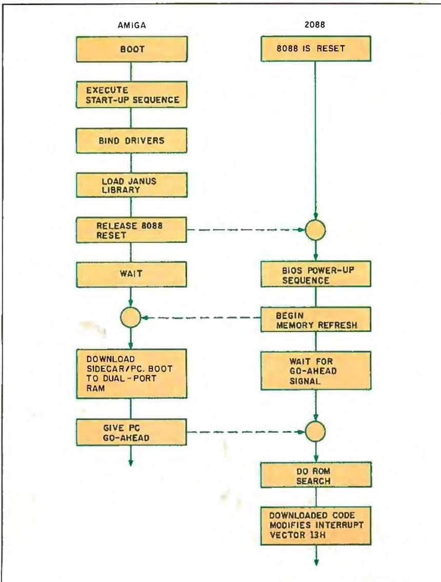
**Figure 5:** The sequence of events necessary to boot the A2088 board with the Amiga 2000.
