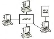
The PC Station is the only terminal of its kind with dual-host capability, which allows it to be connected to a mainframe host and an AT host simultaneously.
