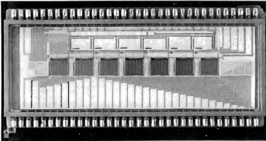
**Photo 7:** A hybrid carrier designed by Dr. Robert Nathan holds five VLSI chips and allows up to 35 simultaneous multiply/add operations to be performed on image data.
