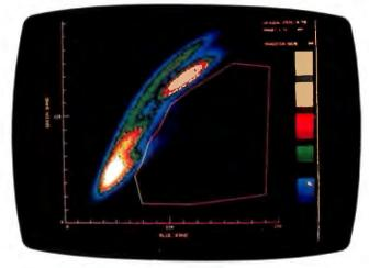
**Photo 12:** A bi-scatter plot of pixel values in the head-neck region. Pixels represented by combinations within the polygon are good candidates for data manipulation.
