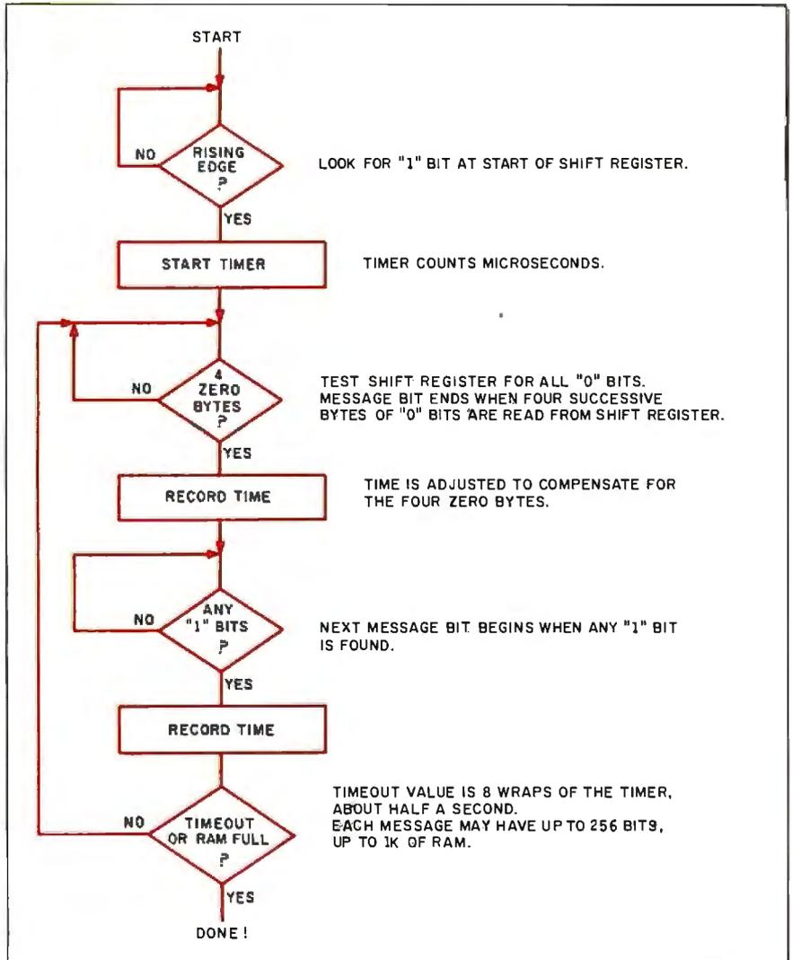
Figure 3: Signal-capture flowchart.
