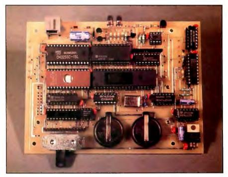
**Photo 2:** Component side of the Master Controller, showing the 2764 EPROM and 8031 CPU (center left and right). The backup batteries and Dallas Semiconductor DS1210 battery controller are in the bottom center and right.
