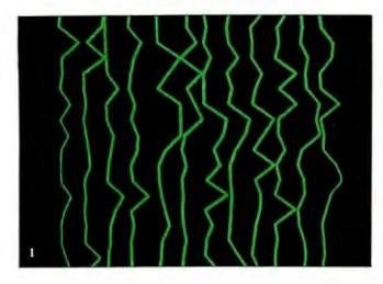
**Photo 1:** Unenhanced ultrasonic C-scan image from the east wall of the Palazzo Vecchio showing the inhomogeneous nature of the masonry structure.
