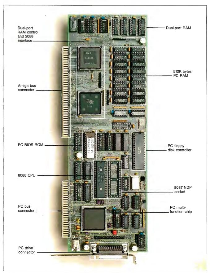
**Photo 5:** The A2088 PC emulator board. This board contains the 8088 processor, memory, ROM, and support chips of an IBM PC-compatible computer and correctly uses any PC peripheral cards connected in the PC slots.
