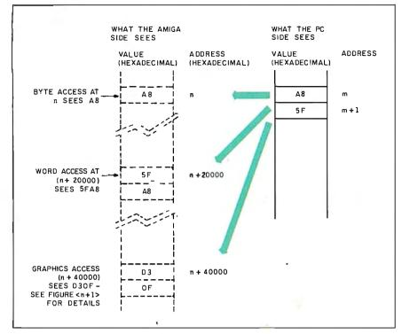
Figure 3: Three modes of access for the Amiga 2088 board's dual-port RAM. Though each memory location in the dual-port RAM has only one address on the PC-compatible side, it appears at three different locations in the Amiga's address space. The dual-port RAM maps the bits to the Amiga side in a different order based on the location accessed.
