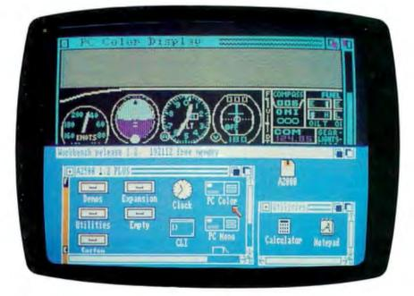
**Photo 6:** Running IBM PC software on the A2000. Here, the Amiga's desktop screen has been "pulled down" to reveal the PC color display screen. You can see Microsoft's Flight Simulator program running in the PC screen.
