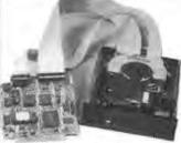
**PC Hard Disk** Systems with Drive, Controller & Cables
