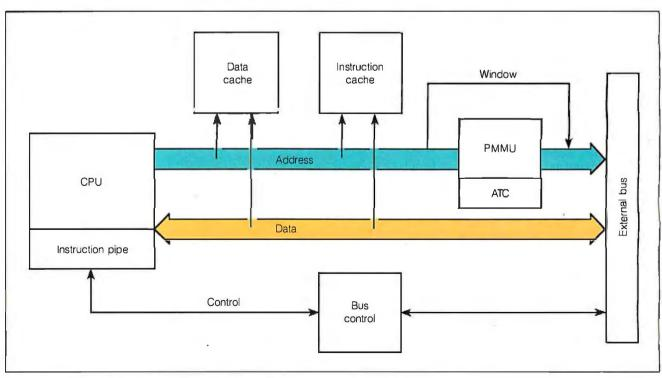
Figure 6: A functional block diagram of the MC68030 microprocessor.
