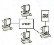
The PC Station is the only terminal of its kind with dual-host capability, which allows it to be connected to a mainframe host and an AT host simultaneously.
