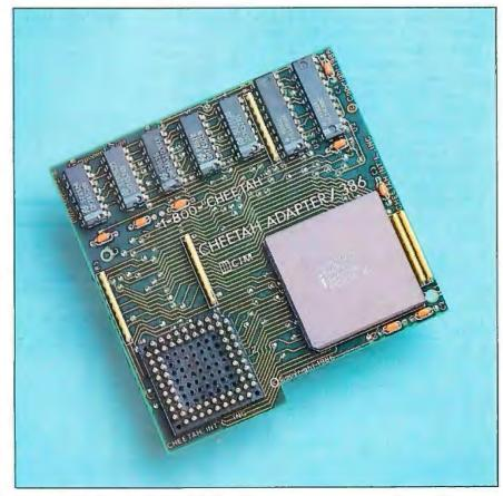
**Photo 1:** The Cheetah Adapter/386 board with pin grid array plug (lower left).
