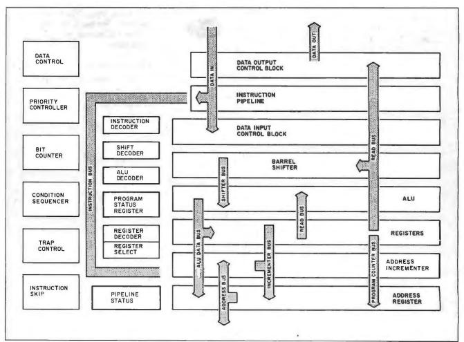
Figure 4: The ARM block-and-position diagram.
