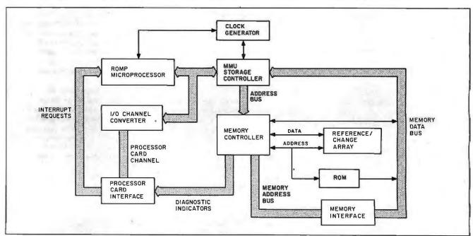
Figure 1: The IBM RT PC processor-board block diagram.
