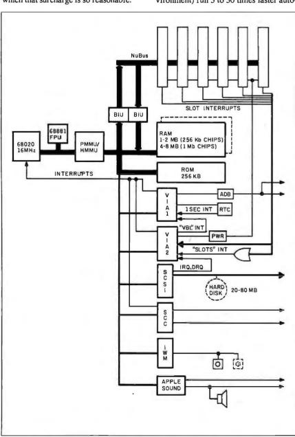
Figure 1: A block diagram of the Macintosh II. The dashed components are optional.
