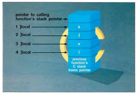
Figure 2: The C stack frame for the code fragment shown in listing 1.
