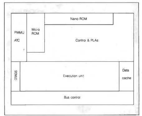
Figure 7: The location on the chip of the various MC68030 circuits.
