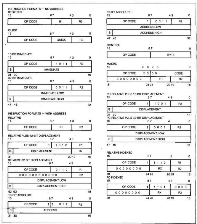
Figure 1: Clipper's balanced instruction set blends 101 RISC-like hard-wired streamlined instructions with 67 CISC-like macros.
