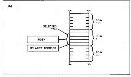
Figure 3: (a) Relative addressing provides a simple means for accessing any array item. (b) Relative indexing facilitates the more complex task of accessing items in two-dimensional arrays.
