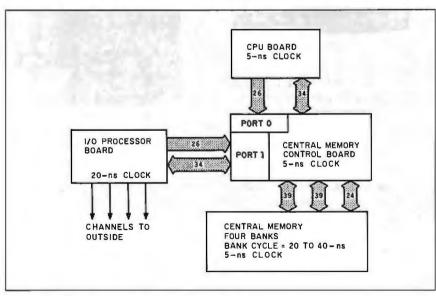
Figure 5: The TI/CDC GaAs RISC-system block diagram.
