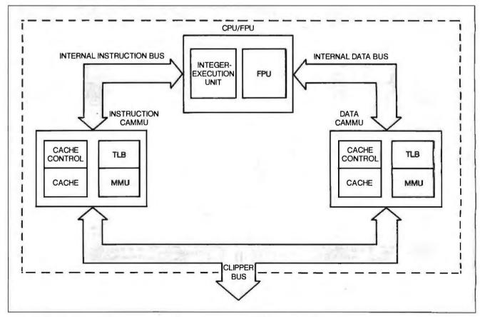
Figure 5: Twin high-bandwidth buses connect data and instruction CAMMUs to the CPU.
