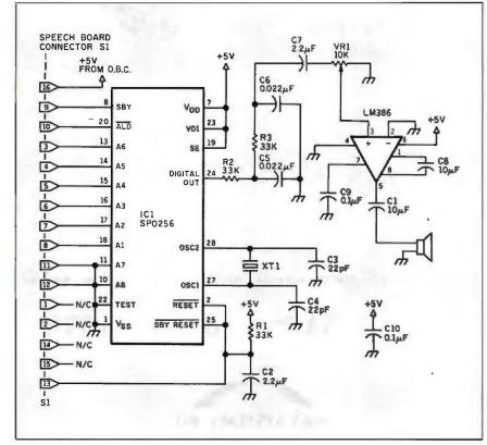
Figure 4: Schematic diagram of BERT's speech board.
