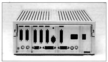
Photo 1: The back of the computer shows the wealth of built-in I/O. From left to right are the headphone jack, two serial ports, a joystick port, a disk drive port, the RGB and monochrome/composite video connectors, and the keyboard connector.
