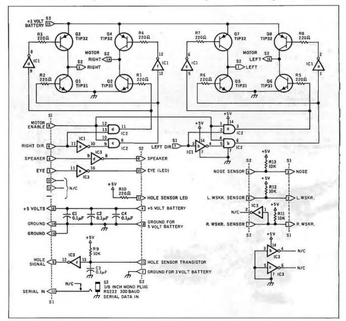
Figure 3: Schematic diagram of BERT's motor control board.
