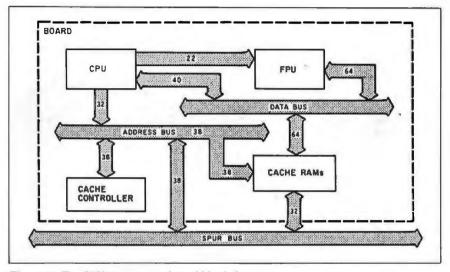
Figure 2: The SPUR processor-board block diagram.
