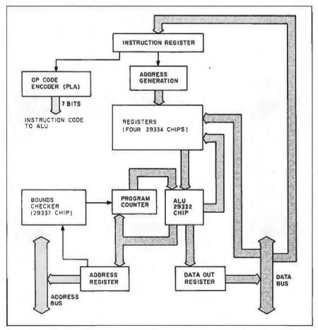
Figure 3: The AMD RISC-system block diagram.
