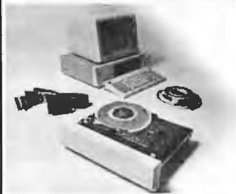
For information interchange, backup and archival storage, IBEX offers a 9-track, IBM format-compatible 1/2" magnetic tape subsystem for the IBM PC, featuring:
