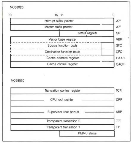
Figure 5: Additional MC68020/MC68030 supervisory model registers.
