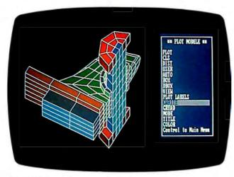
PCTRAN Plus helps create finite-element models.
