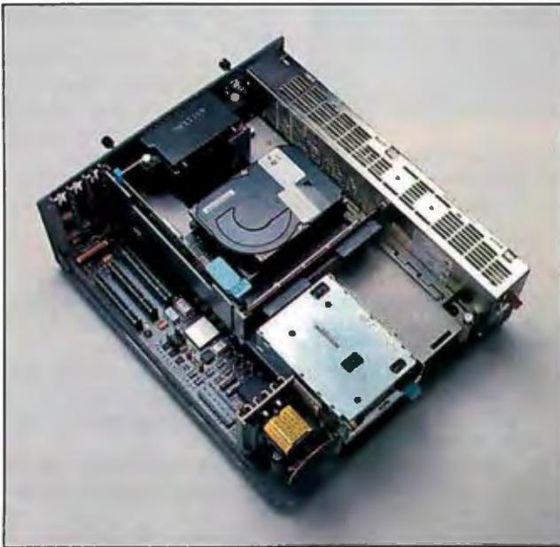
**Photo 1:** The Model 50 with its housing off. Notice how the hard disk (in the center of the machine) plugs directly into the controller board.
