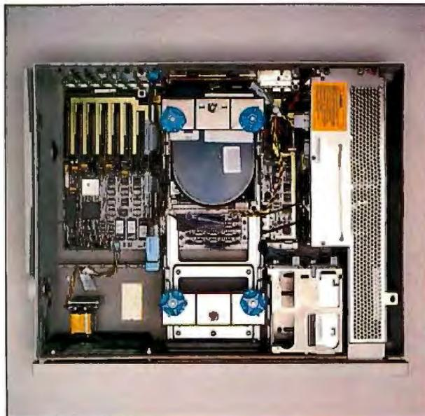
**Photo B:** The interior of the Model 60. "Up" in this photo is actually to the right, so the boards mounted in the Micro Channel slots (on the left) sit horizontally in the machine.
