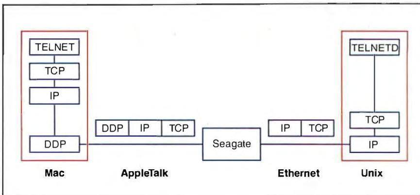
**Figure 1b:** *Exchanging ARPA packets through Seagate.*
