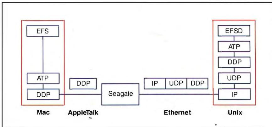
**Figure 1a:** *Exchanging AppleTalk data packets through Seagate.*
