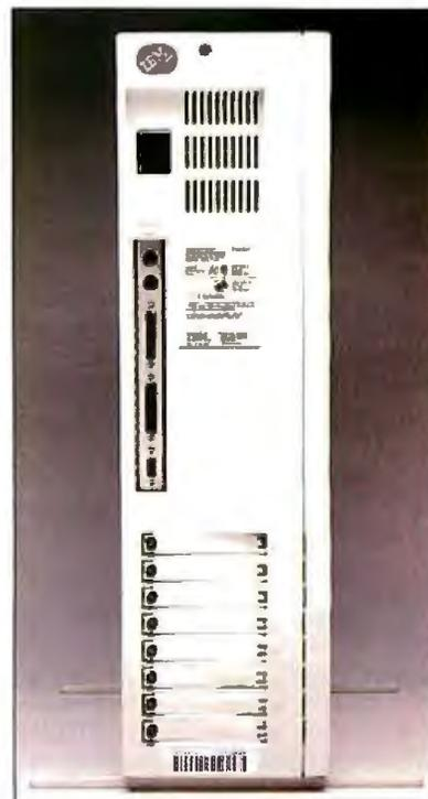
**Photo C:** The rear of the Model 60, showing the connectors for the keyboard, mouse, serial port, parallel port, and video monitor.
