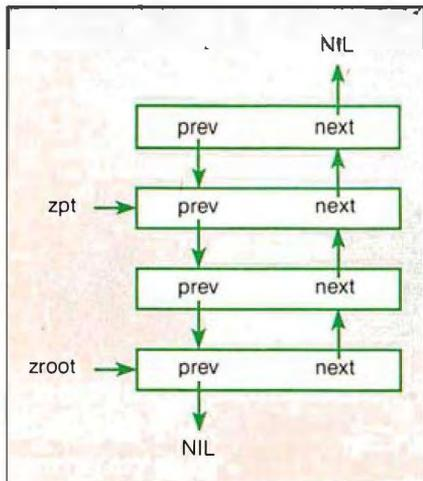
Figure 1: Typical stack structure.
