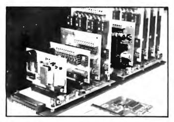
An A-BUS system with two Motherboards
