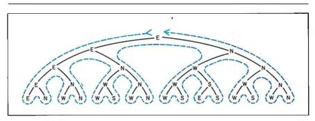
Figure 6: The broken arrow shows how the procedure in listing 1 draws the cells at the bottom of the diagram in the order that it encounters them.
