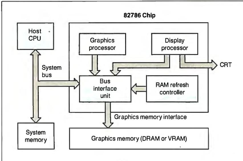
Figure 1: The 82786 graphics coprocessor architecture.
