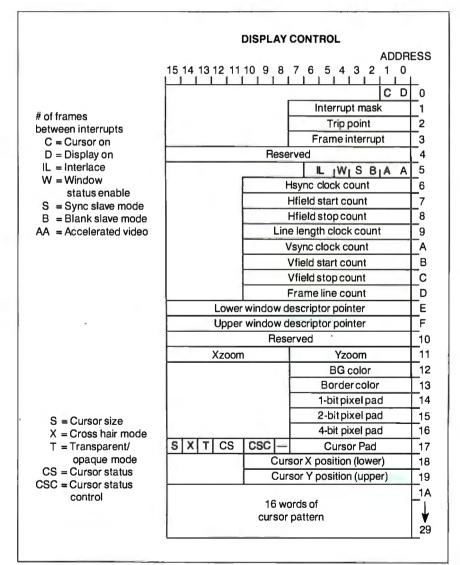
Figure 2: Graphics coprocessor display-control block.
