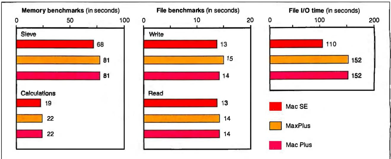
**Figure 1:** A comparison of the Mac SE against a Mac Plus and a Mac Plus-caliber machine. "MaxPlus" is a 512K-byte Macintosh with a 128K-byte ROM upgrade, MacMemory's 2-megabyte RAM expansion, and SuperMac Technology's SCSI port upgrade and DataFrame 20 20-megabyte SCSI hard disk drive. The Mac Plus tested was equipped with an Apple Hard Disk 20 20-megabyte hard disk drive connected
