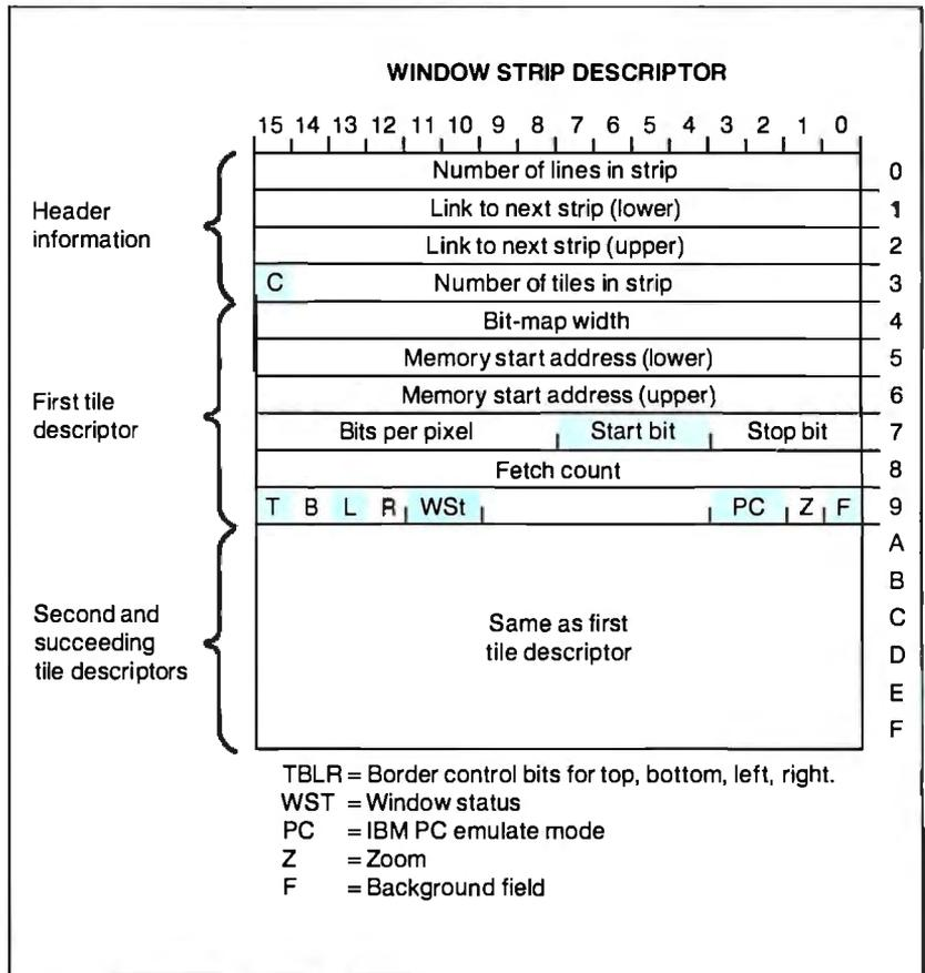
**Figure A:** Graphics coprocessor window-descriptor block.
