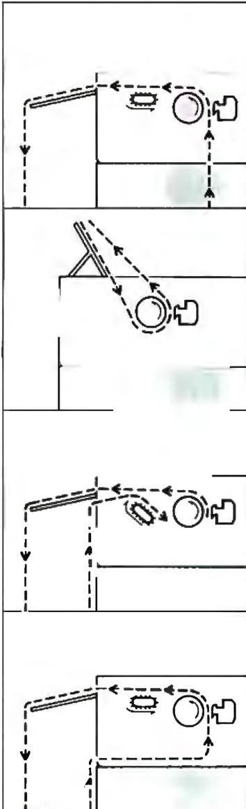
*To handle any kind of paper, numerous feed methods are offered, including bottom feed...*
