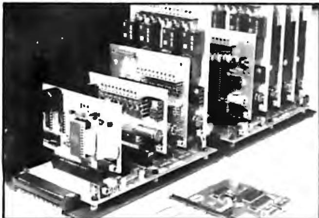
An A-BUS system with two Motherboards
