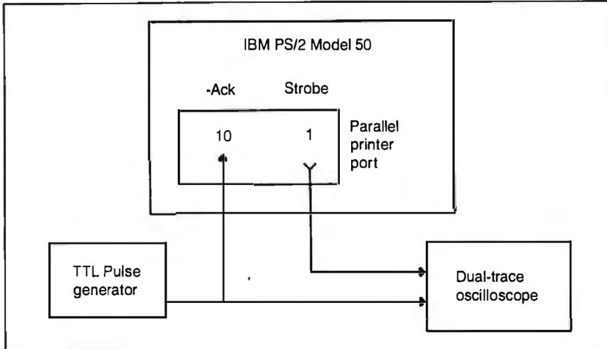
**Figure 2:** Our interrupt test hardware. We replaced the standard interrupt handler for the PS/2's parallel printer port with a specialized one. We measured the interrupt time delays by connecting a dual-trace oscilloscope to both the Ack line and an output-port bit controlled by the interrupt handler.
