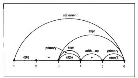
**Figure 1:** A diagram showing how the syntactic constructions described in listing l are matched to the statement "id(b) := id(b) + num(1)".
