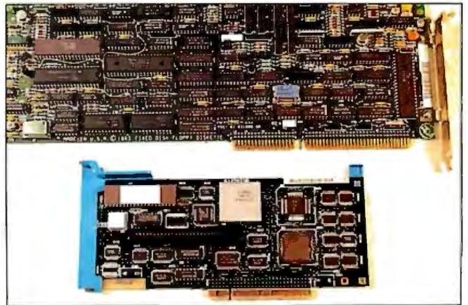
**Photo 4:** The PC AT's hard and floppy disk controller (top) versus the Model 50's hard disk controller (bottom).
