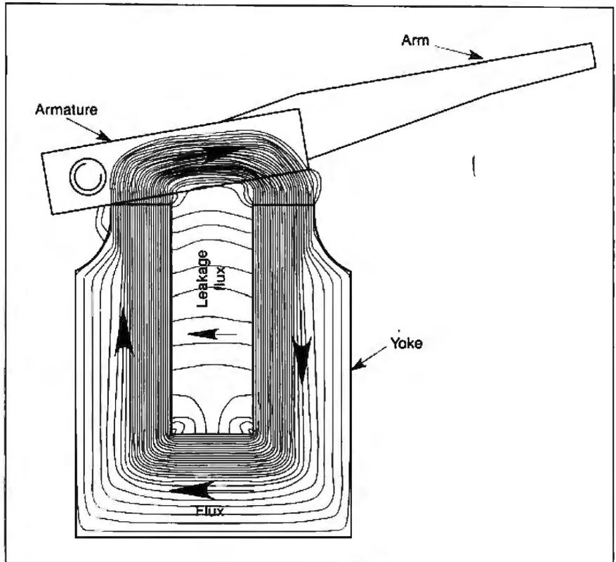
bury engineers rejected the previous coaxial design. A laminated cylinder is expensive to manufacture and is less efficient. Instead, they chose a simple U-shaped yoke with a pivoted armature (see figure 3) and used this design as the basis for a mathematical model describing the dynamics of the actuator to the point of air-gap closure (when the armature is pulled down by magnetic force onto the yoke).
