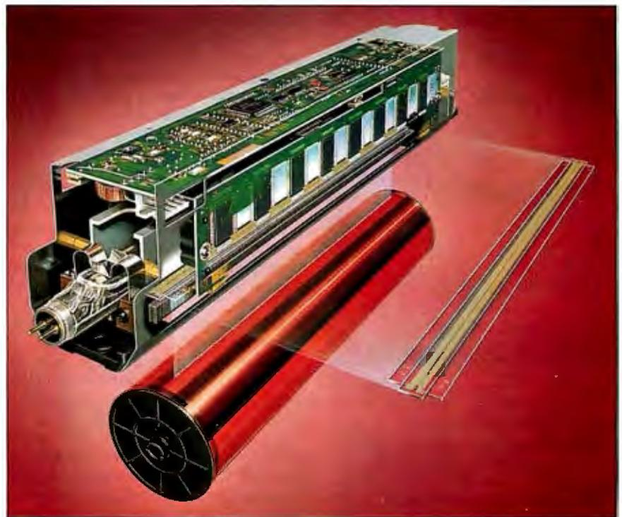
**Figure 2:** The print-head assembly of an LCS printer. The fluorescent bulb in the head provides light to the shutters, which open and close according to commands from the controller, charging selected dots on the photoreceptor drum. (Figure courtesy of Taxan USA Corp.)
