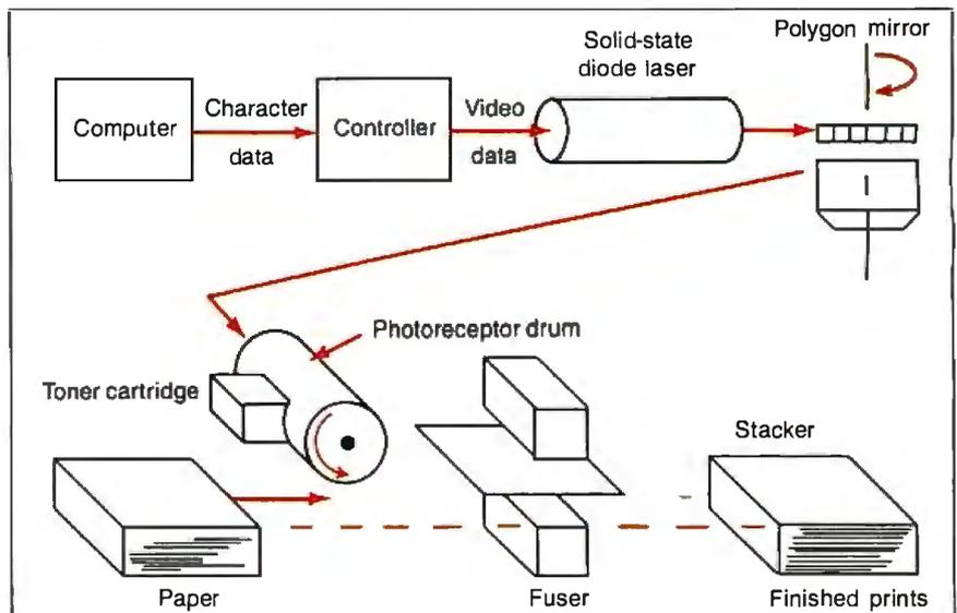
**Figure 1:** A schematic diagram of a laser printer. Raster-scanned light from a laser is deflected by a mirrored cylinder to expose the surface of a photoreceptor drum. The charged areas attract toner to the drum, which is then transferred to paper and fused on by heat.
