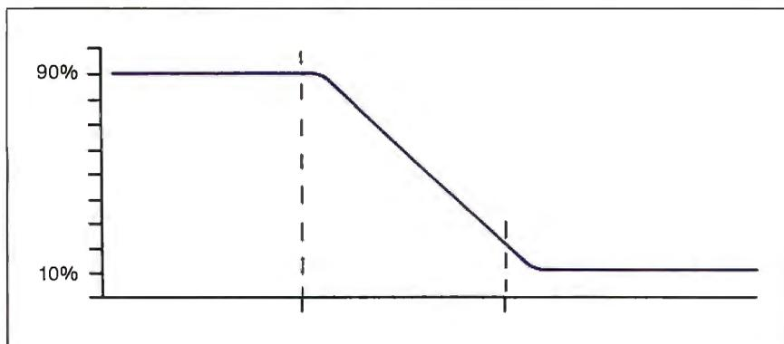
**Figure 6:** The gray level of a character is plotted as a function of distance. The area between 90 percent and 10 percent intensity corresponds to the fuzzy edge of the character. In sharp, clear printing, this region is minimized.
