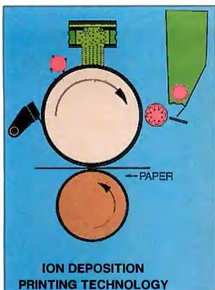
**Figure 3:** A schematic diagram of an ion-deposition printer. A modulated ion source (top) similar to that in a triode electron tube generates the ions, which are directed onto the drum, forming a latent image. The image attracts toner from the cartridge, which then is pressure-fused onto paper passing between the drum and a pressure roller. (Figure courtesy of C. Itoh Electronics Corp.)
