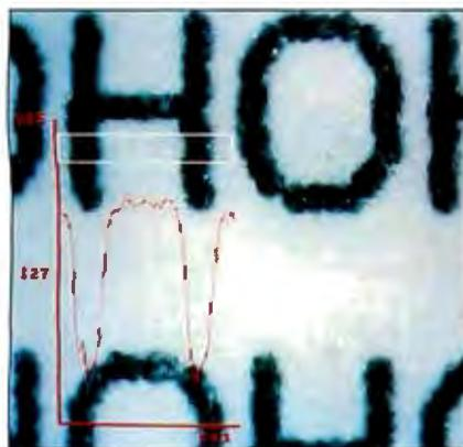
**Photo 3:** Edge sharpness is measured within the white border. The red graph shows the rate of fall off from black to white.
