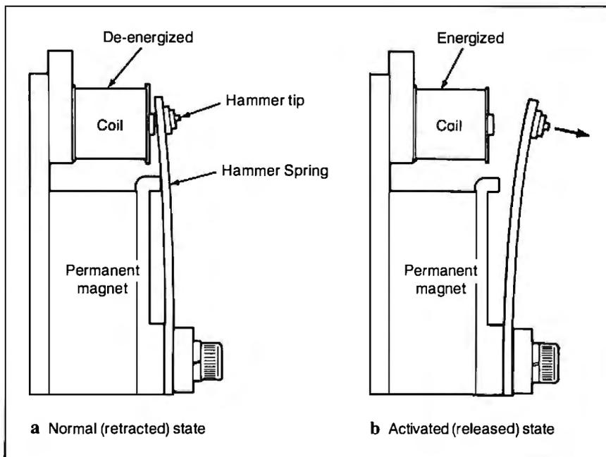
**Figure 3:** The hammer bank consists of 24 stored-energy print hammers. a) While the coil is de-energized, the permanent magnet holds the hammer in tension. b) When the coil is energized, its magnetic force field cancels that of the permanent magnet, letting the hammer spring forward, striking the ribbon onto the paper on the platen.
