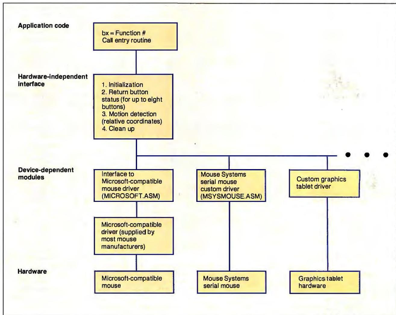
**Figure 1:** By placing a device-independent interface between the application code and the input hardware, a programmer can write an application that works with a variety of input devices. The device-dependent code is isolated into modules
