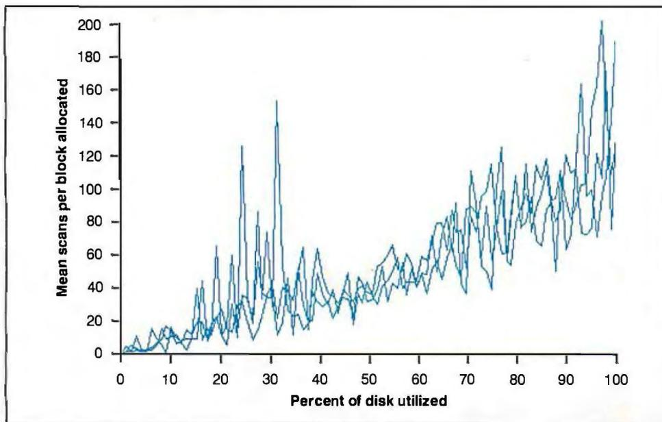
**Figure 2:** A simulation plot showing the mean number of scans required per block allocated as a function of disk utilization; three runs are plotted. The first-fit algorithm was used. Note the direct linear relationship between disk utilization and scans required. In this simulation, disk capacity is 1000 blocks, and the mean file size is 1 percent of disk capacity.
