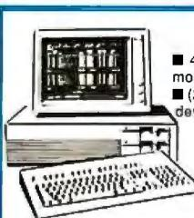
■ 4.77/10MHz. ■ 640 KB RAM (120 nano-seconds) on motherboard. ■ 150W Power Supply. ■ 8 Expansion Slots.
