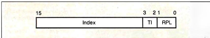
**Figure 2:** The selector format. The index can range from 0 to 8191, and it points to the descriptor. The TI equals 0 if the selector refers to the GDT, or 1 if it refers to an LDT. The privilege level (RPL here) is described in figure 3.
