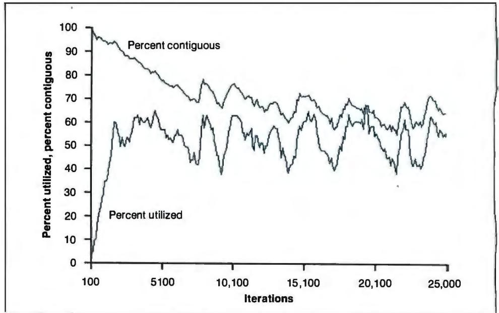
**Figure 5:** The same as figure 4, but the next-fit algorithm was used. Percent contiguous remains at a constant high level under the usage pattern selected for this simulation. With other usage patterns (not shown), percent contiguous drops to 90 percent but remains relatively constant.
