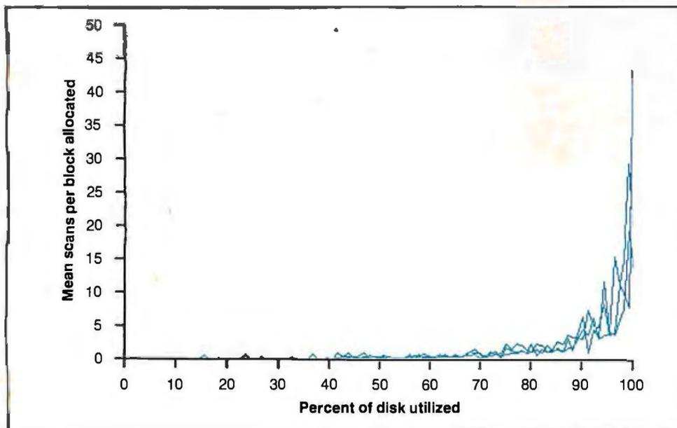
**Figure 3:** The same as figure 2, but the next-fit algorithm was used, and mean file sizes for three runs are 0.5, 1, and 2 percent of disk capacity. Note that the number of scans remains at a constant low level until the utilization reaches 90 percent.
