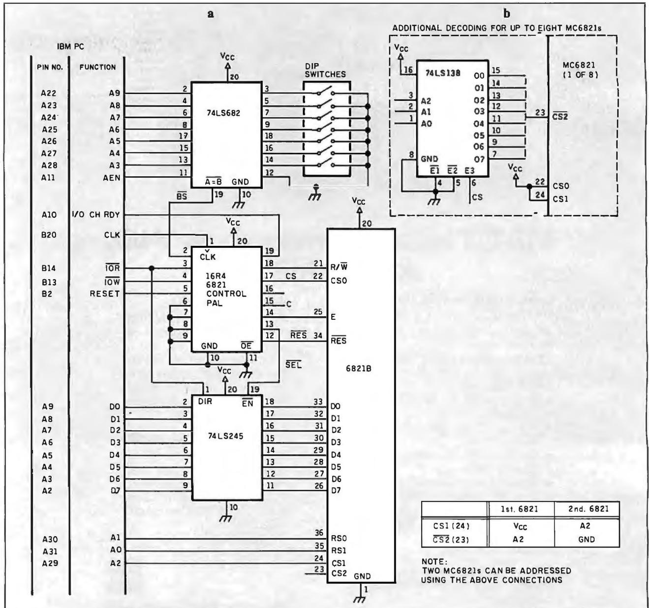
**Figure 10:** (a) A circuit design that uses the MC6821 as a word I/O port. The note tells you how to connect two MC6821 chips. (b) Use of a 74LS138 decoder to interface up to eight MC6821 chips to the circuit.
