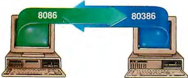
80386-based PCs & PS/2s are dual-personality computers. To run DOS programs, they act as PCs with a 640K memory limit. But to take advantage of their minicomputer capacity, they operate in true 80386 mode which lets them address up to four gigabytes of memory. PC-MOS enables the 80386-host and its workstations to independently switch between these modes—making DOS compatibility and 80386 power simultaneously possible.
