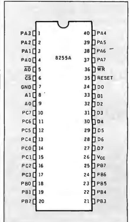
Figure 3: Pin-outs for the Intel 8255.
