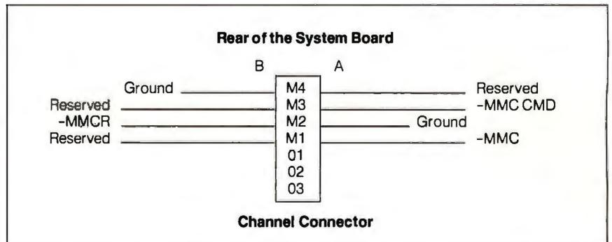
Figure 2: The matched-memory extension to the 32-bit Micro Channel.
