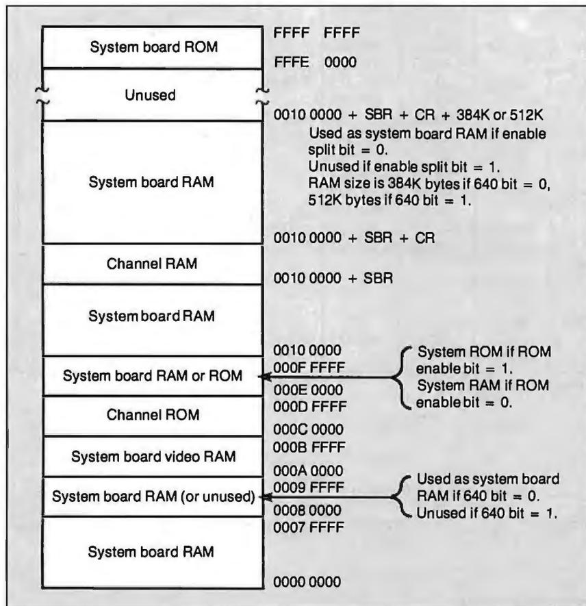
**Figure 1:** The PS/2 Model 80 memory map. The memory arrangement is determined by the contents of the memory-encoding and split-address registers. SBR is system board RAM; CR is channel RAM. System board RAM and channel RAM are allocated in 1-megabyte chunks above address FFFFFh, with the exception of the split-system RAM. The system ROM at addresses E0000 through FFFFF is a copy of the system ROM at addresses FFFE0000 through FFFFFFFF.
