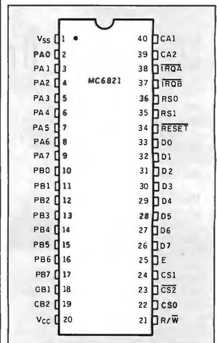
Figure 8: Pin-outs for the Motorola MC6821.
