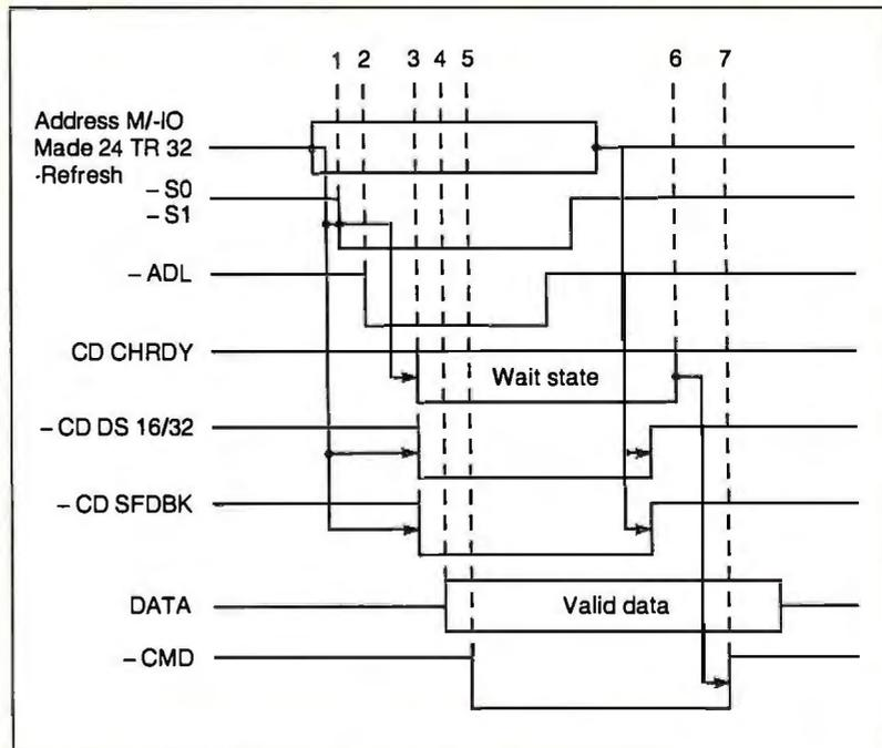
Figure A: A Micro Channel Basic Write cycle.
