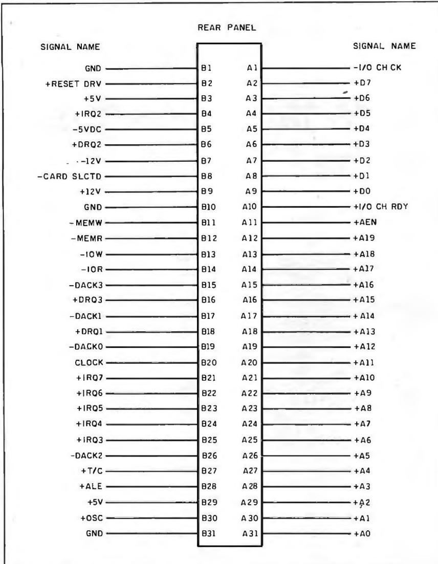
low at the end of the T2 cycle. Note that when the card tristates the driver for the I/O CH RDY line (shown in the diagram with the level at the halfway point), the line is actually pulled up to the ready state. Delaying the I/O cycle by more than a few microseconds will cause problems with the memory refresh system. The designs supplied here normally won't require more than a few extra clock cycles to operate properly.
