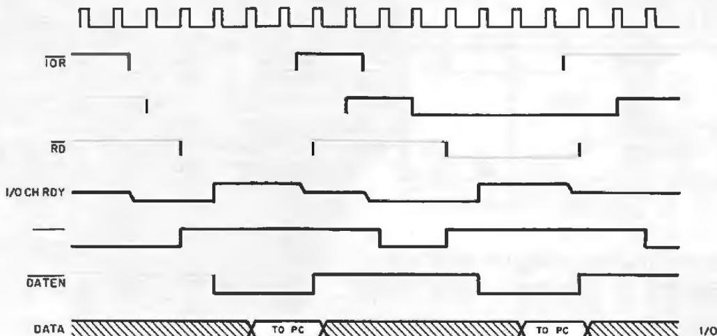
Figure 12: Timing signals for an NSC810A word I/O cycle. I/O CH RDY is used to extend the PC I/O cycles.
