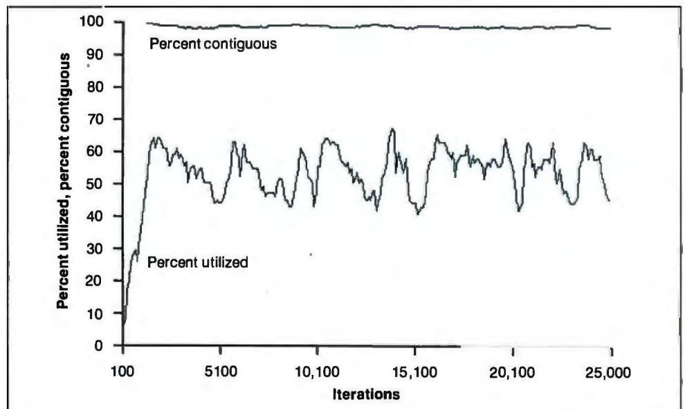
**Figure 6:** In modified next-fit simulation, resetting the last-position pointer after every 100th iteration brings the percent contiguous down to around 85 percent, in close agreement with measurements on an actual disk.
