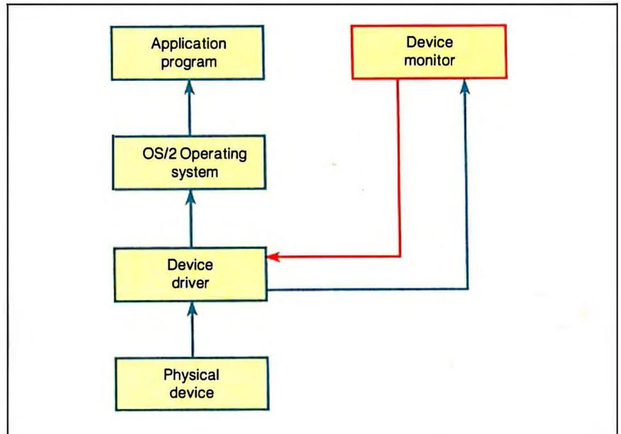
**Figure 1:** The left side of this diagram shows the normal flow of data from a character device to an application. Registering a device monitor changes the flow to add the box on the right. The characters are passed from the driver to the device monitor in packets, where they can be translated or deleted, and new characters can be added. The characters are then passed back to the driver and from there flow through the operating system to the applications.
