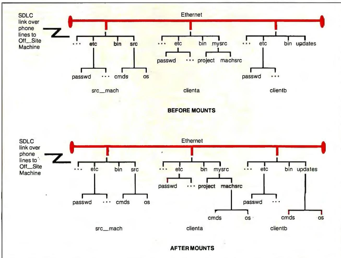
**Figure 1: A four-machine RT PC network before and after users of the network have issued commands shown in table 2. The highlighted lines in the second half of the figure indicate paths that have been changed or added due to the commands.**
