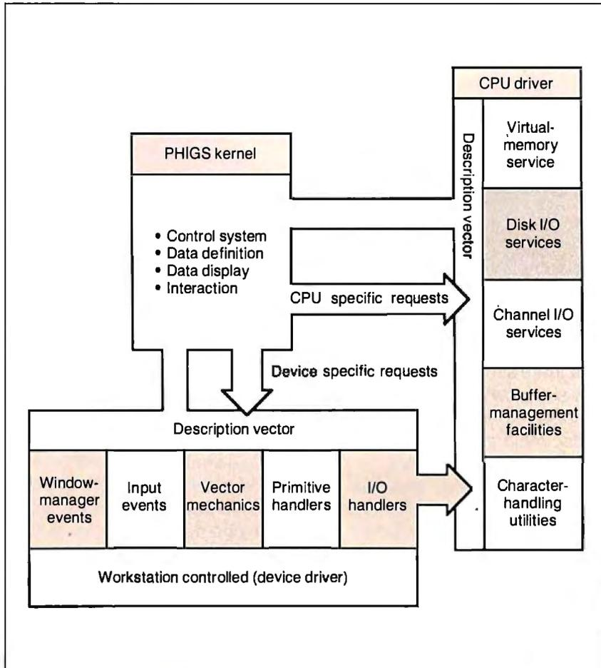
Figure 4: Figaro's CPU and device intelligence.
