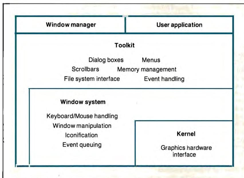
**Figure 1:** Window-system architecture. A window system provides a high-level interface between the application and the hardware.
