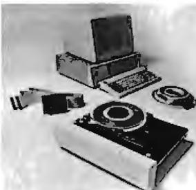
For information interchange, backup and archival storage, AK Systems offers a 9-track, IBM format-compatible 1/2" magnetic tape subsystem for the IBM PC, featuring:
