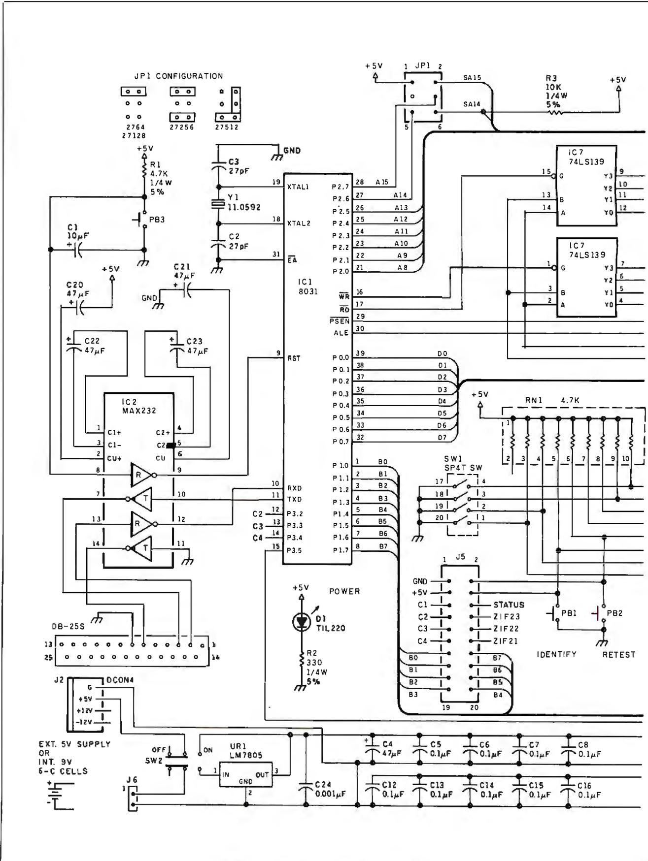
Figure 2: Schematic for the Circuit Cellar IC tester.
