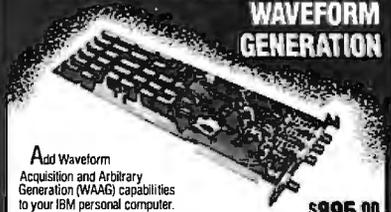
Add Waveform Acquisition and Arbitrary Generation (WAAG) capabilities to your IBM personal computer. Your PC becomes a dual-channel scope and a waveform generator when you plug in this single-slot-board. All the software you need is supplied to allow you to:
