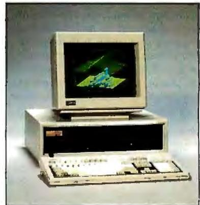
disk with less than 20-ms access time. The system comes with a 1.2-megabyte 5¼-inch floppy disk drive, and a 1.4-megabyte 3½-inch floppy disk drive is available as an option. Also available is a 135-megabyte internal tape drive that uses DC-600 tape cartridges.
