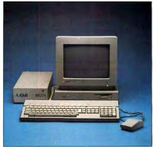
The Mega 4 uses the TOS operating system and the GEM Desktop ROM-based system software. With a color monitor, the Mega 4 costs \$2599.95. (See the box on page 154 for details on the different configurations and their prices.)
