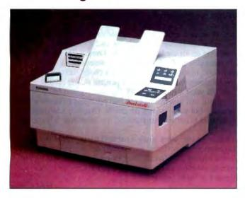
The Toshiba PageLaser12 (\$3699) is a 12-page-per-minute laser printer that features 300 by 300 dot-per-inch resolution, serial and parallel connections, 512K bytes of memory (expandable to 2 megabytes), and emulations for the Diablo 630, IBM 5152 Graphics, Qume Sprint 11, and Toshiba P351 printers.
