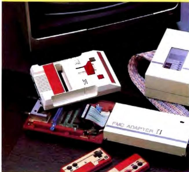
This is the key to debug the custom CPU FMC-2A03 of the FAMILY COMPUTER (Nintendo). All you need is this unit! Then, you can debug and develop your software for the FAMICOM without much knowledge on hardware of the FAMICOM.
