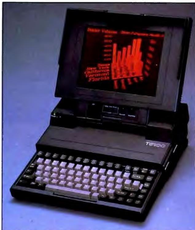
Toshiba's new portable is 80386-powered.
