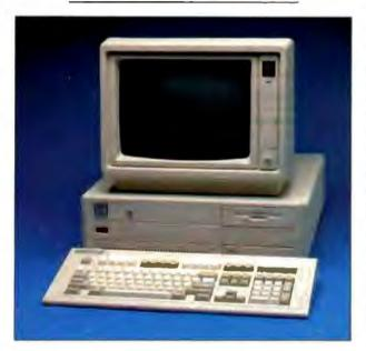
narrower and 11/2 inches deeper than the standard IBM PC AT. It looks and feels sturdy. It has a power-on LED on the front panel, but it has no disk activity light. This minor omission can be annoying when you are trying to decide whether the system is working or hung. There is a keyboard lock on the front and a rocker-style power switch on the rear right side.
