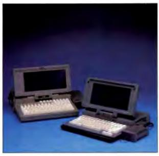
The Datavue Snap l+1 (left) and Spark are 9-pound laptops with full-size keyboards and a choice of displays.
