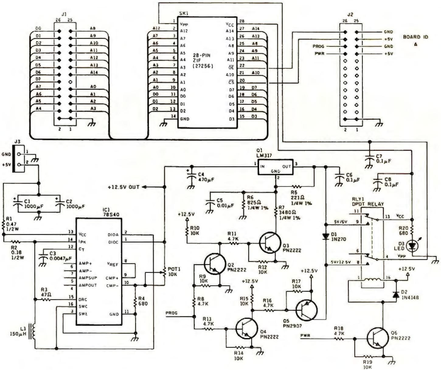
Figure 1: Schematic for the BCC180's EPROM programming board.
