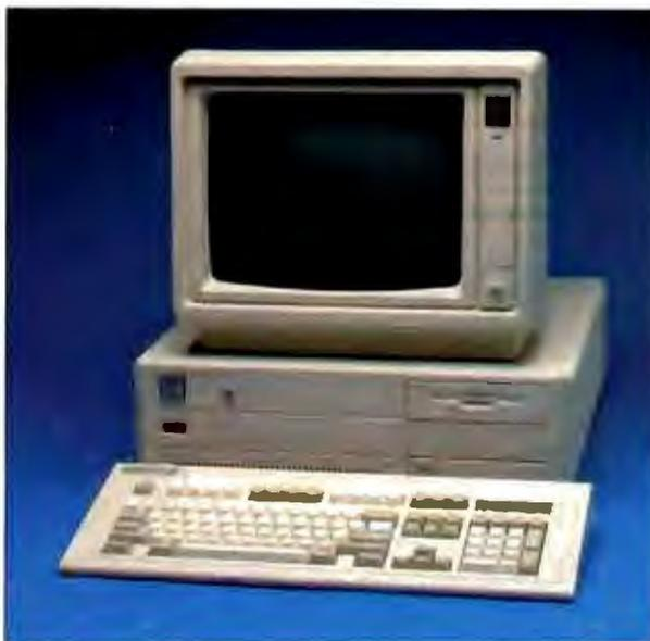
narrower and 1½ inches deeper than the standard IBM PC AT. It looks and feels sturdy. It has a power-on LED on the front panel, but it has no disk activity light. This minor omission can be annoying when you are trying to decide whether the system is working or hung. There is a keyboard lock on the front and a rocker-style power switch on the rear right side.
