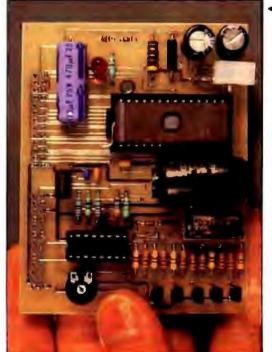
◆Photo 2: The EPROM programmer daughterboard for the BCC180. An EPROM is shown inserted in the zero-insertion-force socket (upper right of board).
