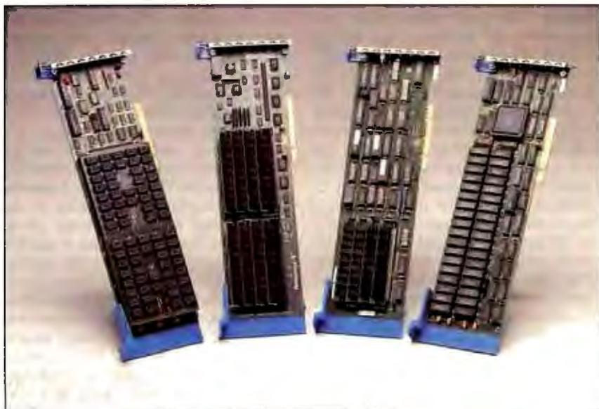
*(Left to right) The Cumulus CuRAM, AST Advantage/2, Quadram QuadMeg PS/Q, and Everex Ram II 4000. Each of these offers more than 2 megabytes of add-in RAM for the Micro Channel bus.*
