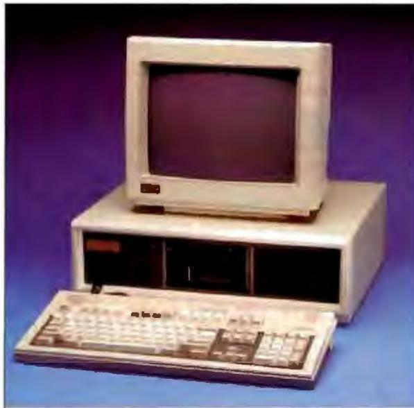
Compaq has always had a reputation for making high-quality, high-performance systems, but the company has surpassed all past efforts with the Compaq Deskpro 386/20. It is an AT-compatible system that uses a 20-MHz Intel 80386 CPU and Compaq's new Flex architecture—a combination of concurrent buses with 32K bytes of cache memory—to provide the highest level of PC performance yet. I love this machine.
