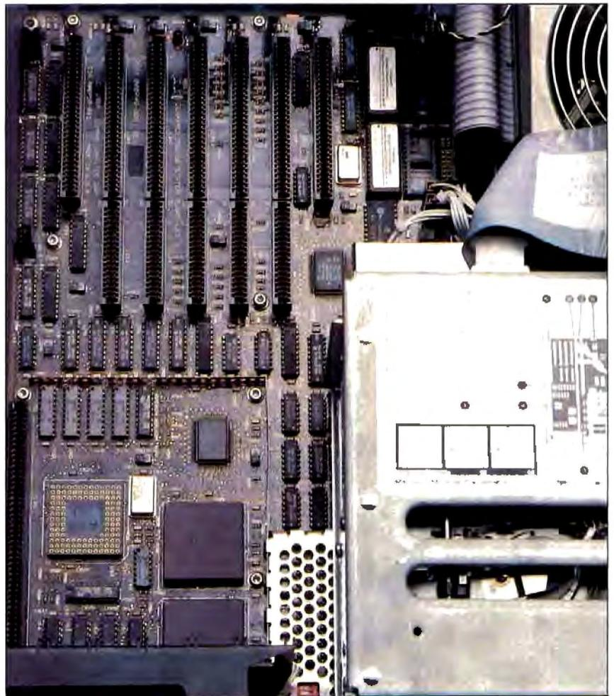
**Photo 1:** *Compaq Deskpro 386/20 motherboard. The system memory board connector is at the bottom left. The board features extensive radio-frequency-interference shielding. The perforated metal cover, at the bottom right beneath the floppy disk drive, covers the 32K-byte bus cache memory.*
