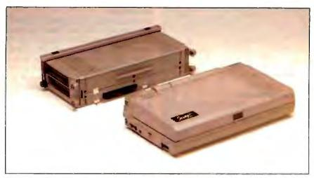
**Photo 1:** The Snap l+l separates into the rear Expansion Module (left), containing disk drives, 640K bytes of main memory, and a half-card expansion stot; and the front Lap Module (right), which, with an optional RAM expansion card, can be used as a lightweight, RAM disk-based portable machine.
