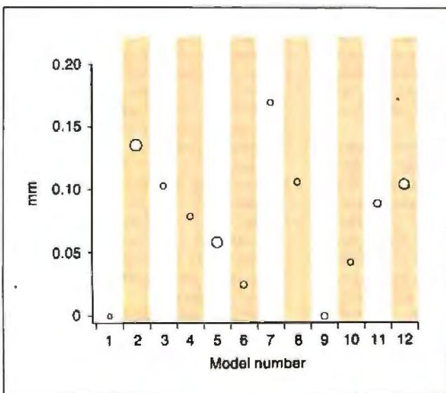
▲ **Figure 4:** Misconvergence in mm. Linear measurements have been adjusted to account for each monitor's screen size. Low error (close to zero line) is preferable. ▲ = red-to-green error, ● = blue-to-green error, ■ = red-to-blue error.
