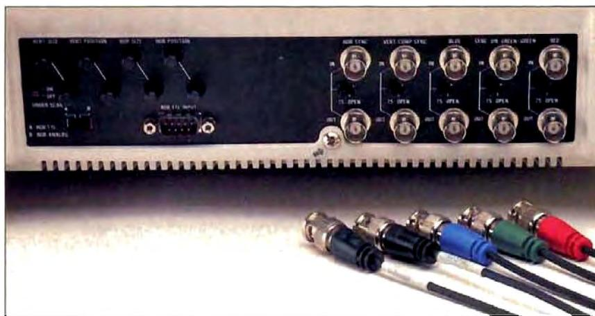
**Photo 2:** The rear panel of the Electrohome ECM 1312 includes most of the connector types and adjustments mentioned in the product descriptions.
