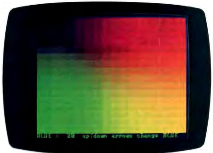
top to bottom. The amount of blue is adjusted from maximum to 0 by keyboard control. The test let us check the monitor's ability to represent fine shades of color across the spectrum (see photo 1).
