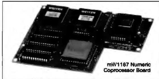
mW1167 Numeric Coprocessor Board
