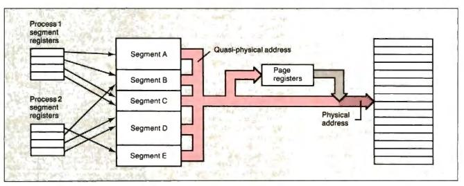
Figure 3: A hybrid segmentation/paging system tends to reduce both internal and external fragmentation.
