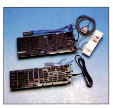
Hardware-assisted debuggers like AT Probe (top) and Periscope III (bottom) can significantly reduce debugging time—for a price.
