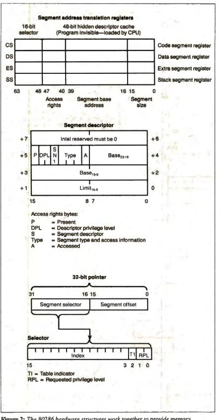
Figure 2: The 80286 hardware structures work together to provide memory protection. The action of loading a segment selector into a segment register causes the 80286 to use the selector to index into the LDT and use the corresponding segment descriptor for limit and access checking.
