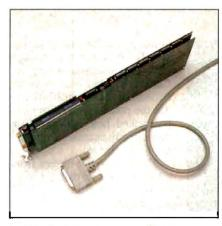
Photo 1: The PS2.0 printer/scanner controller board. It is composed of two boards connected together to occupy one slot.
