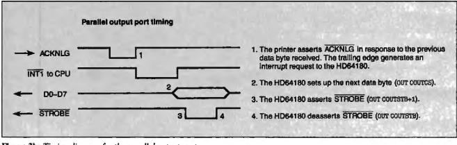
Figure 3b: Timing diagram for the parallel output port.
