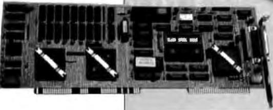
Amiga side, things are a bit more complex because the Amiga needs to provide keyboard and display facilities for the Bridgeboard. The Amiga's existing multitasking windowing software handles all this, letting the PC run as a window within the Amiga.
