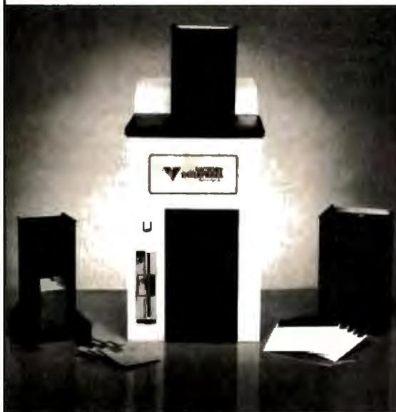
**Copy Different Formats, Flawlessly.** Our Auto-Format-Analysis™ feature lets you copy different formats, including PS/2\*. The system tests for quality and accuracy, sorting disks into one of two output cannisters.
