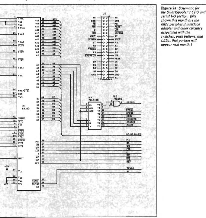
generator consisting of a flip-flop and a couple of gates (IC5, IC6, and IC19). The plastic-leaded-chip-carrier version of the HD64180 can address 1 megabyte, but I feel that 256K bytes is more than adequate for typical printing applications, and it keeps power consumption low.
