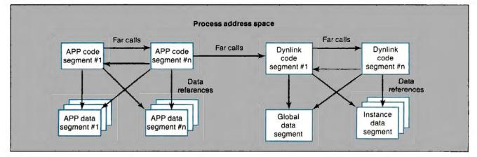
Figure 3: A dynlink routine used as a subsystem. The main difference between a dynlink subsystem and a subroutine is the presence of the global data segment(s).
