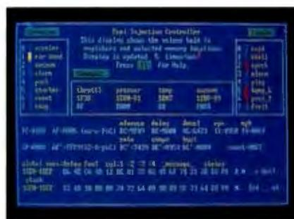
■ InSight is made possible by the 8620's advanced bus state analyzer, its 2730-bus-cycle trace buffer, and a new high-speed parallel interface that eliminates RS-232 bottlenecks.
