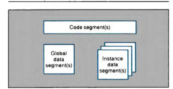
Figure 2: A dynlink routine can have three kinds of segments. Each process using the dynlink module will get its own copy of the instance data segments while sharing the same copy of the global data segments with the other processes attached to the dynlink module. OS/2 performs an optimization so that code segments are shared transparently among all processes.
