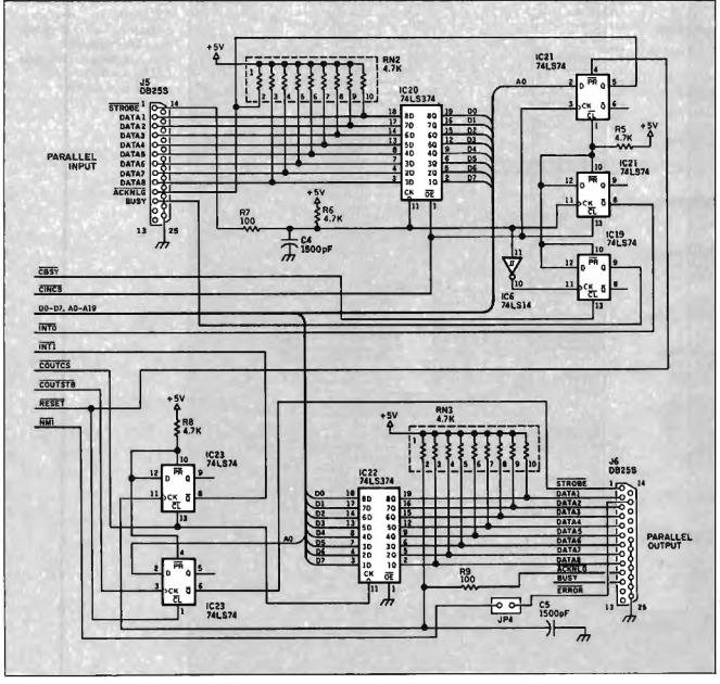
Figure 2b: The SmartSpooler's parallel I/O section.
