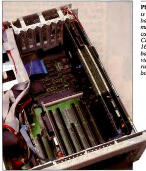
Photo 1: The WYSEpc 386 is designed around a backplane rather than a motherboard. All system cards, including the 80386 CPU card, insert into 8- and 16-bit expansion slots in the backplane and communicate via 32-bit connectors that run across the top of the boards. IOtech has the widest selection of *easy-to-use* interfaces & software for IEEE 488 (GPIB/HPIB)
