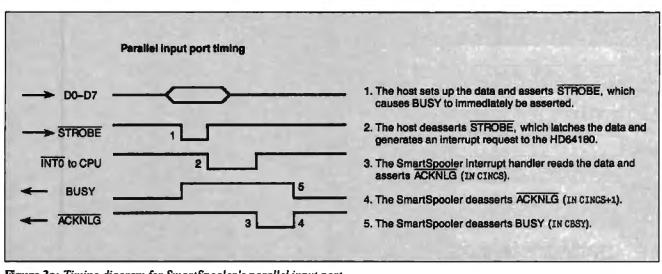
Figure 3a: Timing diagram for SmartSpooler's parallel input port.
