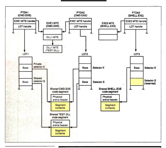
Figure 3: The difference between private and shared selectors. Private selector E maps the same shared (code) segment for all invocations of an executable file. Other tasks may use selector E for other purposes. Shared selector S maps the same shared (code) segment for all tasks attached to the TEST.DLL dynalink library. Shared selector S is reserved for the TEST.DLL segment; other tasks cannot use selector S for any other purpose.
