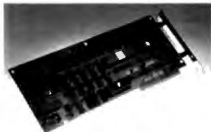
Other RLL controllers require drives approved for RLL encoding. The PERSTOR 200 Series Advanced RLL Controllers are compatible with standard MFM drives and RLL approved drives, whether oxide or plated media.
