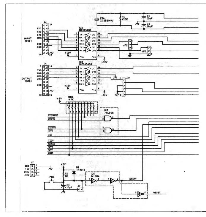
HD64180 CPU because it is ideally suited to the task and significantly reduces the hardware complexity. First, it includes two RS-232C serial ports on-chip, eliminating an external dual-UART (universal asynchronous receiver/transmitter) chip.
