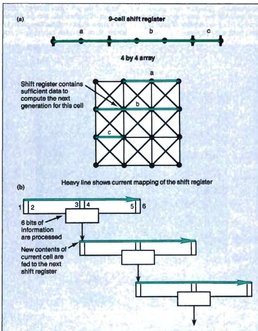
**Figure 3:** The Princeton machine's pipelined architecture. (a) The two-dimensional array of cells is mapped onto a shift register. The illustration shows the case for a 4 by 4 array and a 9-cell shift register. At any given time step, the register has enough information to compute one cell's next generation. It takes 16 time steps to do the entire 4 by 4 array. (b) By pipelining multiple shift registers, multiple generations can be computed at once.
