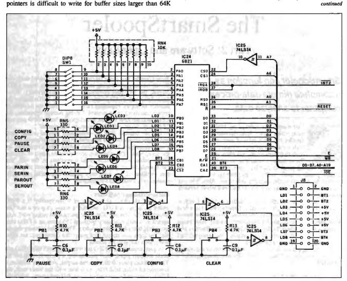
Figure 1: Schematic for SmartSpooler's DIP-switch and LED 1/O circuitry. A single 6821 peripheral-interface-adapter chip handles all the switches and lights.
