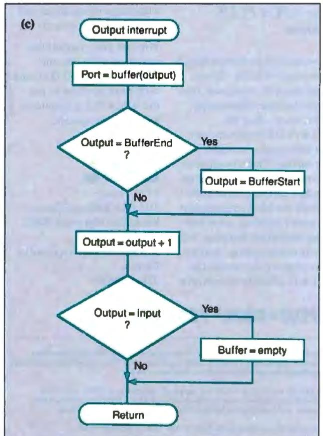
The solution to the problem of inefficiency is to exploit the HD64180's excellent interrupt capabilities. SmartSpooler's I/O is totally interrupt-driven, including the serial and parallel ports as well as the front-panel switches. Table 1 lists these interrupt assignments.
