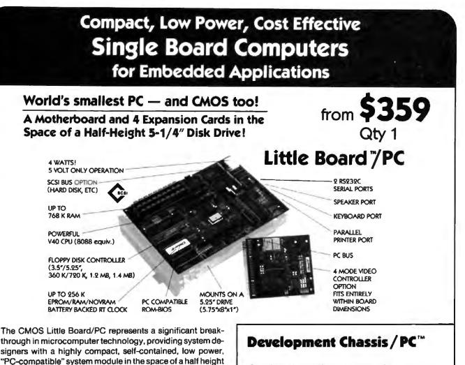
5-1/4-inch disk drive. Everything but the keyboard, monitor, disk drive, and power supply is included! The CMOS Little Board/PC is ideally suited for embedded microcomputer applications where IBM PC software and bus compatibility are required and where low power consumption, small size, and high reliability are critical. Its low power requirements, compactness, and solid state disk drive support make the Little Board/PC especially useful in rugged or
