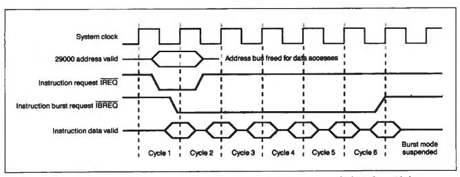
Figure 4: The timing of a short burst-mode instruction-fetch access. Notice that the instruction fetch overlaps with the beginning of each cycle except the first.
