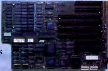
Now there's a simple solution. It's the AST Xformer/286<sup>™</sup> (pronounced "Transformer"), the ultra-fast, 10 MHz, 80286 system board that actually replaces the system board on your XT.
