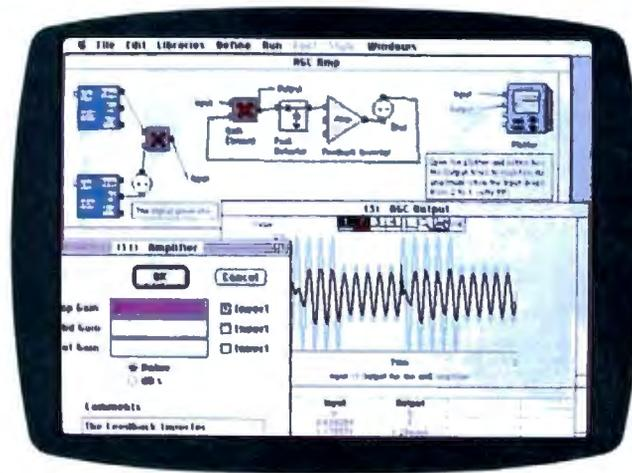
Forming a model from Extend's block diagram.
