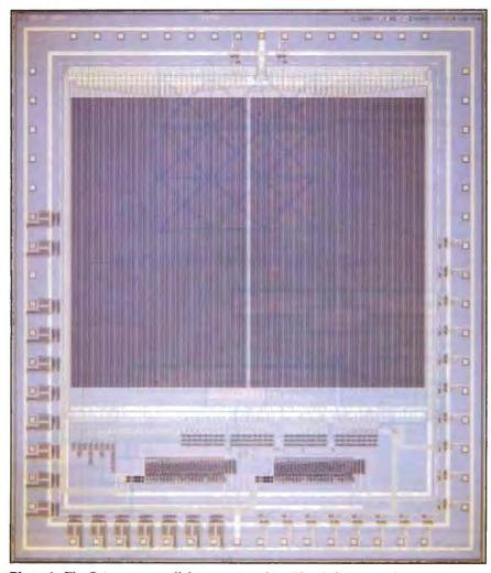
**Photo 1:** The Princeton parallel-processing chip. The shift register dominates the top three-quarters of the photograph while the two processors are at the bottom. The shift register contains 512 memory words. The entire chip contains the equivalent of 68,000 transistors implemented in 3-micron technology.
