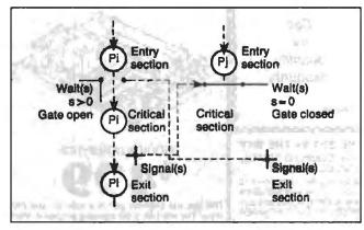
Figure 5: Using a semaphore (s) for controlling critical sections of code. Here, as Pi passes through its entry section, it "closes the gate" for Pj. When Pi exits its critical section, the signal(s) operation will reopen the gate for Pj.
