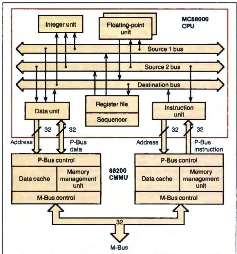
Figure A: The Motorola MC88000 RISC processor and support chip block diagram.
