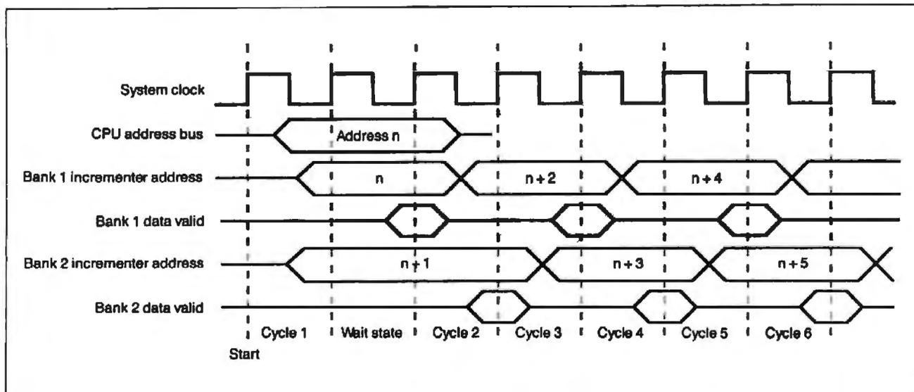
**Figure 5:** The timing for an interleaved instruction-burst access. Notice that the access switches back and forth between the two data banks. This process avoids the wait between accesses on a single bank.
