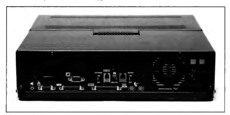
**Photo 1:** The Dynamac's back panel holds (from left to right) the audio port, the mouse port, the external floppy disk drive port, the video port, the SCSI port, the external keyboard connector, the telephone port connector, and two serial ports using DIN-8 connectors.
