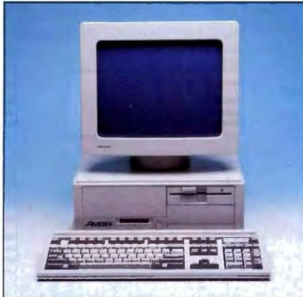
The Amdek System/386's small size and pleasing looks belie its serious side as an 80386-based microcomputer whose performance ranks among the best of the 16-MHz 80386 machines. Its CPU runs with zero wait states at 16 MHz (or with one wait state at 8 MHz) and is mounted on a card that plugs into the computer's backplane; there is no motherboard in the traditional sense of the word.
