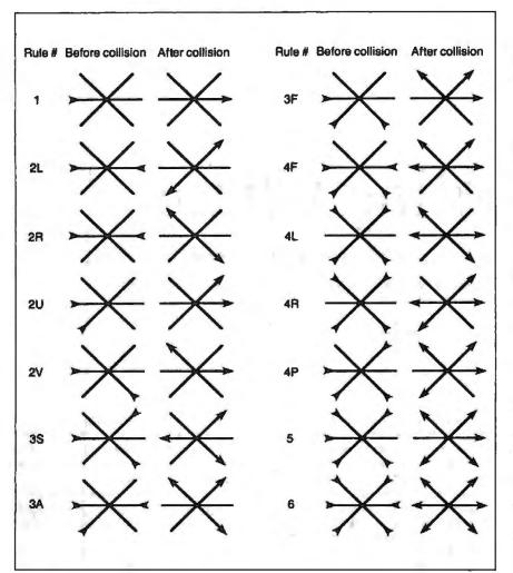
Figure 1: These 14 rules determine the effects of particles colliding in the fluidflow cellular automaton. By rotating and reflecting the axes, the rules cover all 64 possibilities.
