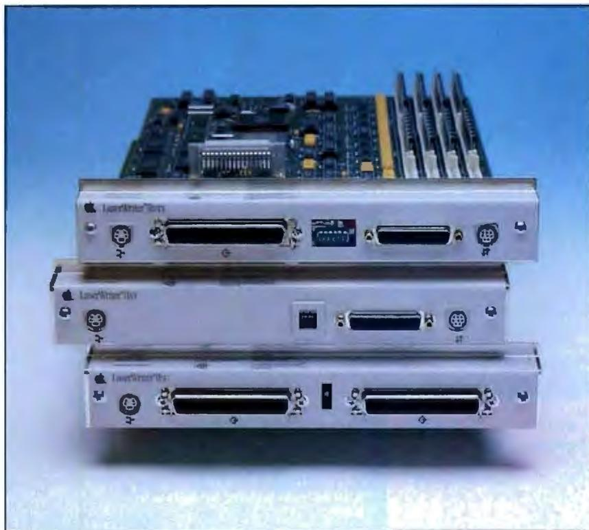
**Photo 3:** The LaserWriter II boards offer a full range of connectors. The IINTX board (top, left to right): ADB port, SCSI port, configuration DIP switches, serial port, LocalTalk port. The IINT board (middle, left to right): ADB port, configuration switches, serial port, LocalTalk port. The IISC board (bottom, left to right): ADB port, SCSI port, board SCSI address selector, SCSI port.
