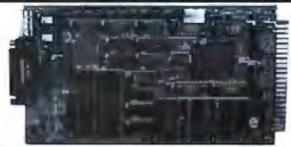
The BCC180 only 4.1" x 8.1" uses the same 64180 CMOS Z-80 instruction compatible processor as Micromint's SB180 and SB180FX single board computers. Configured primarily for process control software it features 4 parallel I/O ports, Unidirectional serial port, 125-4000bps selectable auxiliary serial port, and an interrupt driven DOM resident multitasking BASIC to control the BCC180 (uses the same 64 pin I/O expansion bus as Micromint's BCC52 controller board).
