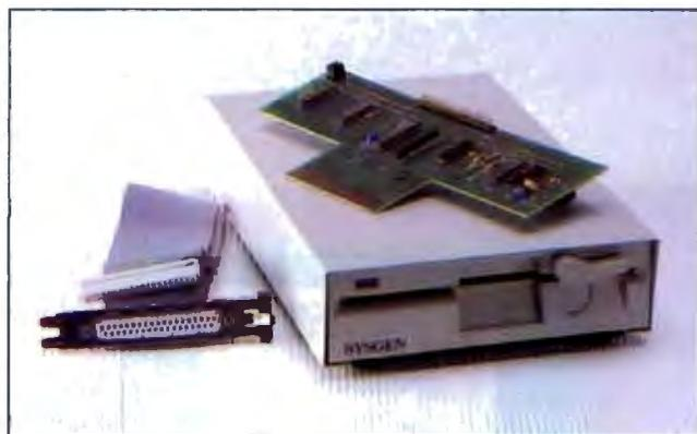
**S**ysgen's **Bridge-File** comes in two configurations. The first can add 1.2-megabyte/360K-byte 5 1/4-inch capability to IBM PS/2 Models 30, 50, and 60. A second version gives the IBM PC, XT, and AT the ability to read, write, and format both 720K-byte and 1.44-megabyte 3 1/2-inch disks. A PS/2 Model 80 version is now said to be available, but it was not part of the package I reviewed.
