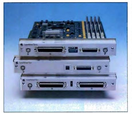
Photo 3: The LaserWriter II boards offer a full range of connectors. The IINTX board (top, left to right): ADB port, SCSI port, configuration DIP switches, serial port, LocalTalk port. The IINT board (middle, left to right): ADB port, configuration switches, serial port, LocalTalk port. The IISC board (bottom, left to right): ADB port, SCSI port, board SCSI address selector, SCSI port.
