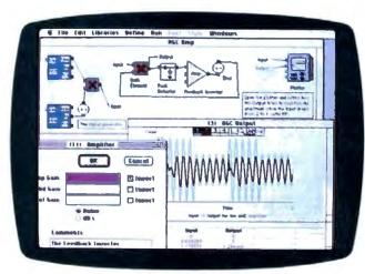
Forming a model from Extend's block diagram.
