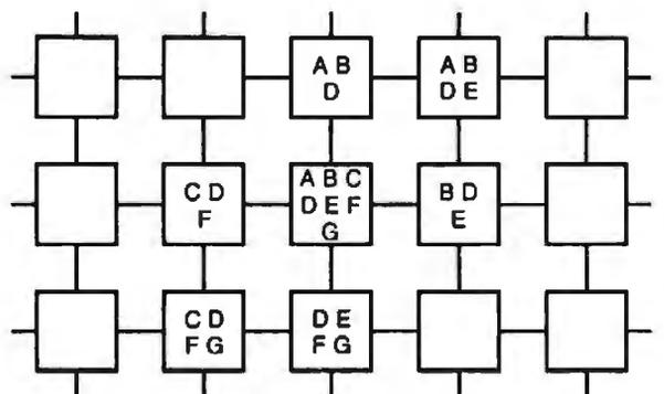
**Figure 4:** A section of the square grid of the Connection Machine, illustrating how information about a cell's six neighbors (A, B, C, E, F, and G; D is the center cell) is funneled through four pathways per cell using a four-step process. At each stage, the letter inside the cell indicates how much is "known" to that cell.
