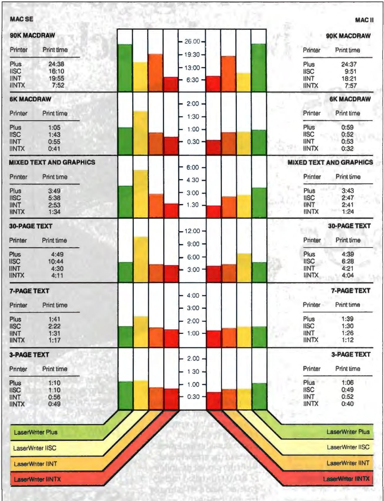
**Figure 1:** These tests compare an original LaserWriter against the LaserWriter IISC, IINT, and IINTX. The IINTX was fastest overall; the IISC was quicker than the IINT on complicated graphics or on very short text files.
