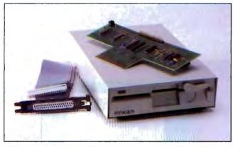
Sysgen's Bridge-File comes in two configurations. The first can add 1.2-megabyte/360K-byte 5¼-inch capability to IBM PS/2 Models 30, 50, and 60. A second version gives the IBM PC, XT, and AT the ability to read, write, and format both 720K-byte and 1.44-megabyte 3½-inch disks. A PS/2 Model 80 version is now said to be available, but it was not part of the package I reviewed.
