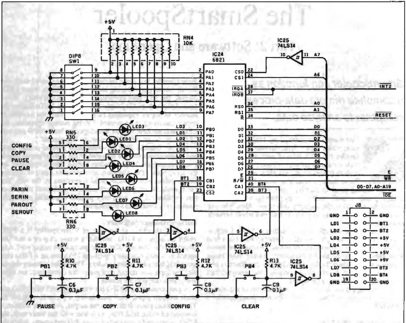
Figure 1: Schematic for SmartSpooler's DIP-switch and LED I/O circuitry. A single 6821 peripheral-interface-adaptor chip handles all the switches and lights.
